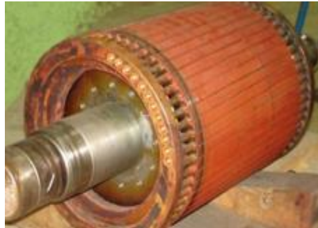
Figure I . 5: Rotor à double cage [6]
