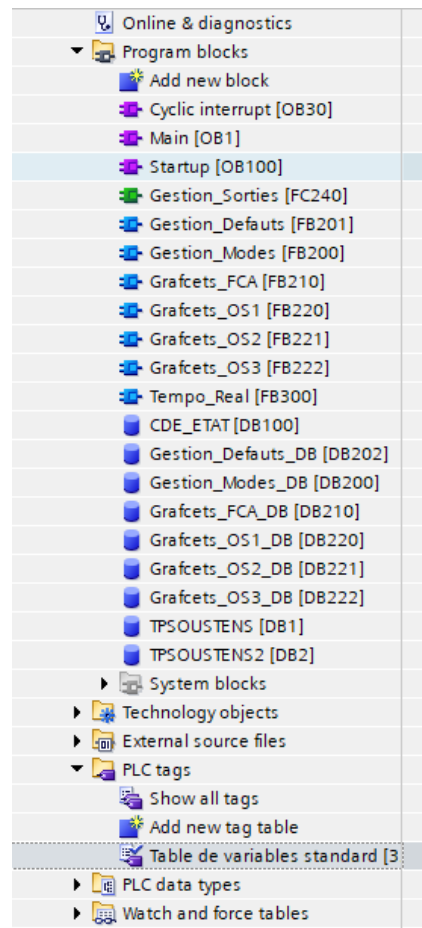
Figure III.4 Blocs du programme
