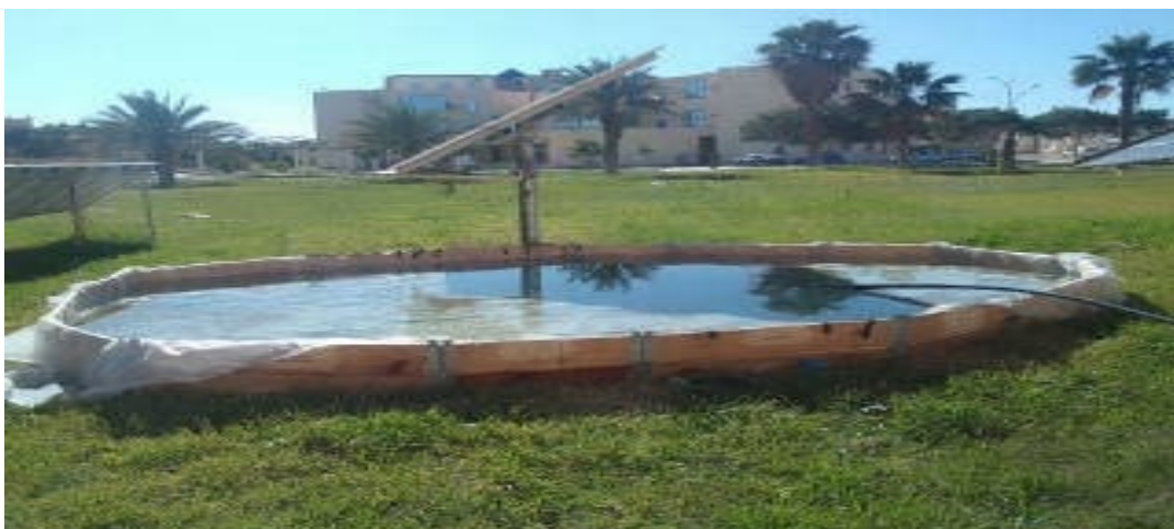
Figure. (IV.1) Experimental artificial water basin was constructed to simulate real-world conditions for floating solar systems
