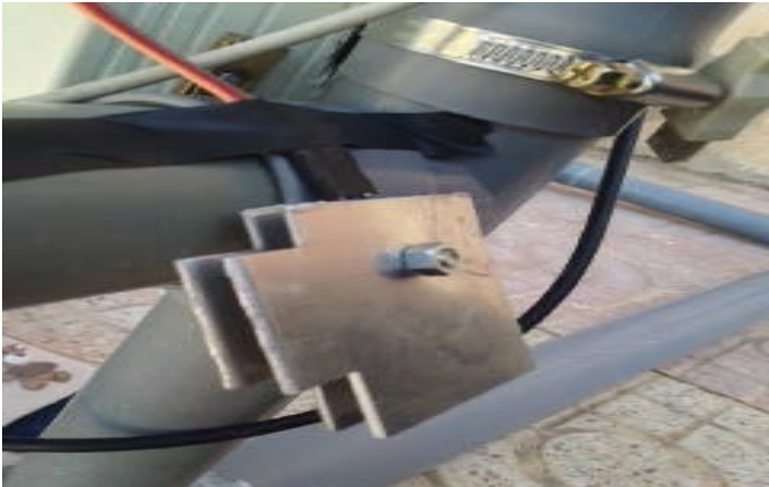
Figure (IV.12): LM35 Sensor Integrated within Aluminum Plates for Thermal Data
