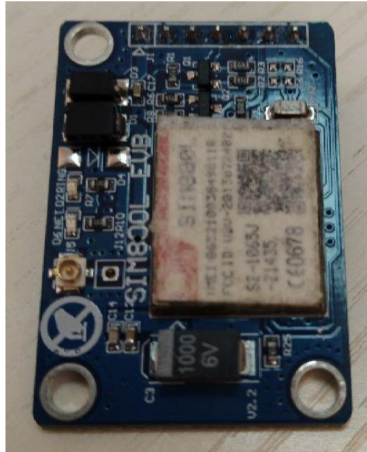
Figure III.15: The stable SIM800L module with the correct capacitor.
