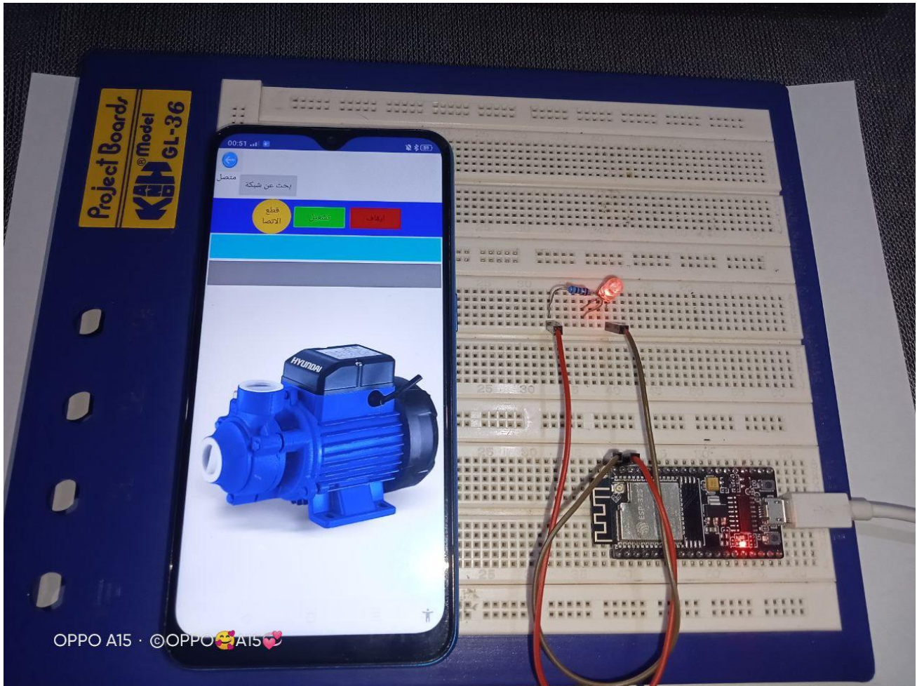
Figure III.7: Direct system control test via Bluetooth (ON and OFF states).
