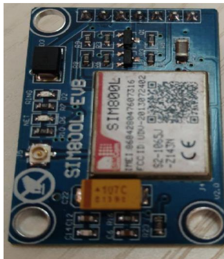
Figure III.14: The initial module with the insufficient capacitor.
