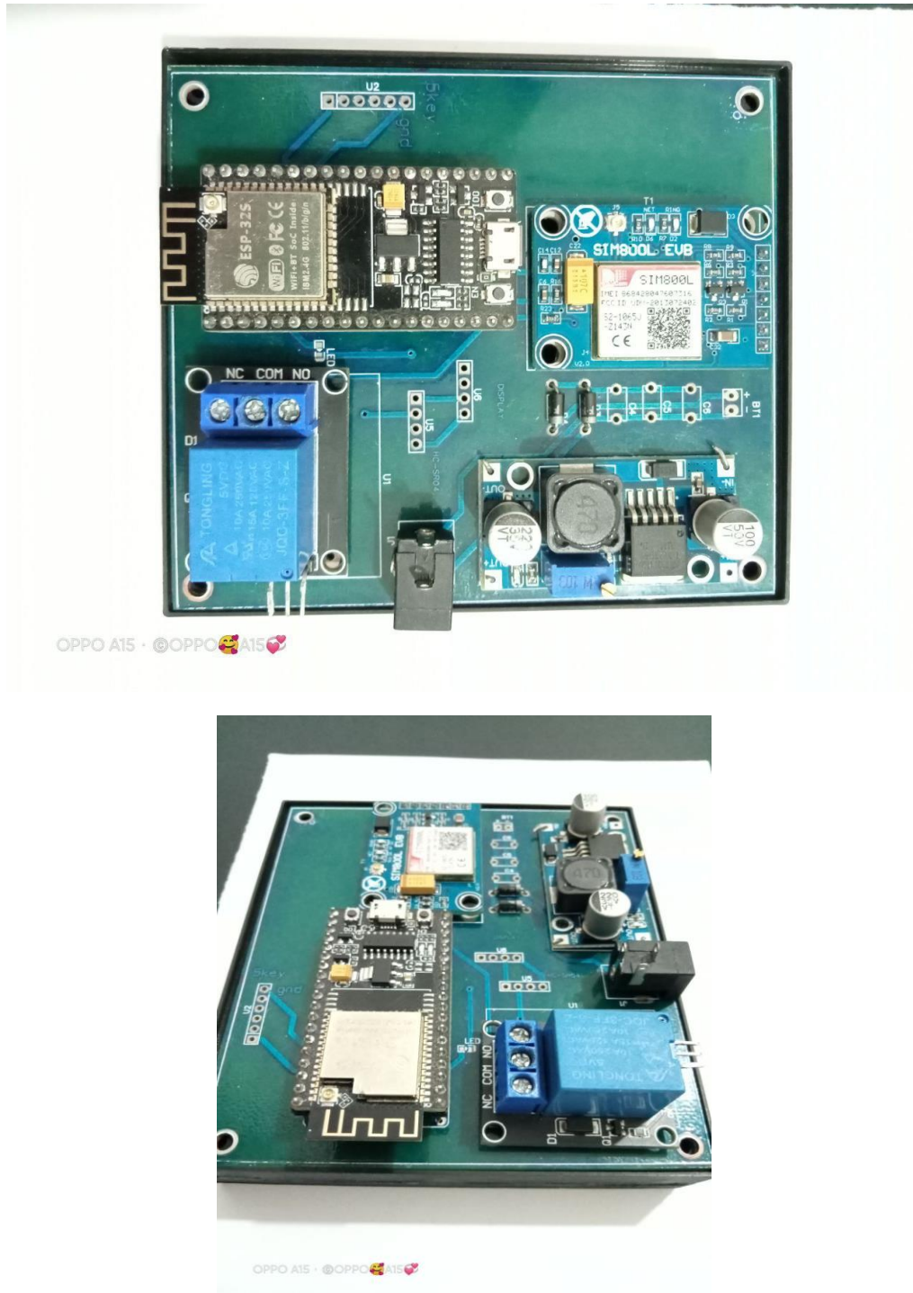
Figure III.16: The soldering of all electronic components.
