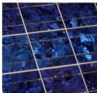
Fig I.6: Cellules photovoltaïques poly cristallin
