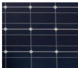
FigI.5: Cellules photovoltaïques monocristallines
