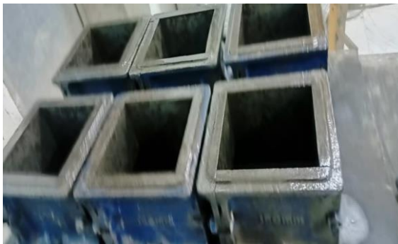
Figure II.19: Moule cubique (150x150x150 mm).
