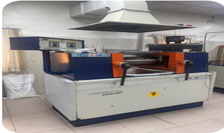
Figure 3.11. Calandre de type schwabenthanpolymix 200P.
