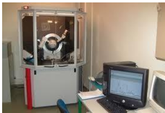
Figure III.14: Diffractometer à rayon X (CRAPC)
