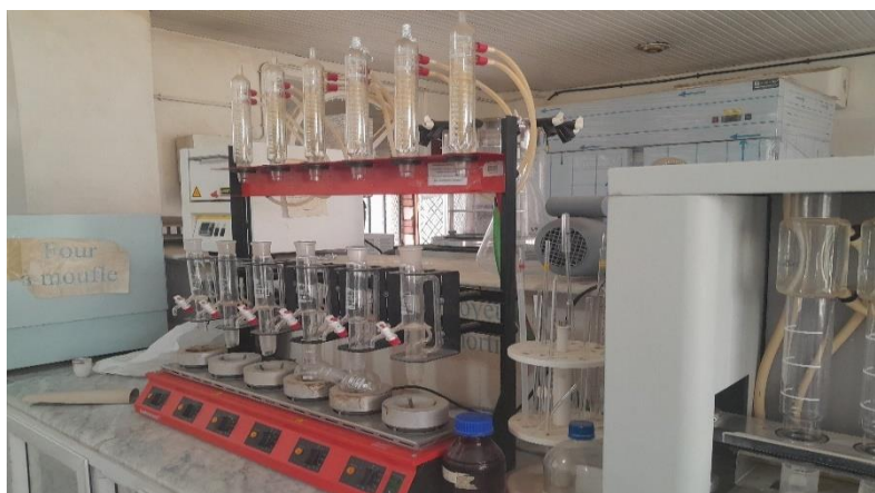
Figure III.4 : Appareil de Soxhlet multiples.
