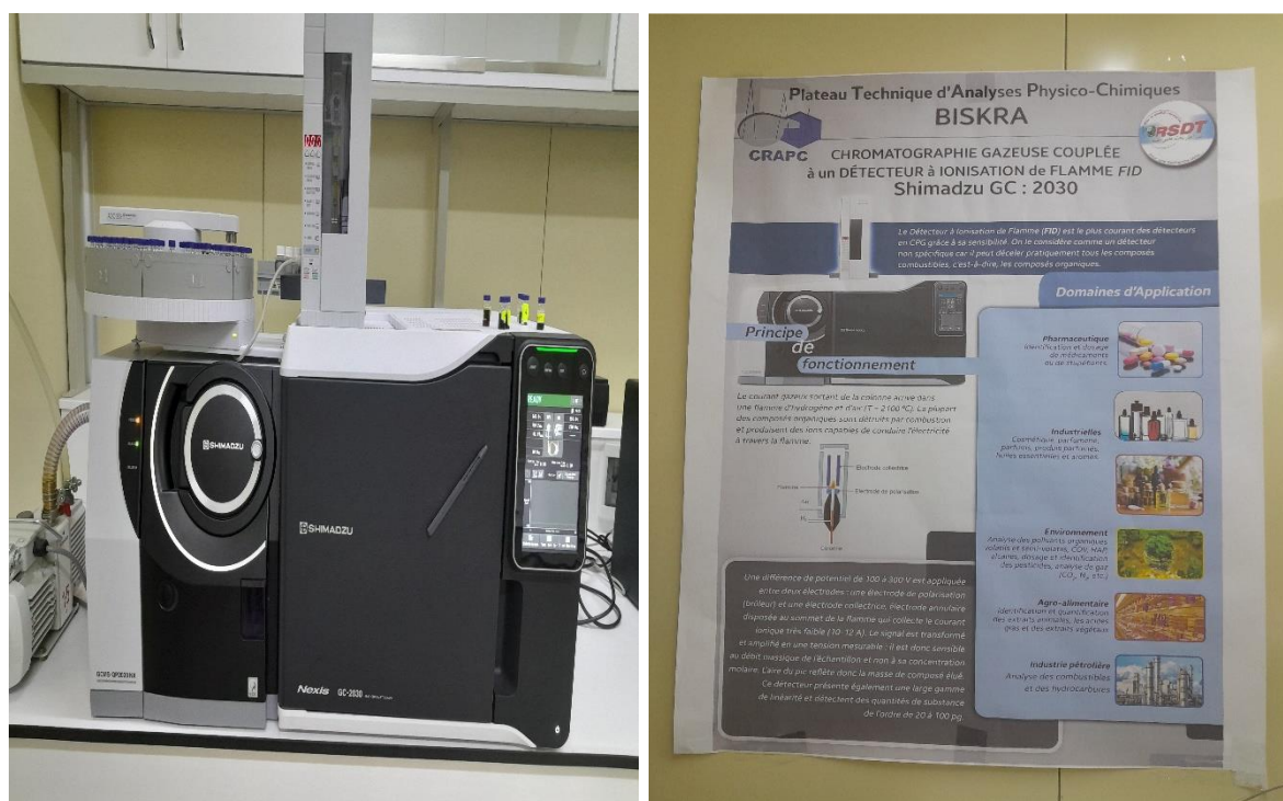
Figure III.7 : Chromatographie GC-MSS HIMADZU Nexis GC-2030.
