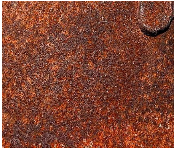
Figure (I.1): La Corrosion Uniform.
