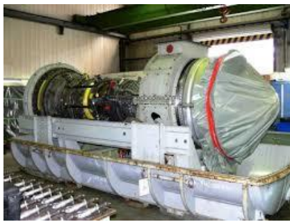
Figure III. 4:Turbine type LM5000
