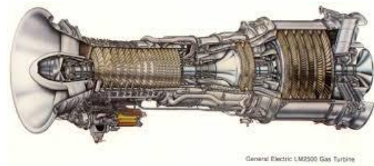
Figure III. 3:Turbine type LM2500
