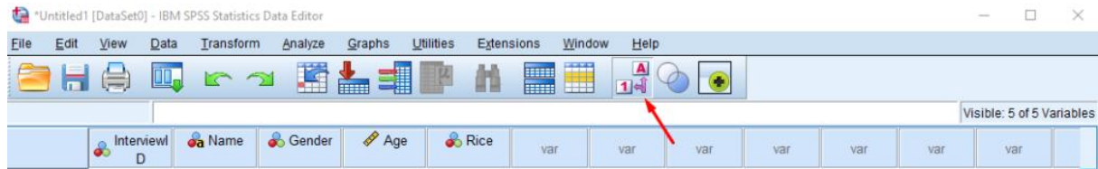
Figure 15: Activating the value labels button to show text labels instead of numeric codes in SPSS.
