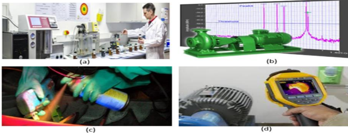
Figure 2-9 (a) Oil Analysis, (b) Vibration Analysis, (c) Ultrasonic Testing and (d) Thermography
