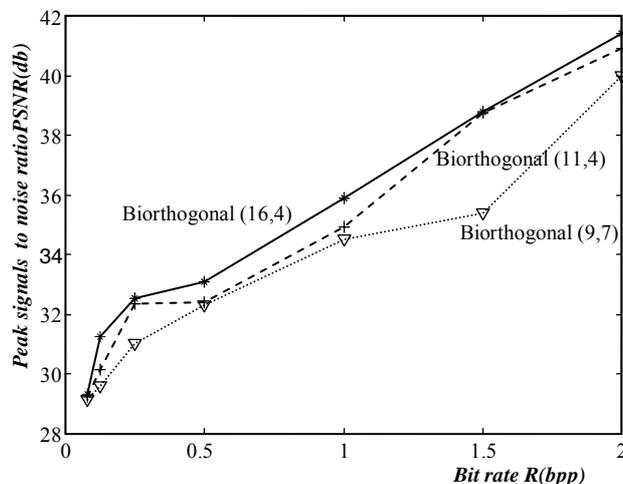
Figure 6: Quality of compression varying Biorthogonal filters((16,4),(11,4),(9,7))
