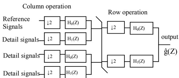
Figure 4 : Synthesis of 2D DWT
