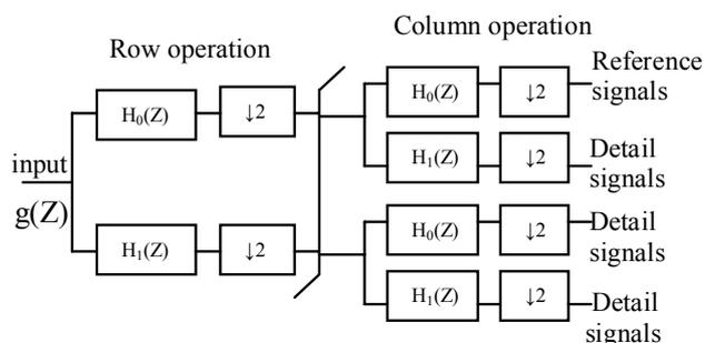
Figure 3 : Analysis of 2D DWT
