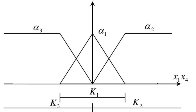
Fig. 2, Membership functions and local controllers
