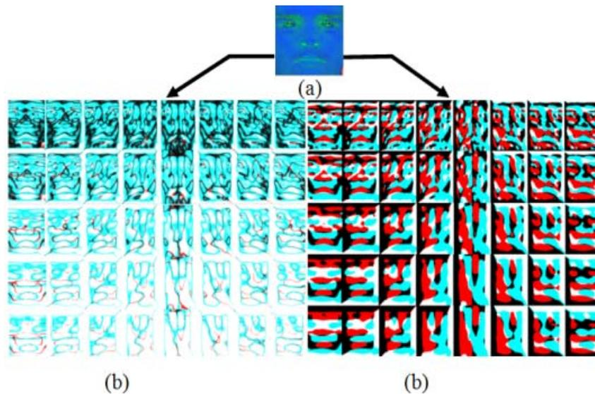
**Fig. 3.** Results of the convolution of a face image with a family of 40 Gabor filters (8 orientations (horizontal) and 5 resolutions (vertical)): (a) Image in HSV color space, (b) represents the amplitudes, and (c) phases of the convolution.
