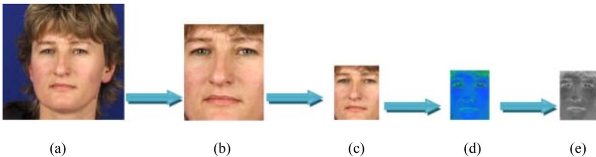
**Fig. 2.** (a) Original image, (b) Image cut, (c) Image decimate, (d) Image system HSV, (e) the S compose (e).
