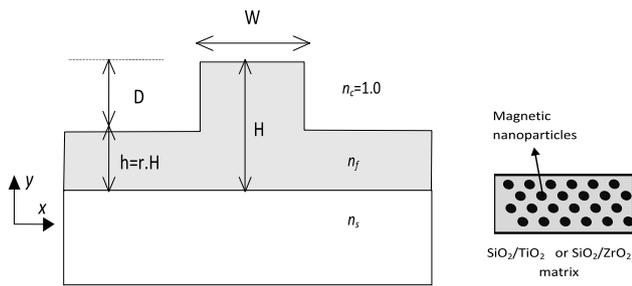
**Fig. 1** Schematic representation of a Rib waveguide. Structural parameters are the height  $h$  and the width  $w$  and refractive-index  $n_s, n_f$ ,  $x$  and  $y$  denote the cross section coordinate axes, with the  $y$ -direction parallel to the substrate surface
