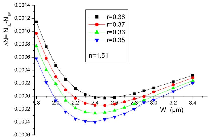
**Fig. 3** Effective-index difference calculation between quasi-TE and quasi-TM polarized modes using FMM, for refractive index of the host matrix  $n = 1.53$  at  $\lambda = 1550$  nm
