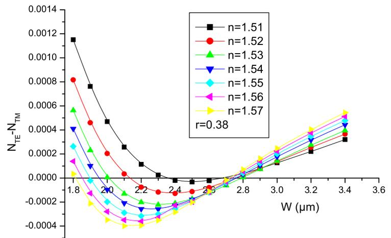
**Fig. 6** Waveguide width influence on etching depth in the structure to support zero birefringence for refractive index of the host matrix  $n = 1.51, n = 1.52, n = 1.53, n = 1.55$  and  $n = 1.57$  at  $\lambda = 1550$  nm
