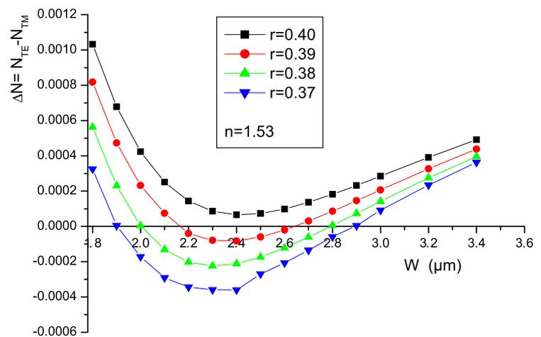
**Fig. 4** Effective-index difference calculation between quasi-TE and quasi-TM polarized modes using FMM, for refractive index of the host matrix  $n = 1.56$  at  $\lambda = 1550$  nm
