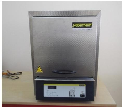
**Figure II.2:** Four Nabertherm 30-3000 ° C controllers B170.
