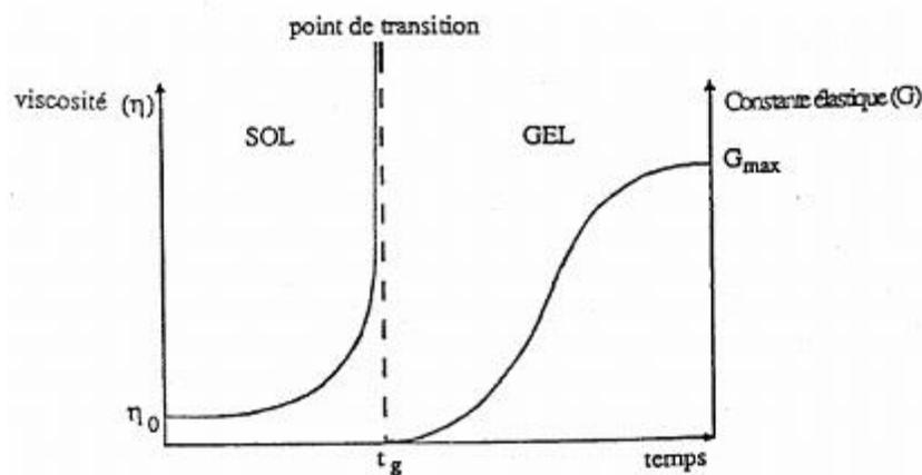
Figure III.4) Evolution of the viscosity of the solution and of the elastic constant of the gel. the Point  $t_g$  is the time after which the sol-gel transition is reached [65].
