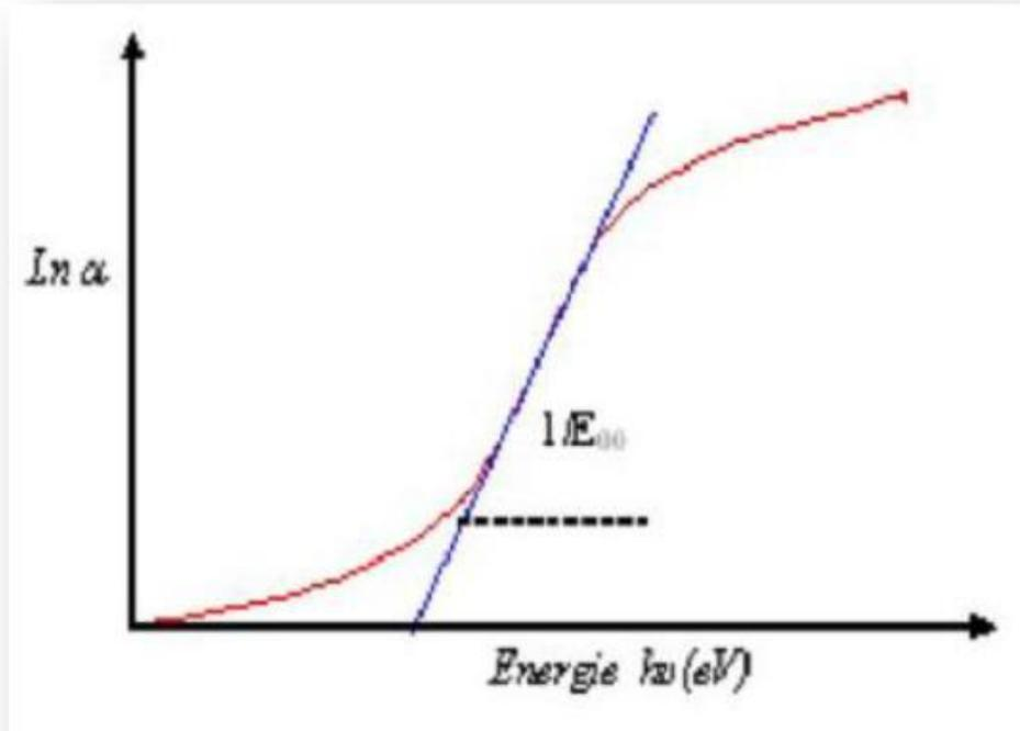
Figure II.18): Determination of the disorder by extrapolation starting from the variation of  $\ln(\alpha)$  has in function of  $hv$  [45].
