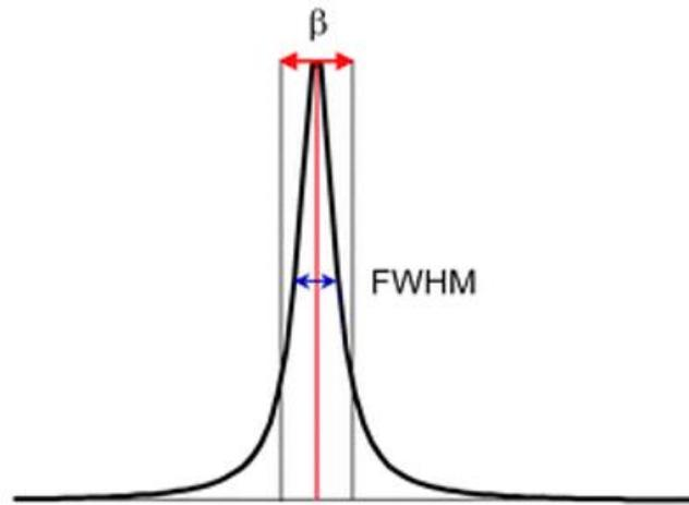
Figure II.14): Illustrate the peak widths FWHM ( $\Delta\theta=\beta$ ). [37]
