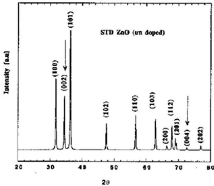
Figure II.12) Spectrum of X-ray diffraction (XRD), by a ZnO stoichiometric powder. (ASTM 36-1451) [41]
