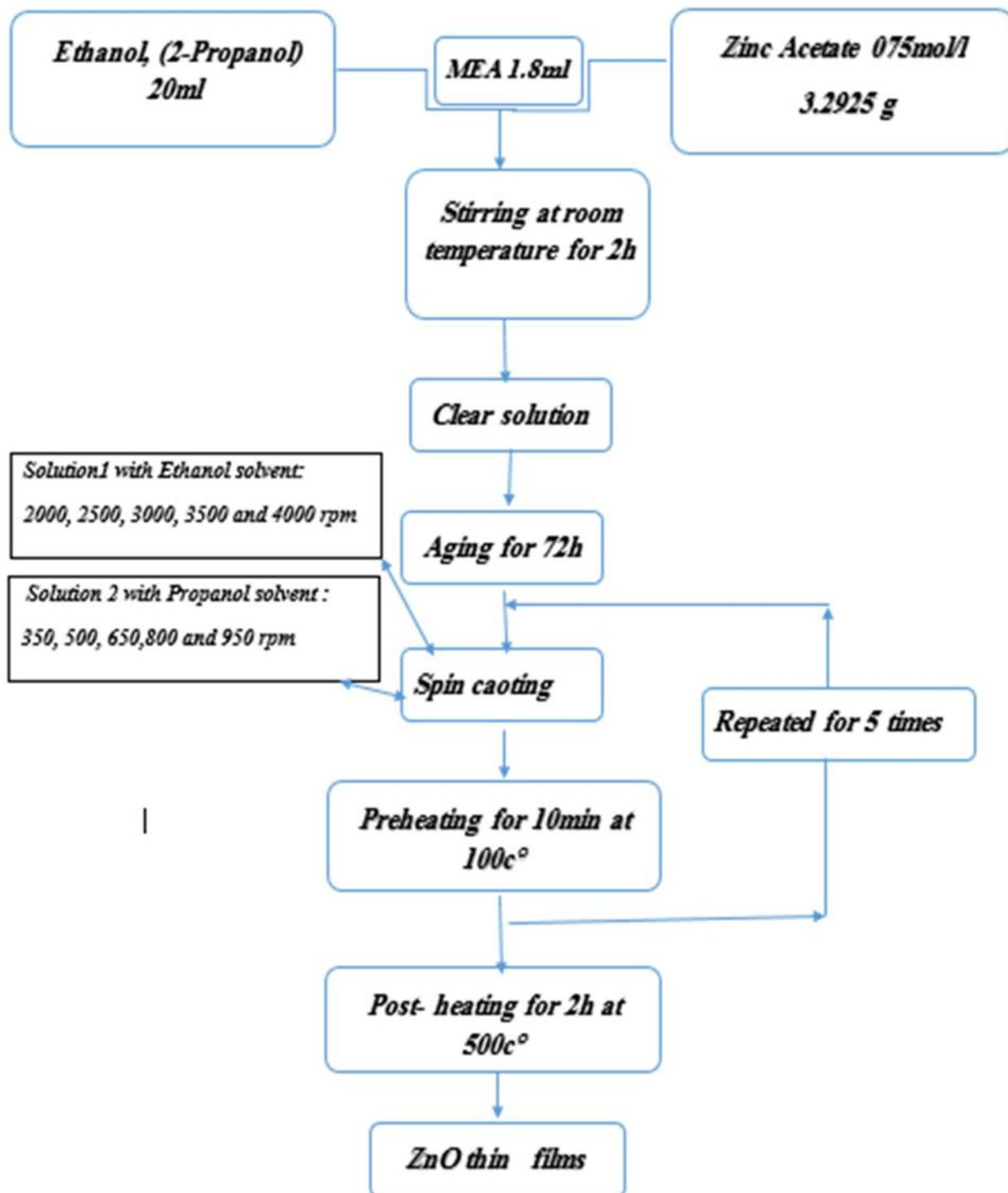
Figure IV.4).Flow chart of sol–gel method for preparation of ZnO thin films.
