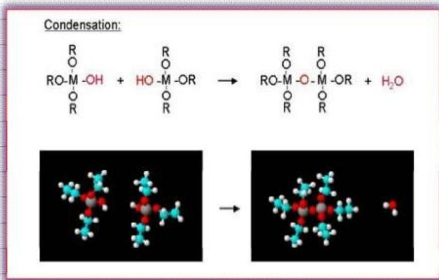
Figure III-3): condensation process [64]
