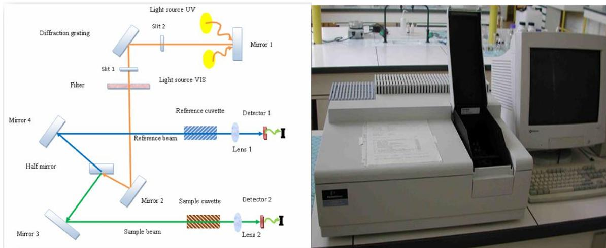
Figure II.15) The principle of operation of UV-visible spectrophotometer [30]
