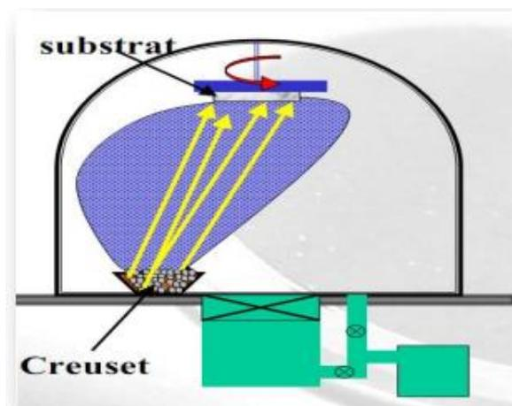
Figure II.2): Vacuum evaporation principle [33]
