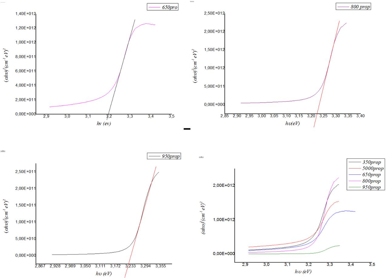
Fig.IV.20 : Optical gap of ZnO thin films for each rotation speed.
