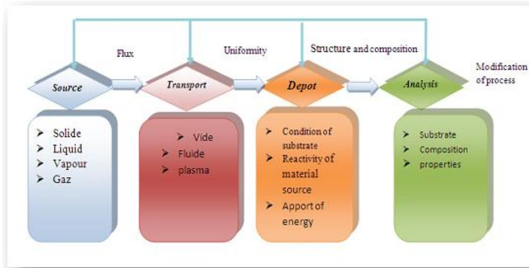
Figure II.1: Diagram presents steps of manufacturing process of thin film [30]
