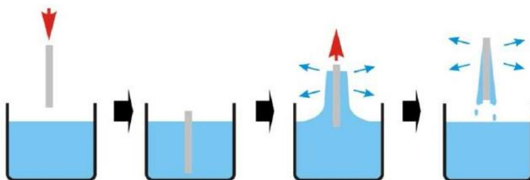
Figure III-5) Deposition of thin films by dipping-drawing [69].
