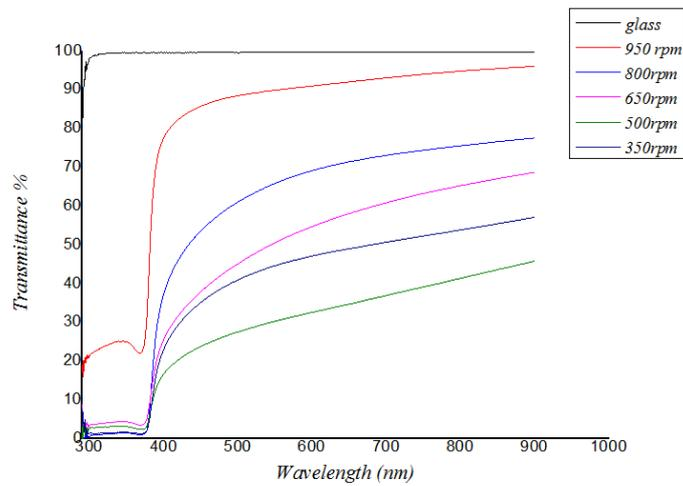
Fig.IV.19: Optical transmittance spectra of ZnO thin films.
