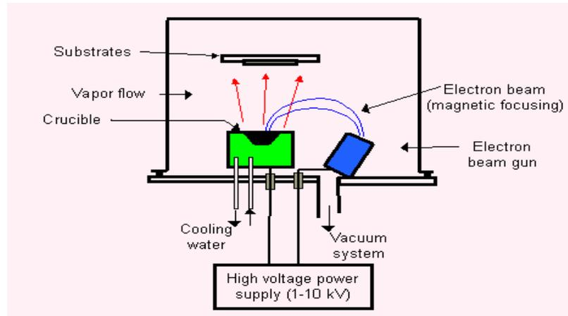
Figure II.3) General diagram of Electron Beam Evaporator [35]
