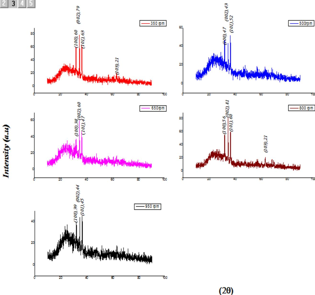
Figure IV.15: Evolution of the spectra of X-rays diffraction of ZnO thin films for differences Rotational speeds solution 2 (Propanol)
