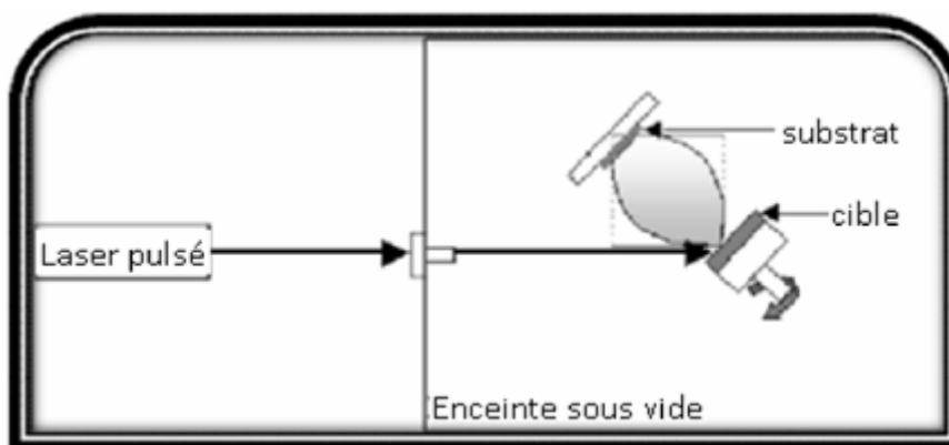
Figure II.6) Schematic of Pulsed Laser Deposition [37]
