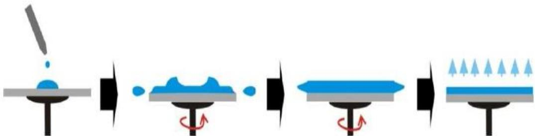
Figure III-7)The four steps of spin coating [69]
