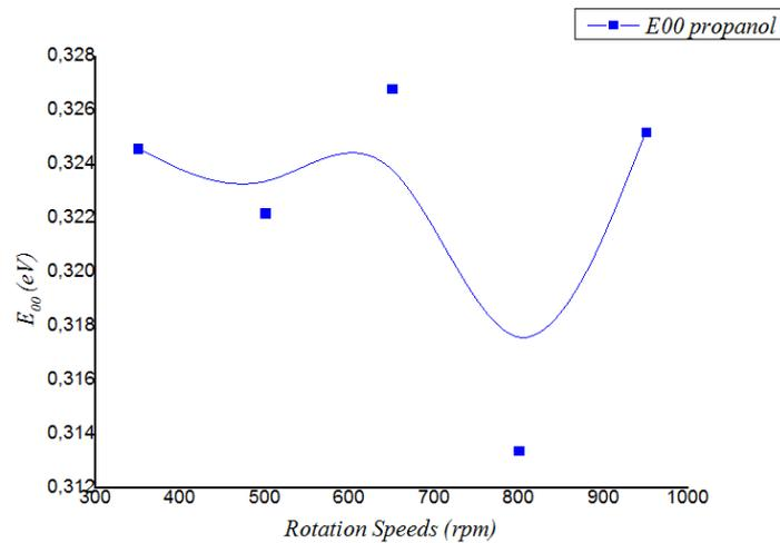
Fig. IV.23: The  $E_{00}$  value of the ZnO thin film as a function of rotation speeds
