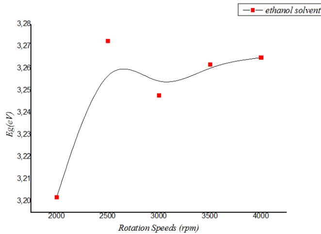
Fig. IV.12 :The Gap value of the ZnO thin film as a function of rotational speed
