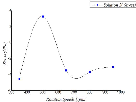
Fig. IV.18: The Stress of the ZnO thin film as a function of rotation speeds
