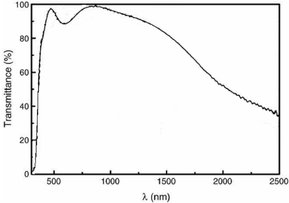
Fig.1.8) Transmission of optical thin film ZnO: Al annealed at 500 ° C [25].
