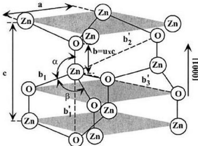
Figure I-6 ) Schematic representation of a wurtzitic ZnO structure having lattice constant  $a$  in the basal plane and  $c$  in the basal direction;  $u$  parameter is expressed as the bond length or the nearest-neighbor distant  $b$  divided by  $c$  (0.375 in ideal crystal), and  $\alpha$  and  $\beta$  ( $109.47^\circ$  in ideal crystal) are the bond angles.[21]
