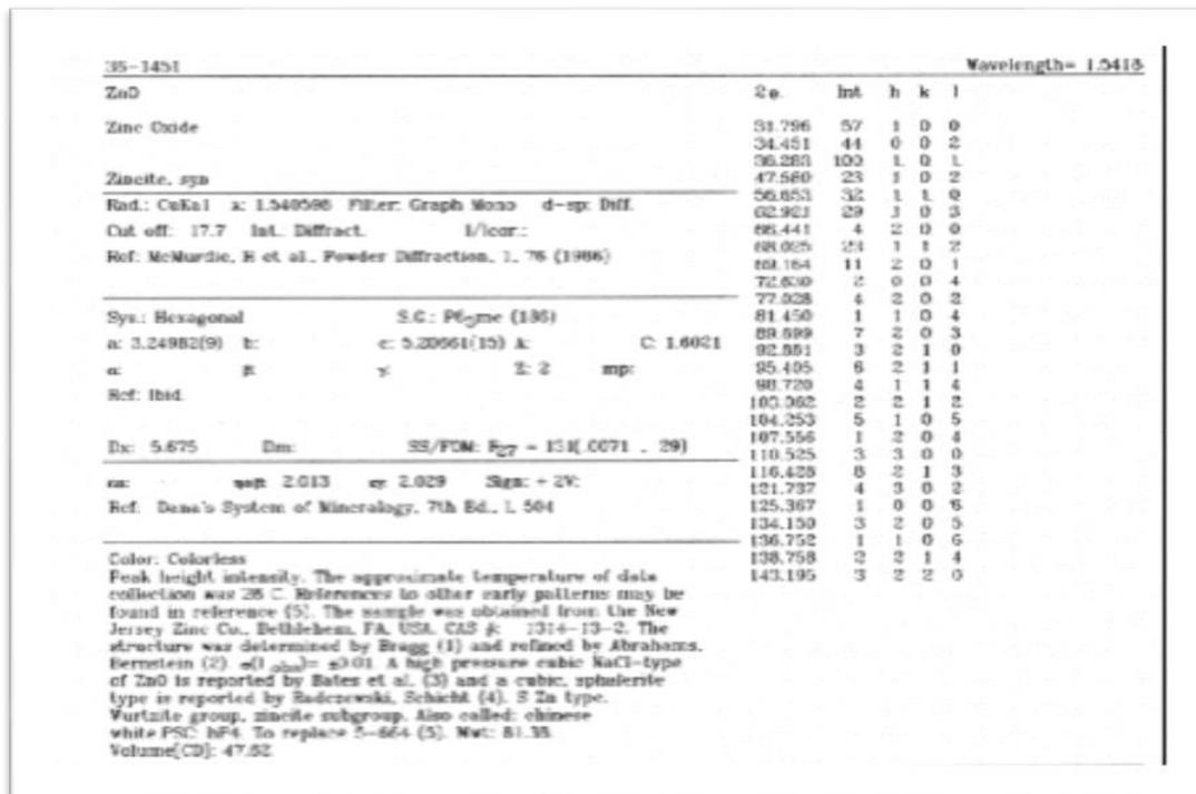
Figure IV.6): ASTM file of ZnO film [ 71]
