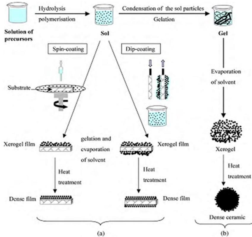
**Fig IV. 1.** Overview showing two synthesis examples by the sol–gel method; (a) films from a colloidal sol; (b) powder from a colloidal sol transformed into a gel [59]
