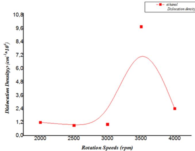
**Fig. IV.9 :** The dislocation densities of the ZnO thin film as a function of rotation speeds
