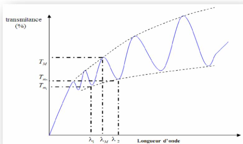
Fig.II.16): Method of interference fringes of  $s$  to determinate the thickness [36]
