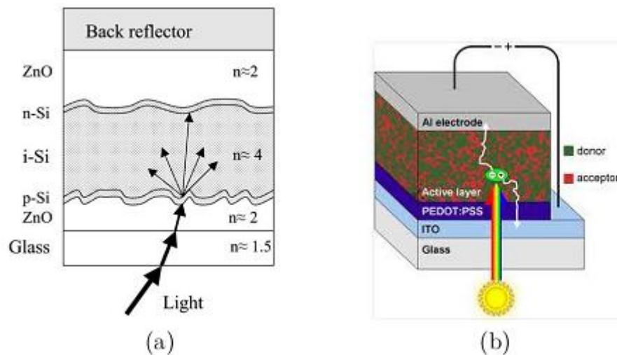
Figure 1.4: A typical architecture of a) thin film solar cell and b) organic solar cell [29].
