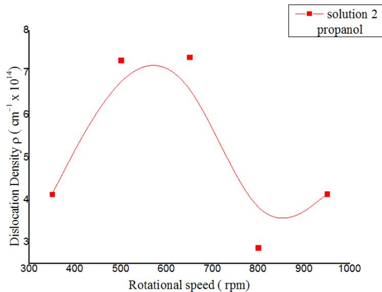
*Fig. IV.19 : The dislocation densities of the ZnO thin film as a function of rotation speeds*
