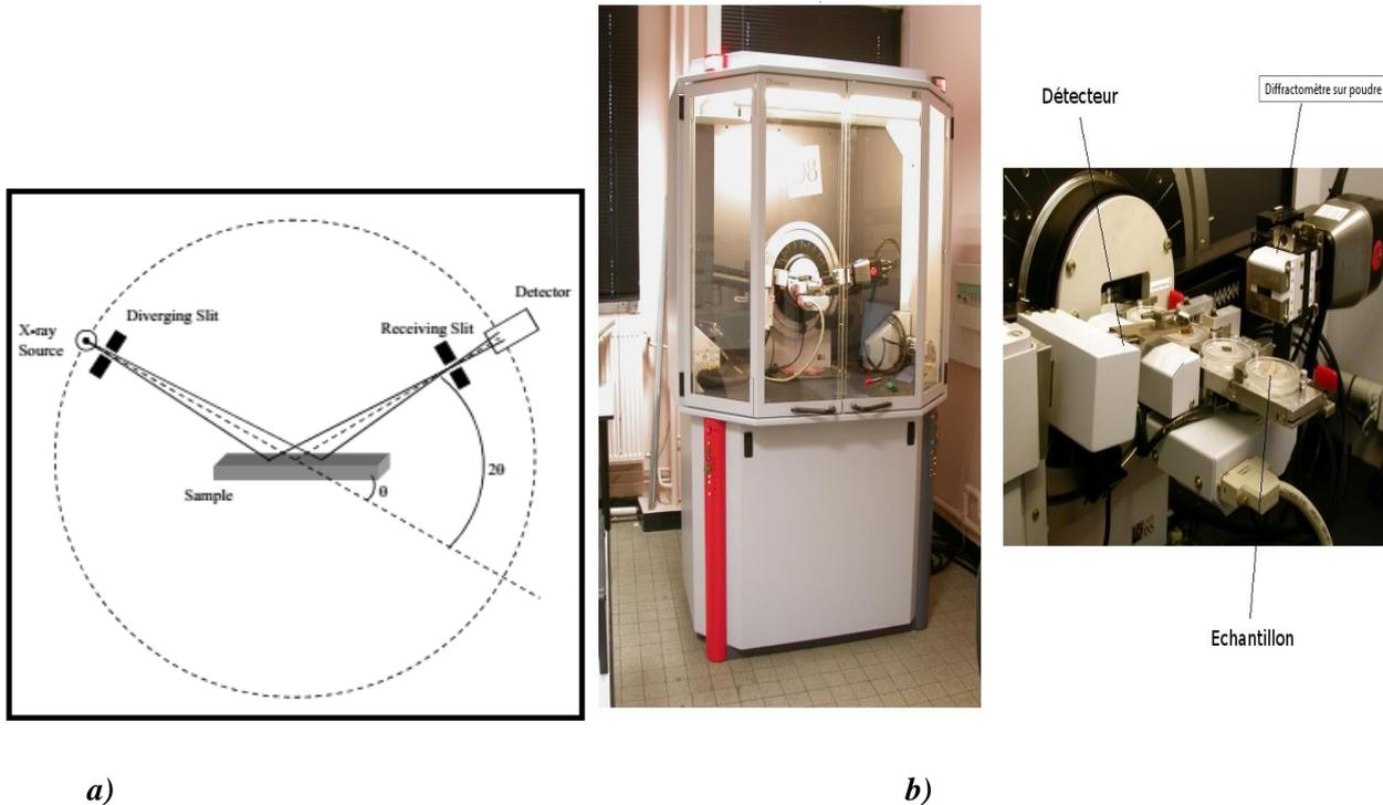
Figure II.11) a) Schematics of X-ray diffractometer. [41] b) Bruker's X-ray Diffraction D8-Discover instrument[36]
