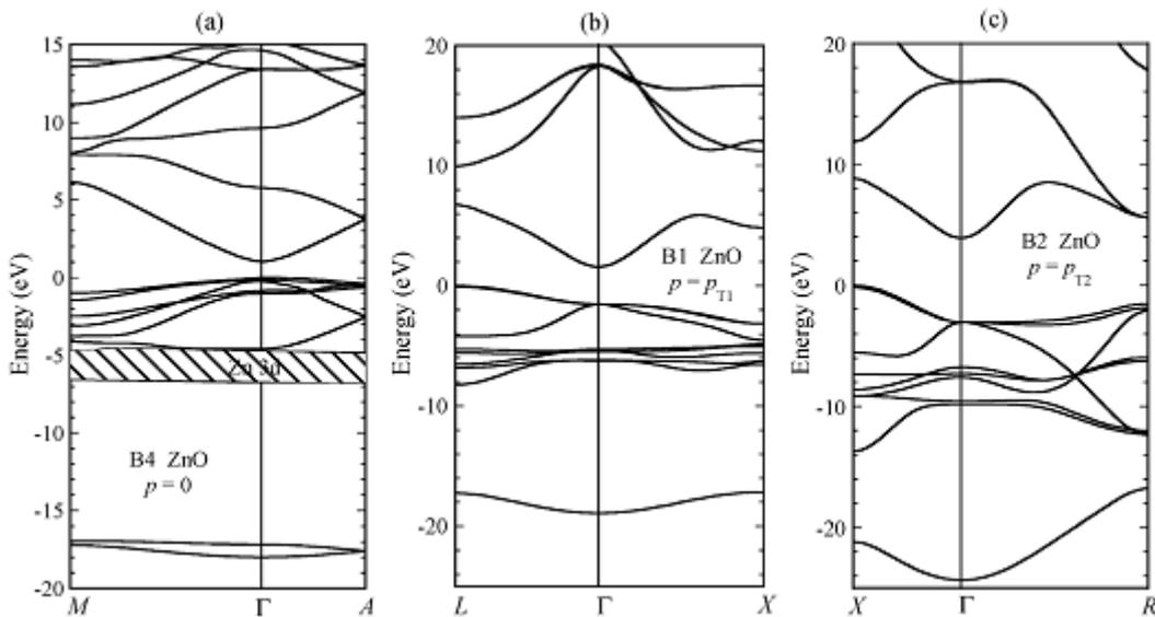
**Figure 1.7** Band structure for ZnO : (a) B4 structure at  $p = 0$ , (b) B1 structure at  $p = p_{T1}$ , (c) B2 structure at  $p = p_{T2}$ . [24].
