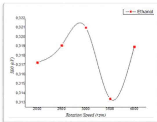
Fig. IV.14 :The  $E_{00}$  value of the ZnO thin film as a function of rotation speed
