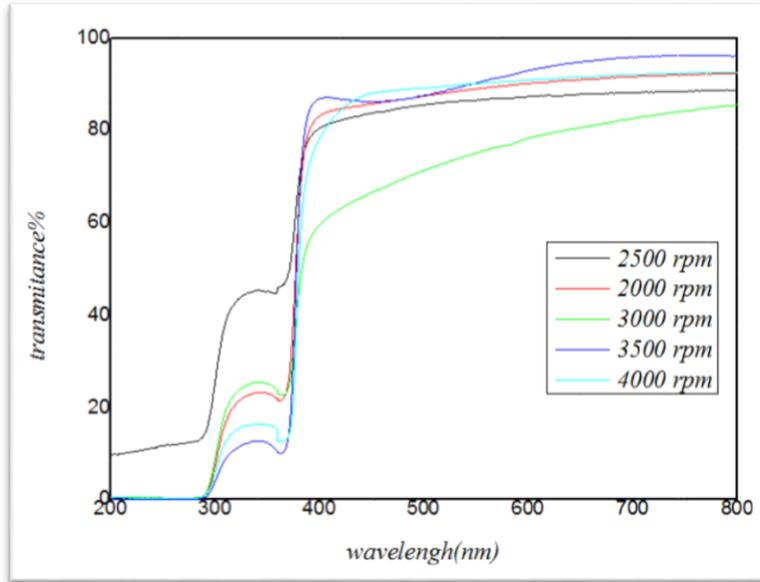
Fig.IV.10 : Optical transmittance spectra of ZnO thin films.
