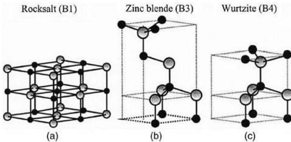
Figure I-5) Stick and ball representation of ZnO crystal structures: (a) cubic rock-salt(B1), (b) cubic zinc blend (B3), and (c) hexagonal wurtzite (B4). The shaded gray and black spheres denote Zn and O atoms, respectively.[21]
