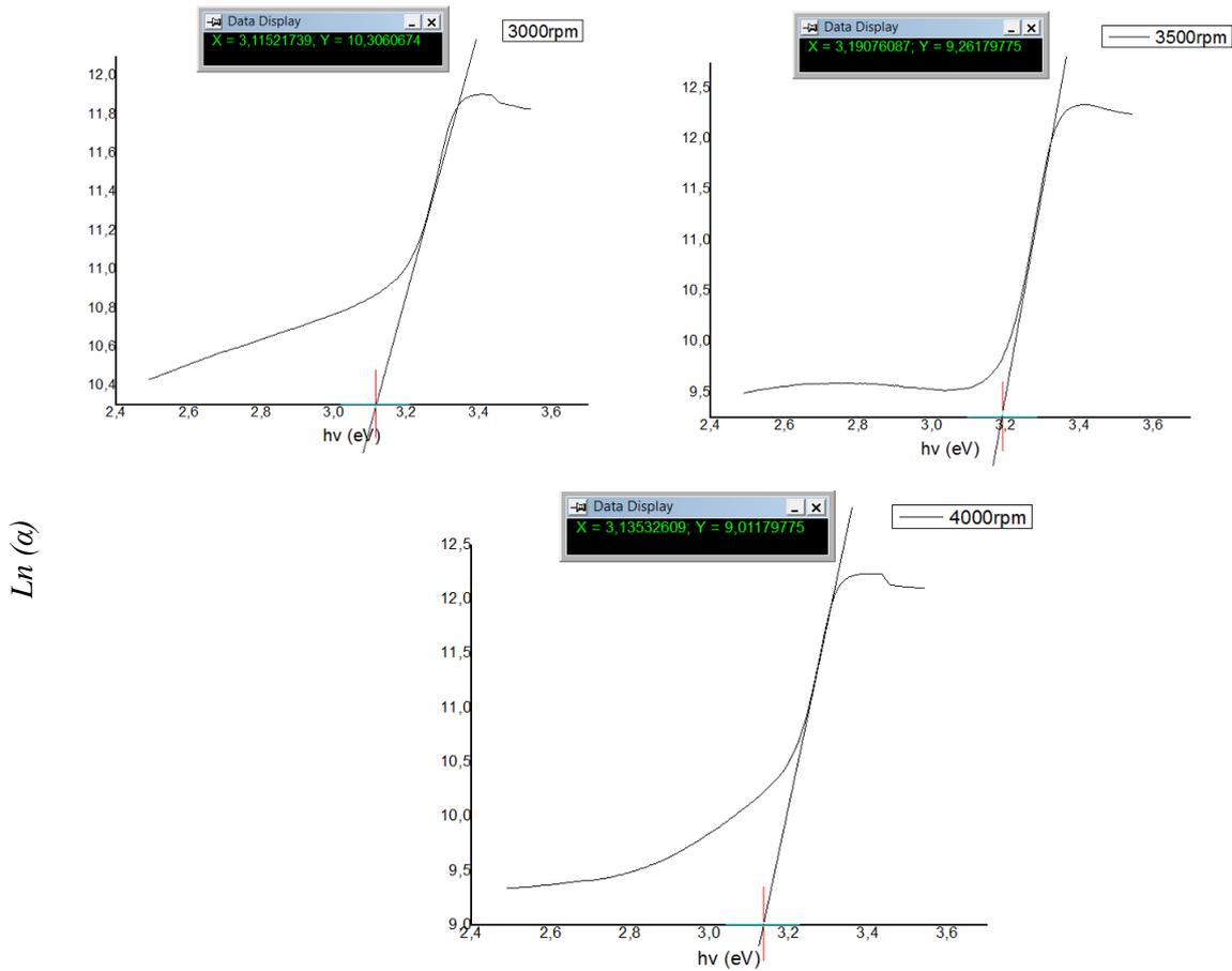
Fig. IV.13 : The  $E_{00}$  value of the ZnO thin film as a function of rotational speeds
