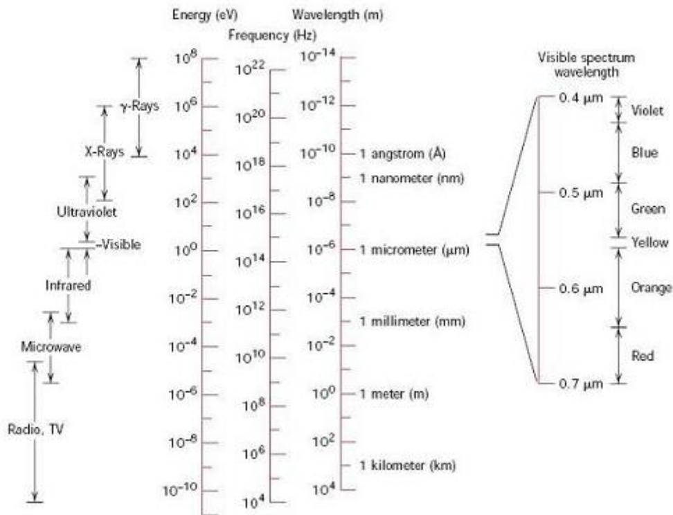
Figure 1-2 The spectrum of electromagnetic radiation , including wavelength ranges for the various colors in the visible [12]
