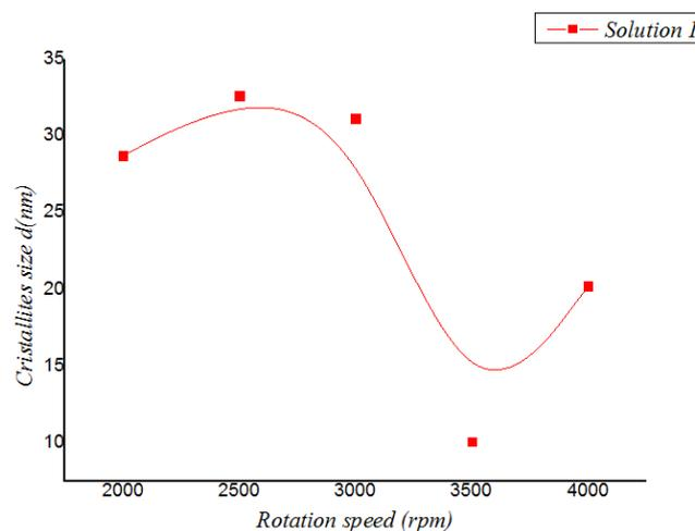
Fig. IV.6: Average crystallite sizes of the ZnO thin film as a function of The Rotation Speeds
