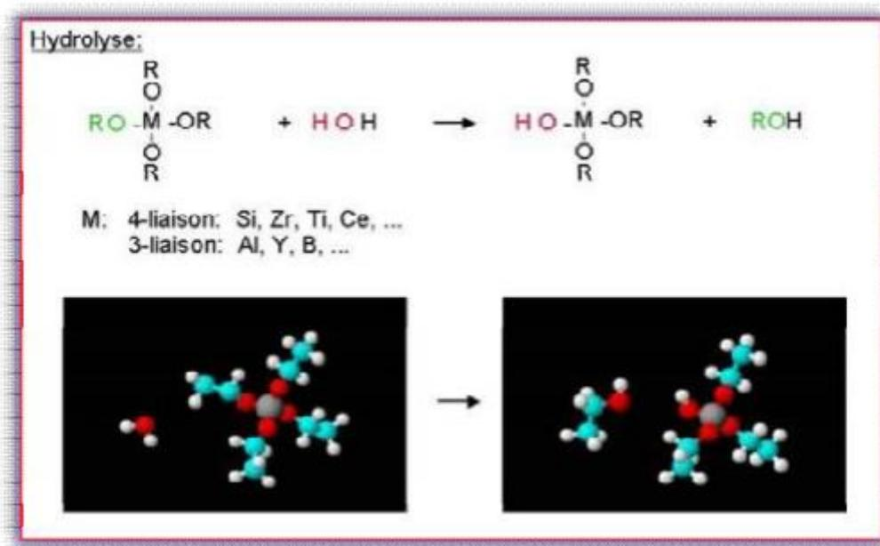
Figure III-2): schematization the hydrolysis process [64]
