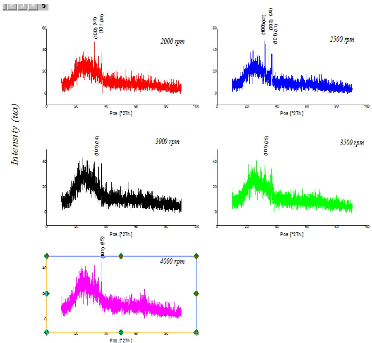
Figure IV.5) Evolution of the spectra of X-rays diffraction of ZnO thin films for differences in rotation speeds solution 1 (Ethanol)
