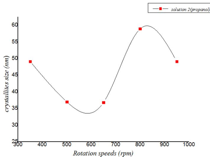
Fig. IV.16 : Average crystallite sizes of the ZnO thin film as a function of The Rotational Speeds
