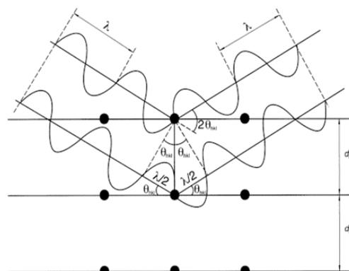
Figure 2.9.33-1. - Diffraction of X-rays by a crystal according to Bragg's law
