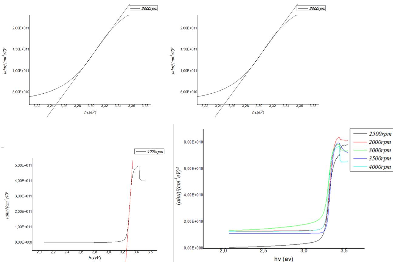
Fig.IV.11 : Optical gap of ZnO thin films for each rotational speed.
