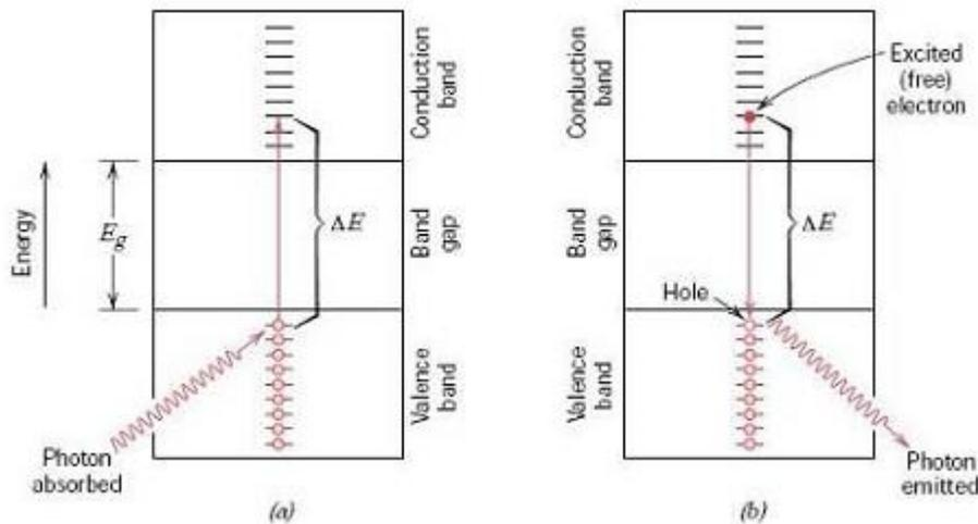
Figure I-1 (a) Mechanism of photon absorption for non-metallic materials in which an electron is excited across the band gap, leaving behind a hole in the valence band. The energy of the photon absorbed is  $\Delta E$ , which is necessarily greater than the band gap energy  $E_g$ . (b) Emission of a photon of light by a direct electron transition across the band gap [12]
