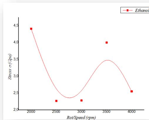
Fig. IV.8 : The Stress of the ZnO thin film as a function of rotation speeds
