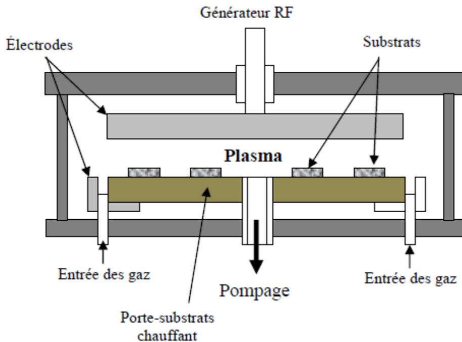
Figure II.9) Principe of the PECVD system [39]
