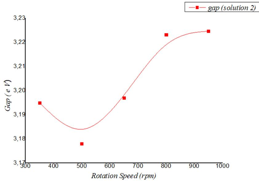
Fig.IV. 21 :The Gap value of the ZnO thin film as a function of rotation speed
