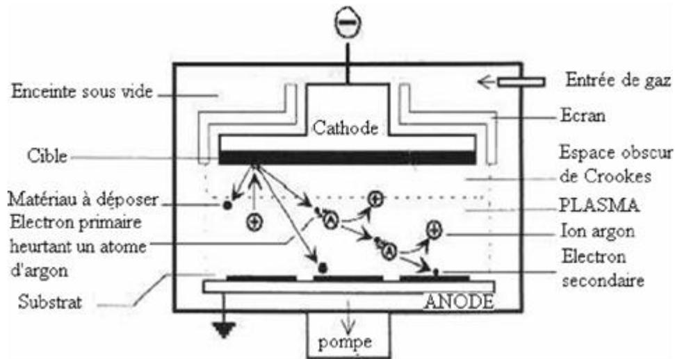
Figure II.5) Schematic of the principle of Sputtering [36]
