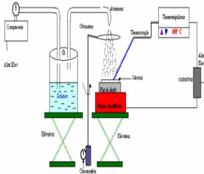
Fig II.10 : pyrolysis spray [40]
