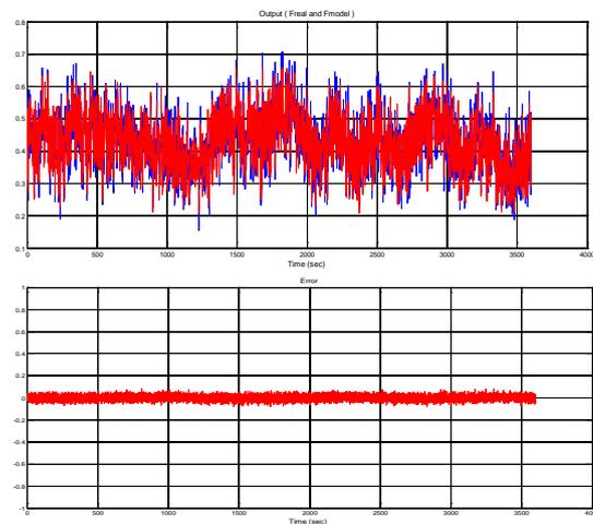
Fig. 8 (up) Actual output  $F$  with the estimated  $F'$ . (down) Residual  $R_F(t)$
