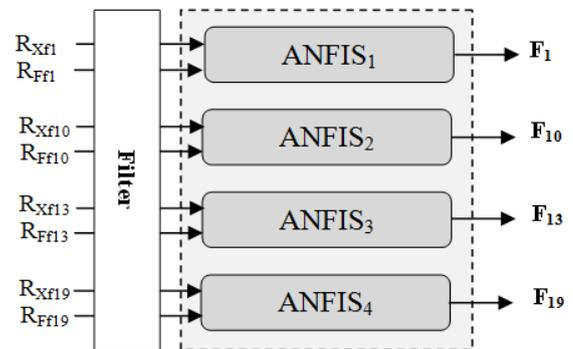
Fig. 15 Diagram bloc of the faults diagnosis system
