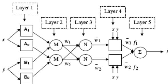
Fig. 1 ANFIS structure for TS system with 2 inputs-one output
