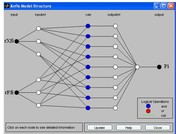
Fig. 14 The structure of fault classifier
