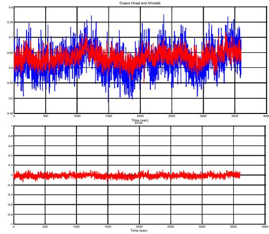
Fig. 7 (up) Actual output  $X$  with the estimated  $X'$ . (down) Residual  $R_X(t)$
