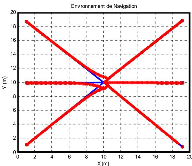
Figure 12: Straight paths following using neural controller
