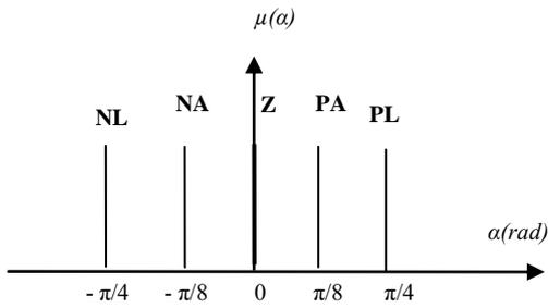
Figure 5: The membership functions of the output control.
