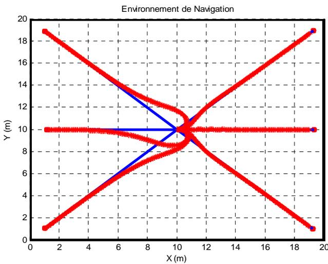
Figure 11: Straight paths following using fuzzy controller
