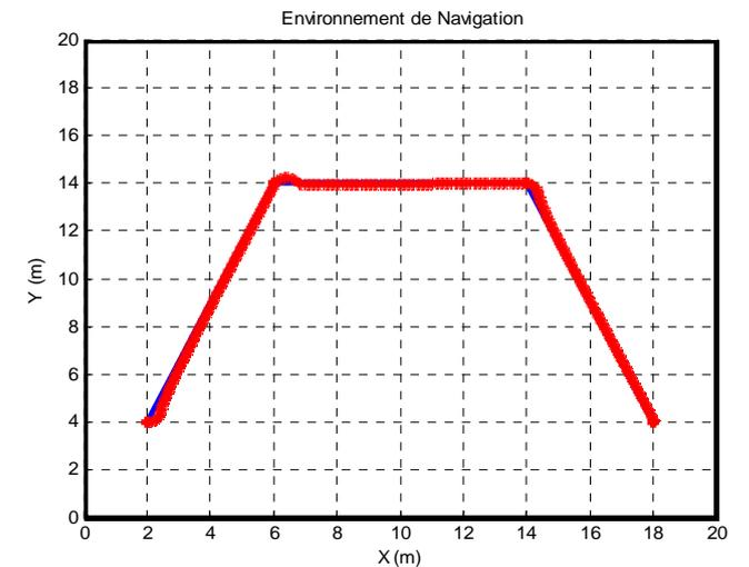
Figure 13: Robot trajectory for trapezoidal reference path using fuzzy controller (a) and neural controller (b).
