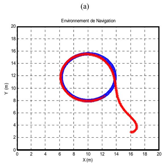
Figure 17: Pursing a target with a curve path using fuzzy controller (a) and neural controller (b).
