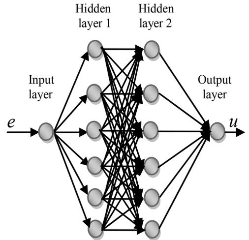
Figure 6: The proposed neural network structure
