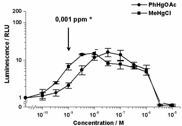
Fig. 2 : Response curve of the mercury sensor.
