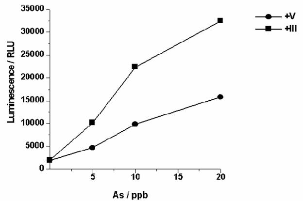
Fig. 3 : Response curves of the Arsenic-III and Arsenic-V sensors
