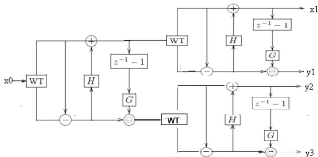
Figure 2: The analysis operation in 2D (three stage lifting scheme)
