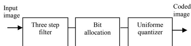
Figure 1: Principle of the compression scheme
