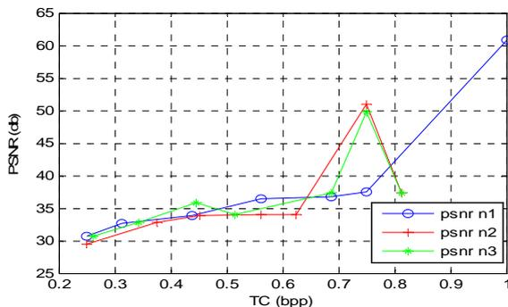
Figure 11: Effect of quantization on the 9/7 filters for Montage Image
