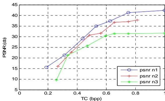
Figure12: Effect of quantization on the filters nonlinear three steps for Slope Image
