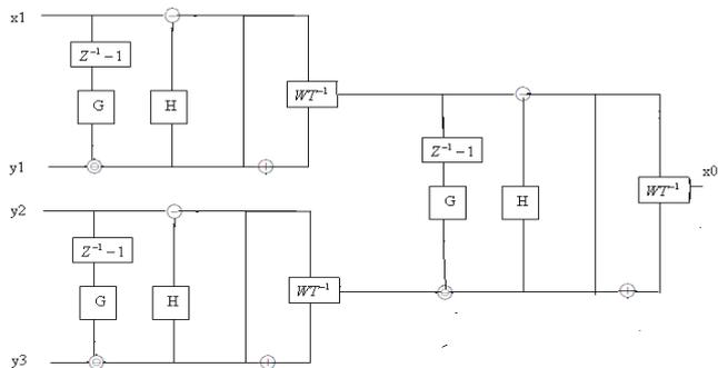
Figure 3: The synthesis operation in 2D (three stage lifting scheme)
