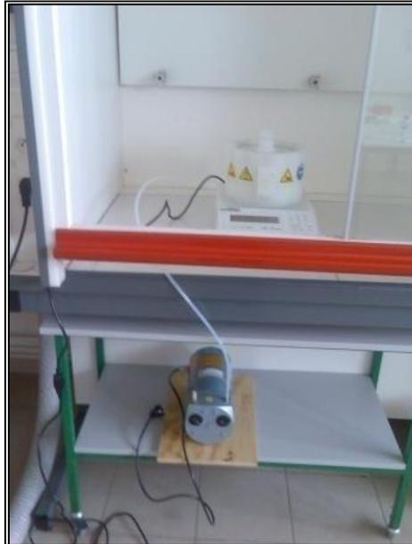
**Figure III.7:** *Technique de Spin-coating (Spin-coater type spin150)*
