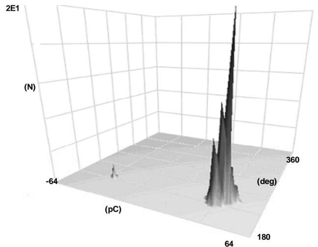
Figure 14: Partial discharge pattern with space charge.
