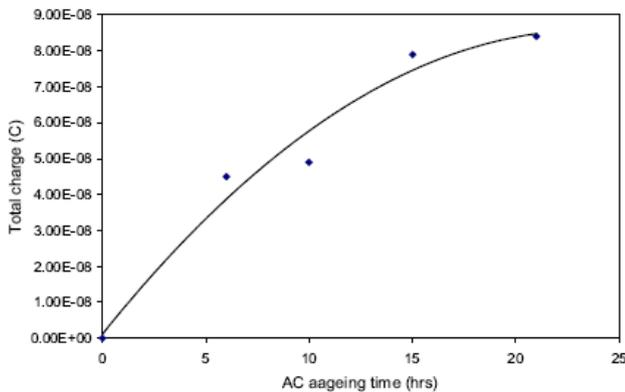
Figure 1 : Relationship between the total charge and ageing time at 50 kV/mm [5]
