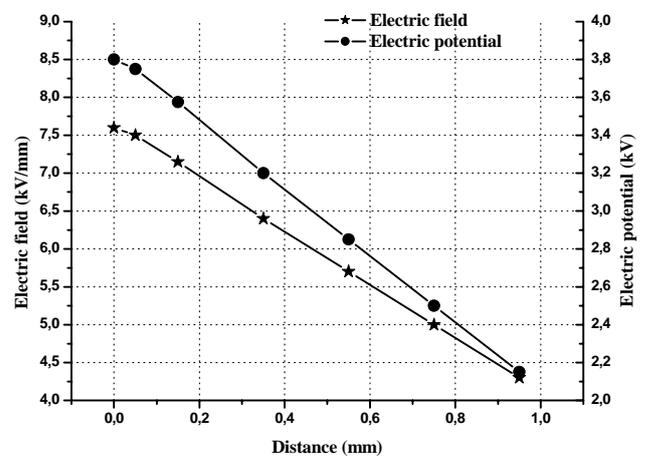
Figure 7: Electric field and electric potential distribution within the cavity as a function of the distance.
