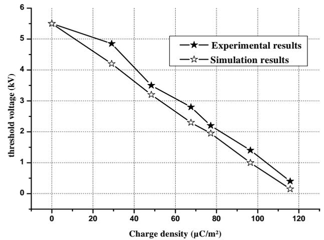
Figure 17: Threshold voltage of PD ignition as a function of charge density
