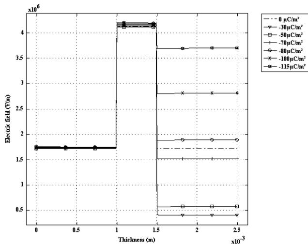
Figure 16: Electric field distribution within the cavity as a function of charge density
