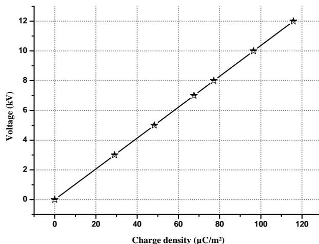
Figure 10: Applied DC voltage as a function of charge density
