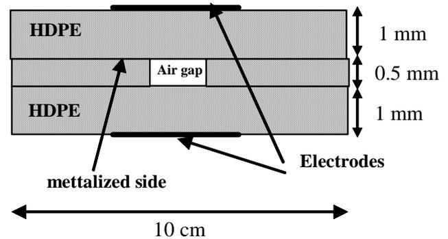
Figure 2 : Transverse section of the sample.
