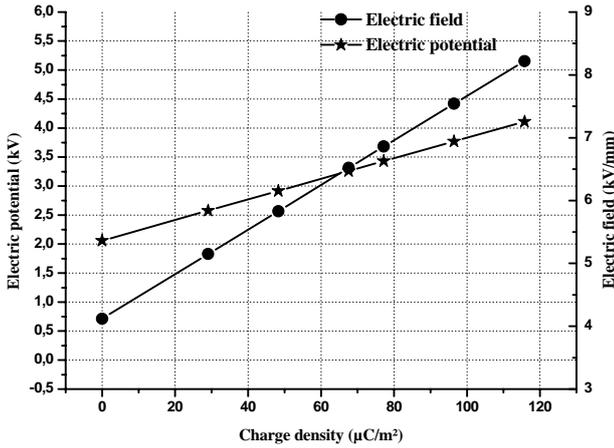
Figure 12: Electric field distribution within the cavity as a function of charge density
