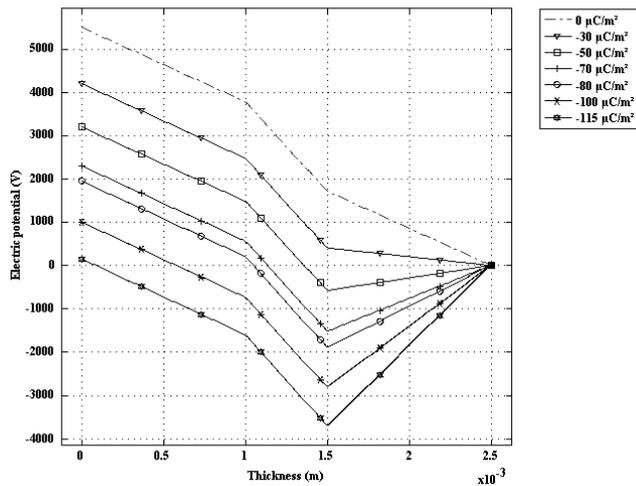
Figure 15: Electric potential distribution within the cavity as a function of charge density
