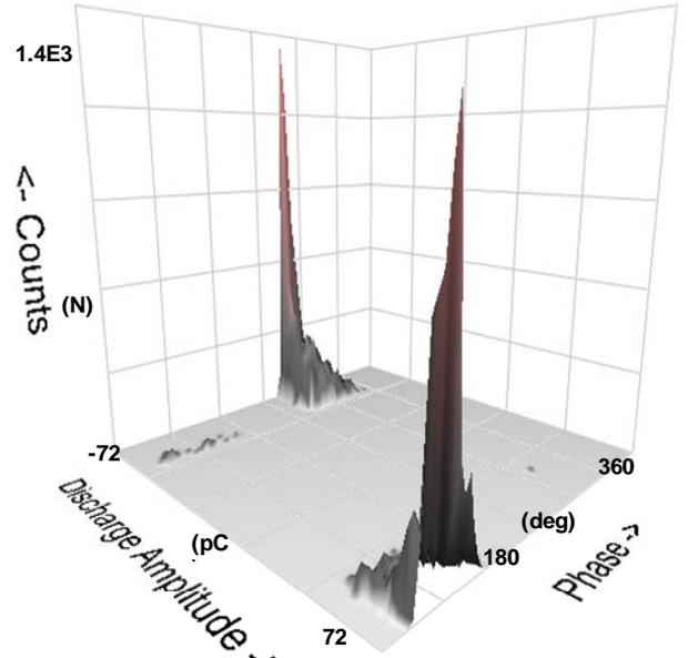
Figure 13: Partial discharge pattern before the application of a DC voltage.
