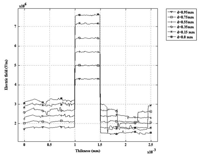
Figure 6: Electric field distribution in the sample as a function of distance which separates space charge and the cavity
