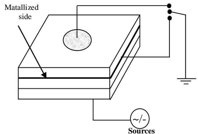
Figure 3: Configuration of the sample including the two supply voltage sources
