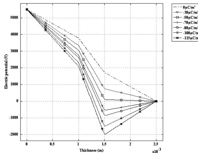
Figure 11: Electric potential distribution within the sample as a function of charge density
