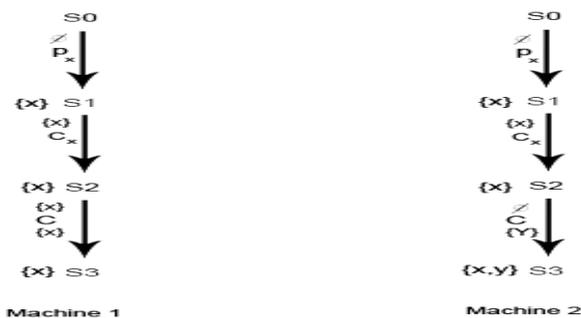
Figure 1: Maximality-based Labeled Transition Systems of machines M1 and M2
