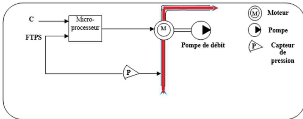
Figure.III.11.Simple Diagram of the Pressure Control Loop
