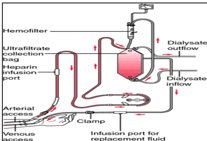
**Figure II.4. A hemodialysis circuit**
