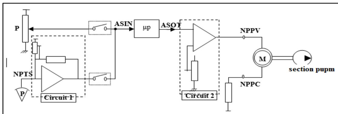
Figure III.12. Simplified Electrical Circuit Pressure
