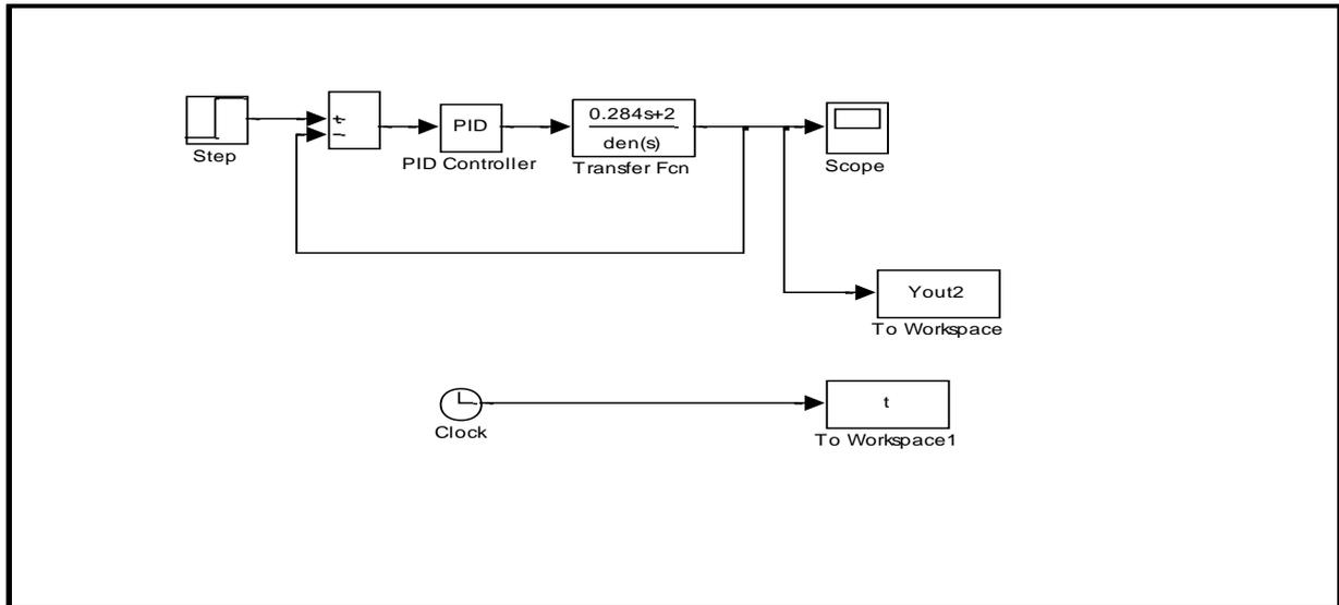
Figure.III.18. Simulink model with PID
