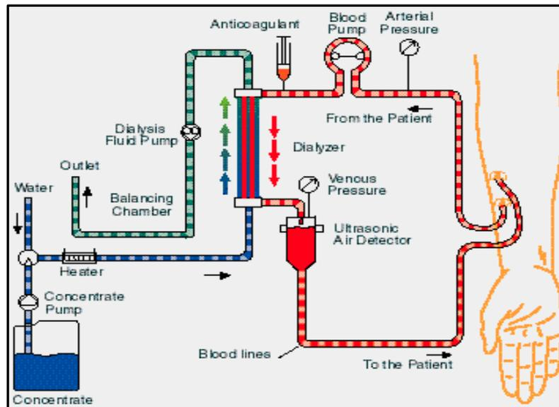
**Figure II.3. Principle of hemodialysis**
