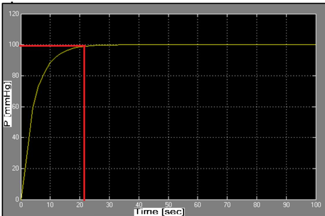
Figure III.21.Response with Proposed ABC-PID
