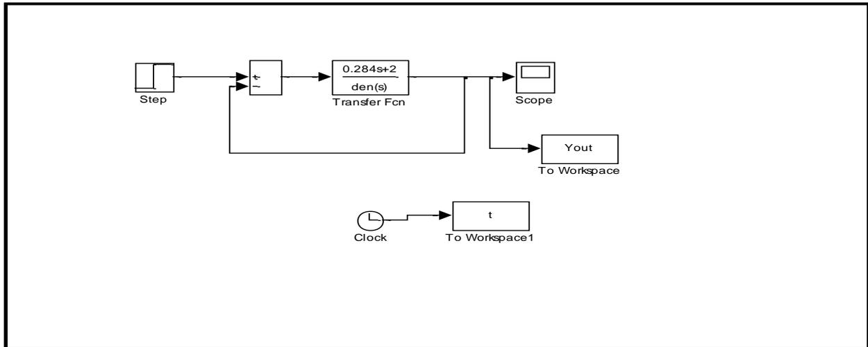
Figure III.16. Simulink Model with Closed Loop
