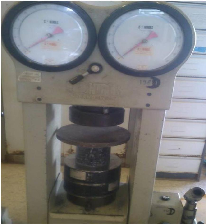
**Photo III.7 :** Machine de compression.
