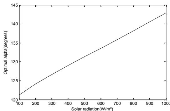
Figure 8: Optimal firing angle alpha
