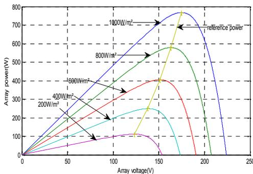
Figure 2: Power voltage characteristics of the PV array at T=25 °C at different solar radiation levels
