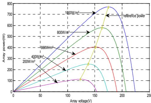
Figure 2: Power voltage characteristics of the PV array at T=25 °C at different solar radiation levels
