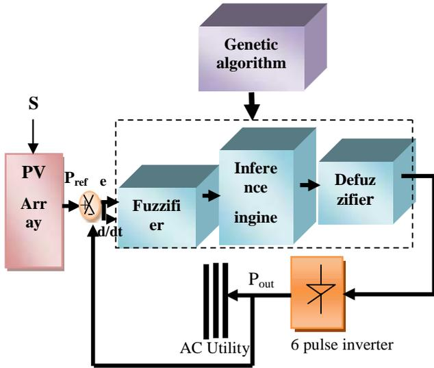
Figure 3: Control scheme for the photovoltaic power plant
