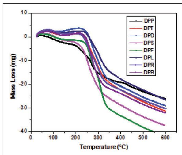
**Figure 7.** Thermogravimetric curves of date palm wood: (DPP)Petiole, (DPT)Thorns, (DPD)Pedicels, (DPS)Spathe, (DPF)Fibrillium, (DPL)Leaflets, (DPR)Rachis, (DPB)Bunch.
