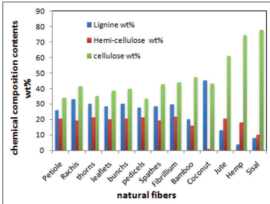
**Figure 3.** Chemical composition of date palm wood compared to other natural fibers.
