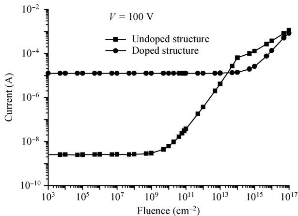
Figure 5. The reverse current versus radiation dose at 100 V.
