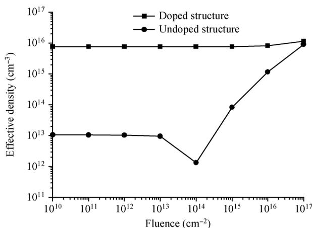
Figure 6. The effective density versus radiation dose at 100 V.
