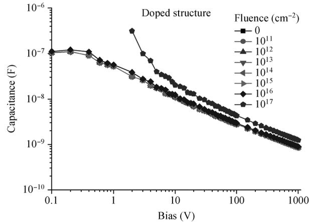
Figure 4. The capacitance–voltage characteristics for the doped sample at 300 K. The fluence is 0,  $10^{10}$  to  $10^{17}$   $\text{cm}^{-2}$  with increasing reverse current at high voltage.
