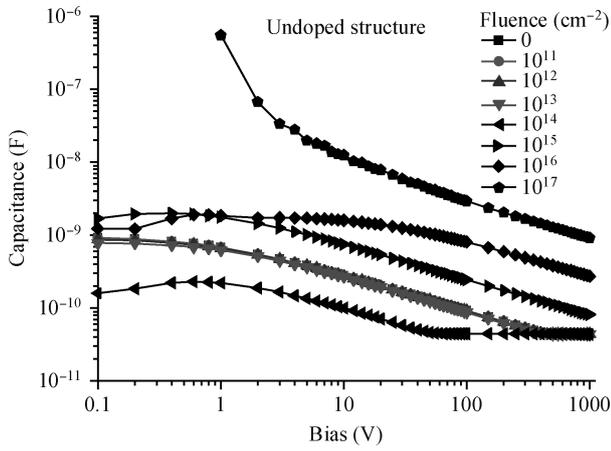
Figure 2. The capacitance–voltage characteristics for the undoped sample at 300 K. The fluence is 0,  $10^{10}$  to  $10^{17}$   $\text{cm}^{-2}$  with increasing reverse current at high voltage.
