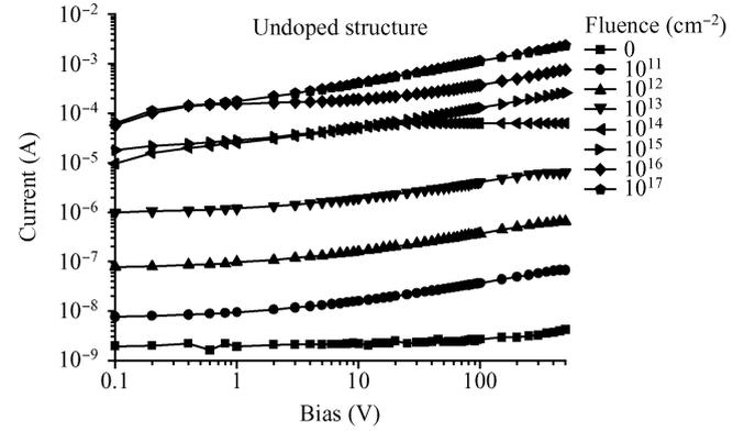
Figure 1. The reverse current–voltage characteristics for the undoped sample at 300 K. The fluence is 0,  $10^{10}$  to  $10^{17} \text{ cm}^{-2}$  with increasing reverse current at high voltage.
