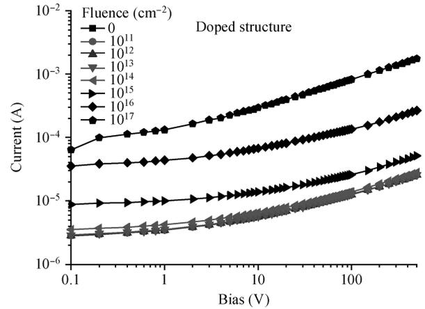
Figure 3. The reverse current–voltage characteristics for the doped sample at 300 K. The fluence is 0,  $10^{10}$  to  $10^{17}$   $\text{cm}^{-2}$  with increasing reverse current at high voltage.
