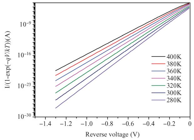
Figure 4. Semi-logarithmic  $I/(1-\exp(-qV/kT))$  versus  $V$  plot from the reverse bias  $I-V$  data in Figure 2 for Au/n-InP SD in the temperature range of 280–400 °K.
