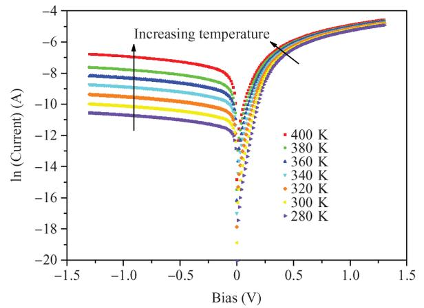
Figure 2. The simulated  $I-V$  characteristics of an Au/n-InP Schottky diode in the temperature range of 200–400 K.
