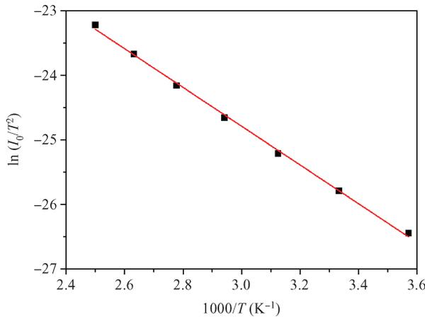
Figure 6. The Richardson plot of  $\ln(I_0/T^2)$  versus  $10^3/T$ .
