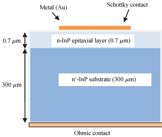
Figure 1. A two dimensional schematic cross section of the simulated Au/n-InP Schottky diode.
