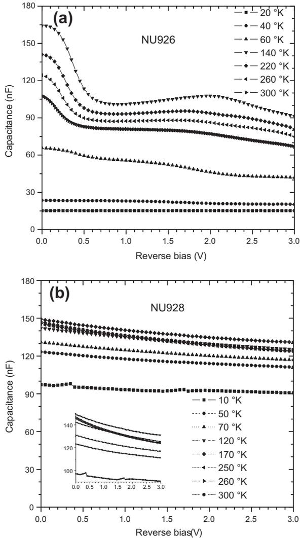
**Fig. 2.** The capacitance–voltage characteristics at different temperatures for the samples (311)A (NU926) (a) and (211)A (NU928) (b).
