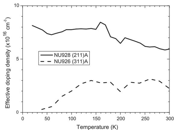
Fig. 1. The average effective density evaluated from the C–V characteristics of the (211)A and (311)A samples at different temperatures.
