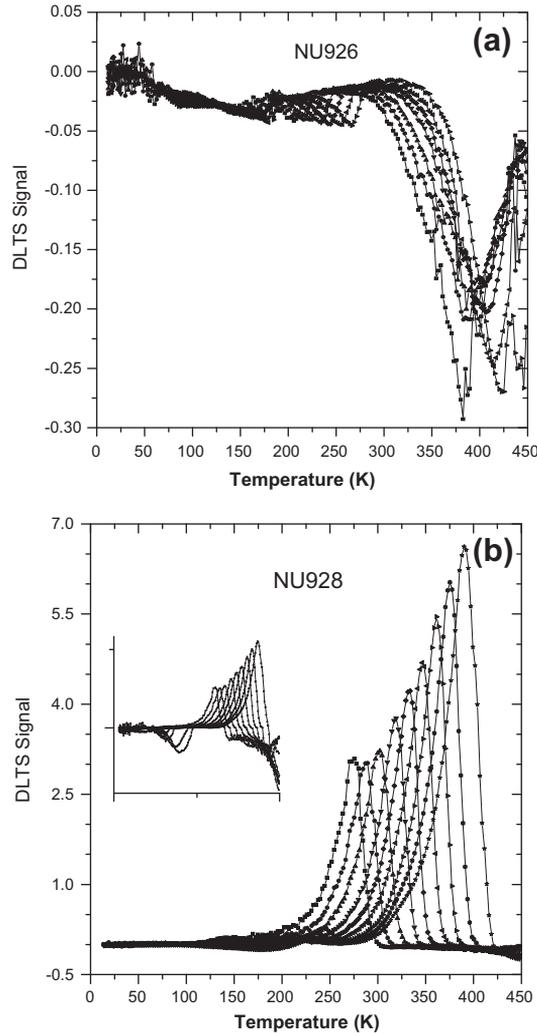
**Fig. 3.** DLTS spectra for (311)A (NU926) (a) and (211)A (NU928) (b) samples. In the insert in (b), the positive signal (electron deep levels) is divided by 20.
