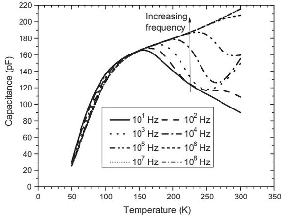
**Fig. 5.** The simulated capacitance–temperature characteristics for different frequencies in the presence of deep acceptors only (3 1 1)A sample (NU926).
