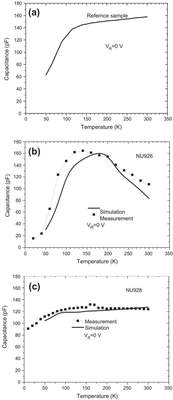
**Fig. 4.** The simulated capacitance–temperature characteristics for three samples: in the absence of deep levels [(a), reference sample], in the presence of deep acceptors [(b) (3 1 1)A sample (NU926)] and in the presence of deep acceptors and donors [(c), (2 1 1)A sample (NU928)].
