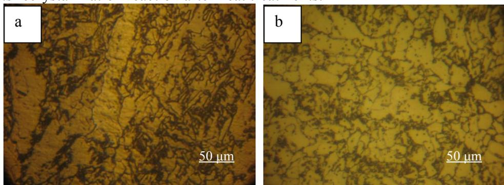
Fig. 5 Microstructures of X70 pipeline steel in weld region:
