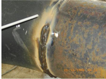
Fig. 1 X70 pipeline steel after industrial arc welding.
