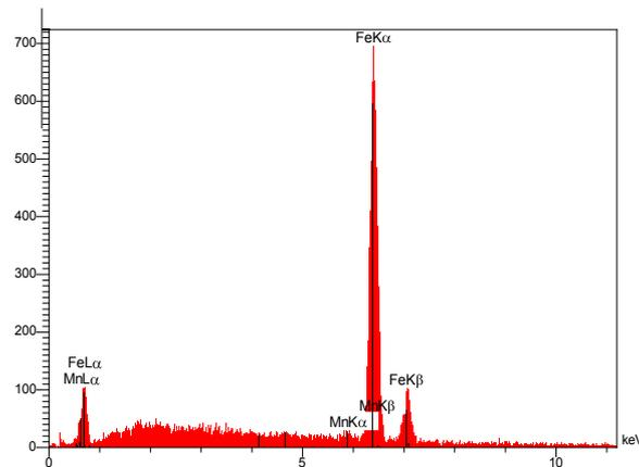
Fig. 2 Spectrum of EDAX analysis of X70 pipeline steel.
