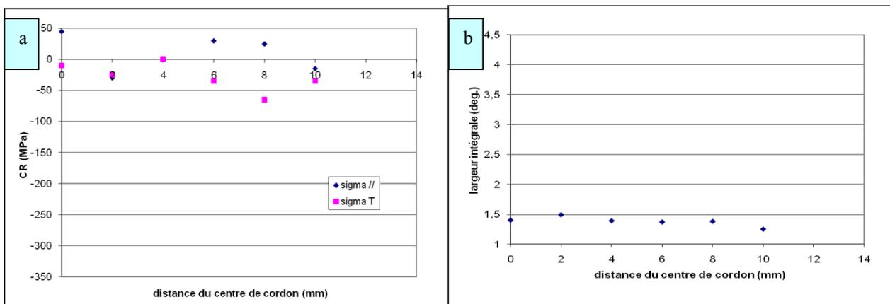
Fig. 9 : The stress distributions and (b) width peak diffraction evolution in the weld region of X70 pipeline steel heat treat 1 h at 600°C.
