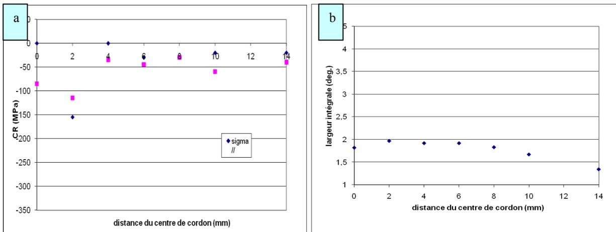
Fig. 8 : (a) The stress distributions and (b) width peak diffraction evolution in the weld region of X70 pipeline steel heat treated 1 h at 200°C.
