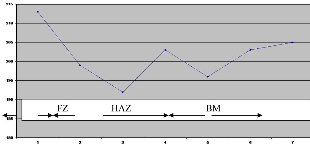
Fig. 6 Microhardness from the fusion zone ( FZ ) across the weld metal after welding of X70 pipeline steel.
