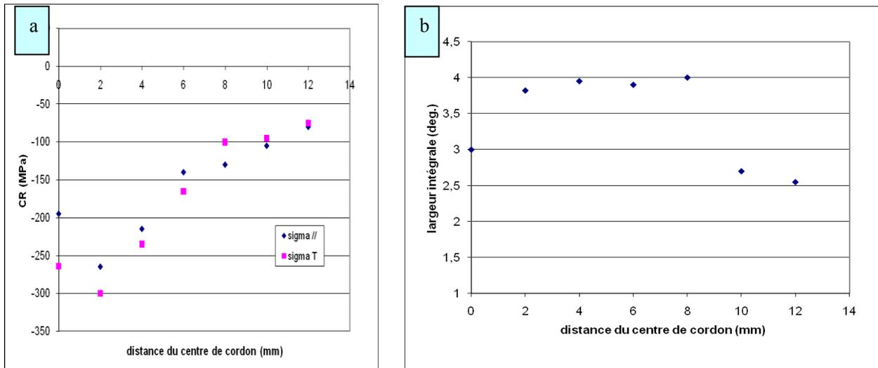
Fig.7 : (a) The stress distributions and (b) width peak evolution in the weld region of X70 pipeline steel
