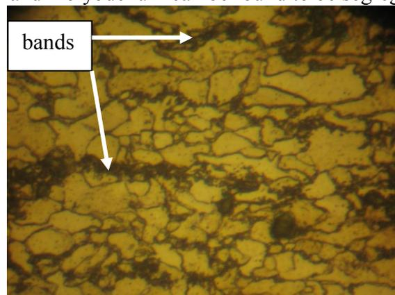
Fig. 3 Microstructure of X70 pipeline steel.
