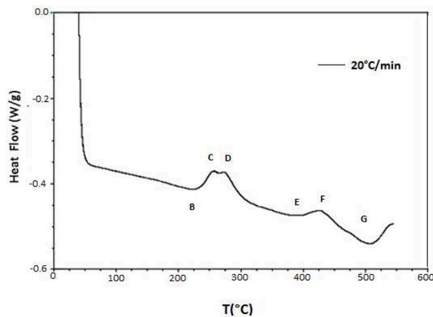
Fig. 2 DSC curve of pre-natural aged Al-Mg-Si alloy during 27 months (heating rate =20°C/min).
