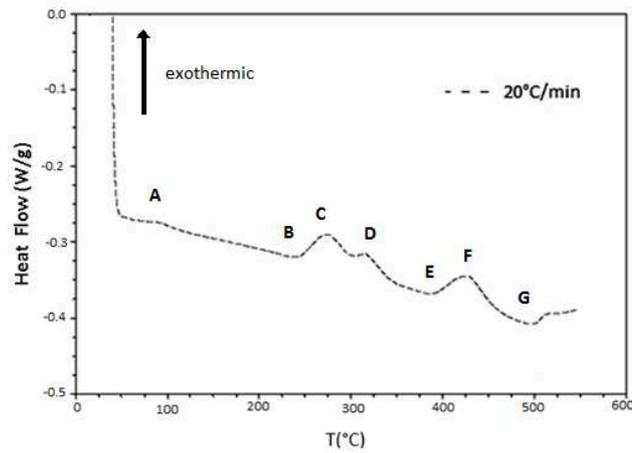
Fig. 1 DSC curves of the Al-Mg-Si alloy homogenized 6 h at 550°C, quenched in water and heated at 20°C/min.
