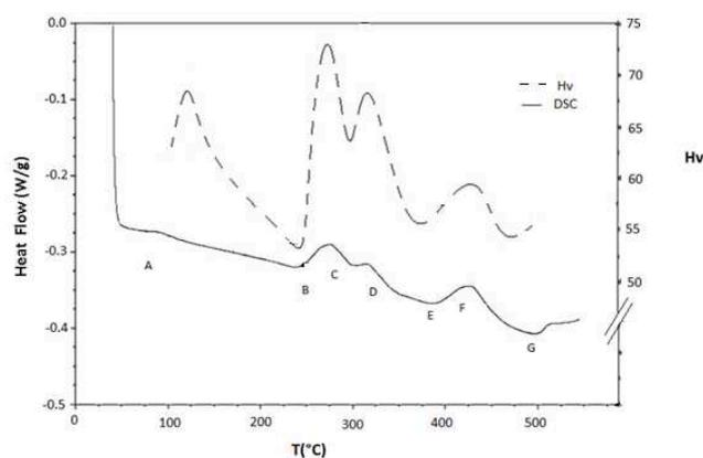
Fig. 4 DSC curve (heating rate 20°C/min) and the corresponding hardness plot for as-quenched Al-Mg-Si alloy.
