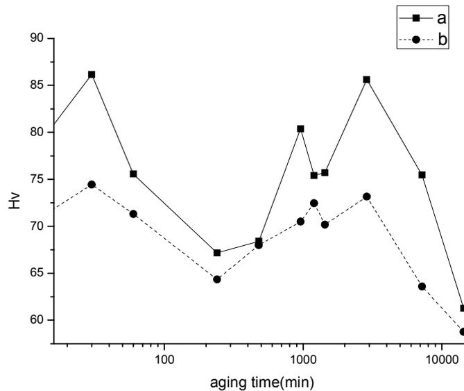
Fig. 5 Hardness variation versus aging time at 150°C of a) quenched Al-Mg-Si alloy and b) natural aged (27 months) Al-Mg-Si alloy.
