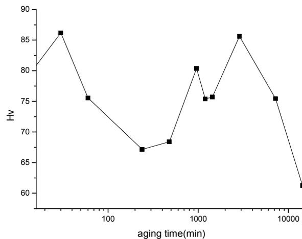
Fig. 3 Hardness variation versus aging time at 150°C of quenched Al-Mg-Si alloy.
