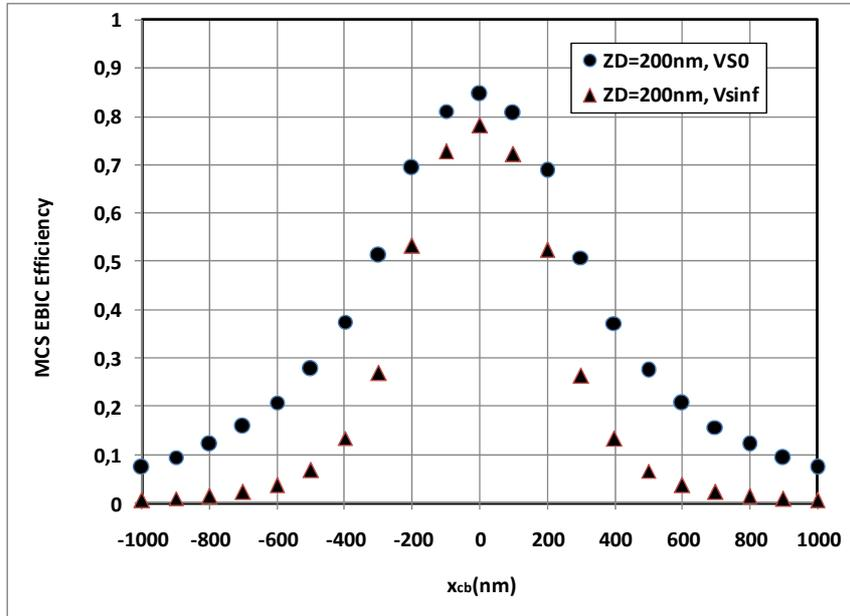
**Figure 3** Variation of the EBIC collection efficiency profiles of a nano Schottky contact of radius  $r_c = 100$  nm in a silicon sample at 5 keV in the case of an infinite surface recombination velocity ( $v_s = \infty$ ) for different values of the depletion region radius  $z_D$  (see online version for colours)
