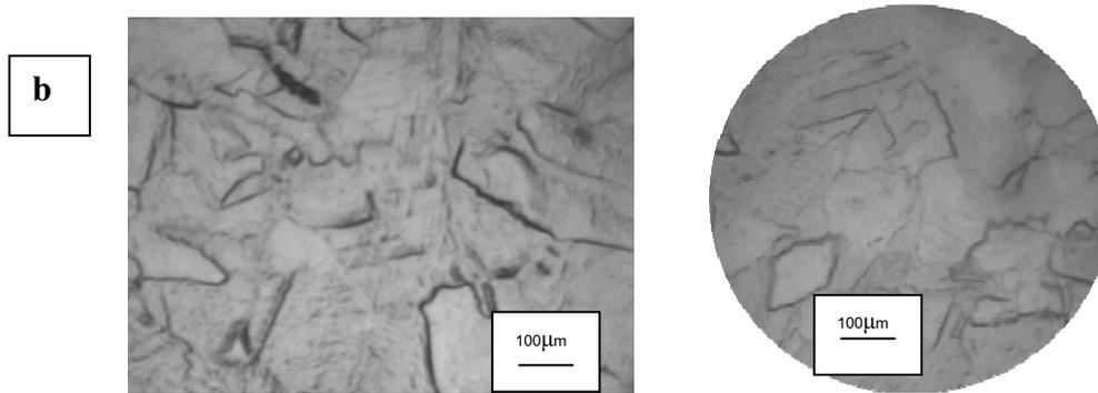
Fig. 1 Microstructural evolution of (a) drawn copper reduced to  $\epsilon=85.94\%$  and (b) followed by an isothermal heat treatment at  $500^{\circ}\text{C}$ .
