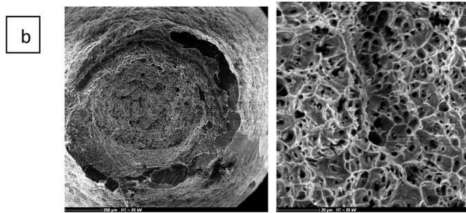
Fig. 5 Fractured surfaces after tensile tests of drawn copper wire (a) un-annealed sample and (b) annealed sample at 500°C for 60 min.
