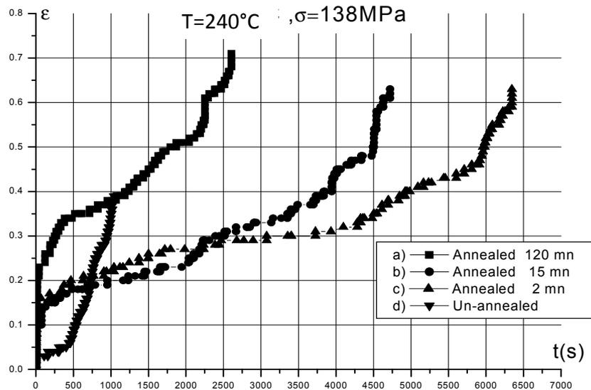
Fig. 2 Creep curves of drawn copper wire at constant temperature and stress.
