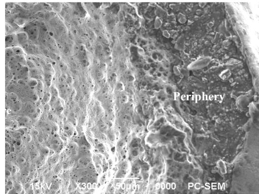
Fig. 3 SEM observation of the cross-section of the fractured drawn copper by creep test.
