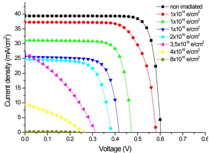
Figure 3. The calculated I-V characteristics of the n+-p-p+ Si solar cell under AM0 for different fluences of 1 MeV electron irradiation taking into account all traps.
