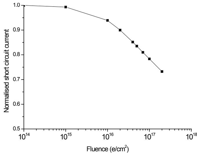
Figure 2. The extracted short circuit current, normalized to the unirradiated value, from the calculated I-V characteristics (Figure 1) of the n+-p-p+ Si solar cell under AM0 for different fluences of 1 MeV electron irradiation taking into account the majority traps and only the shallower minority trap,  $E_C = 0.20$ .
