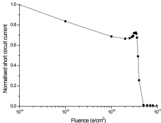
Figure 4. The extracted short circuit current, normalized to the unirradiated value, from the calculated I-V characteristics (Figure 1) of the n+-p-p+ Si solar cell under AM0 for different fluences of 1 MeV electron irradiation taking into account all traps.
