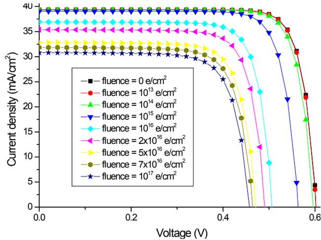
Figure 1. The calculated I-V characteristics of the n+-p-p+ Si solar cell under AM0 for different fluences of 1 MeV electron irradiation taking into account the majority traps and only the shallower minority trap,  $E_C = 0.20$ .
