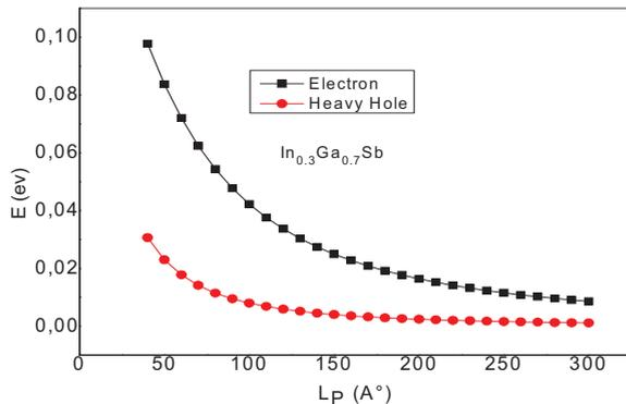
Fig. 1. Variation of Energy quantization as function of well width for ( $n=m=1$ )
