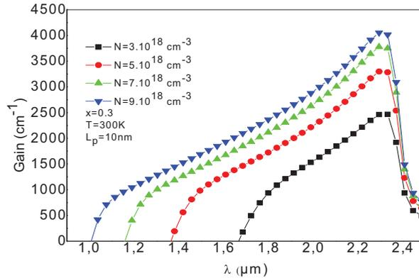
Fig 6: Variation of the gain as a function to wavelength for deferent carrier density
