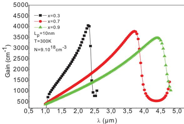
Fig 3. Variation of the gain as a function to wavelength for deferent concentrations of In
