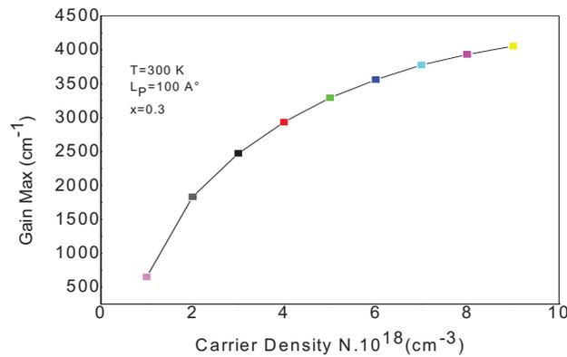
Fig 7. Gain max as a function to carrier density.
