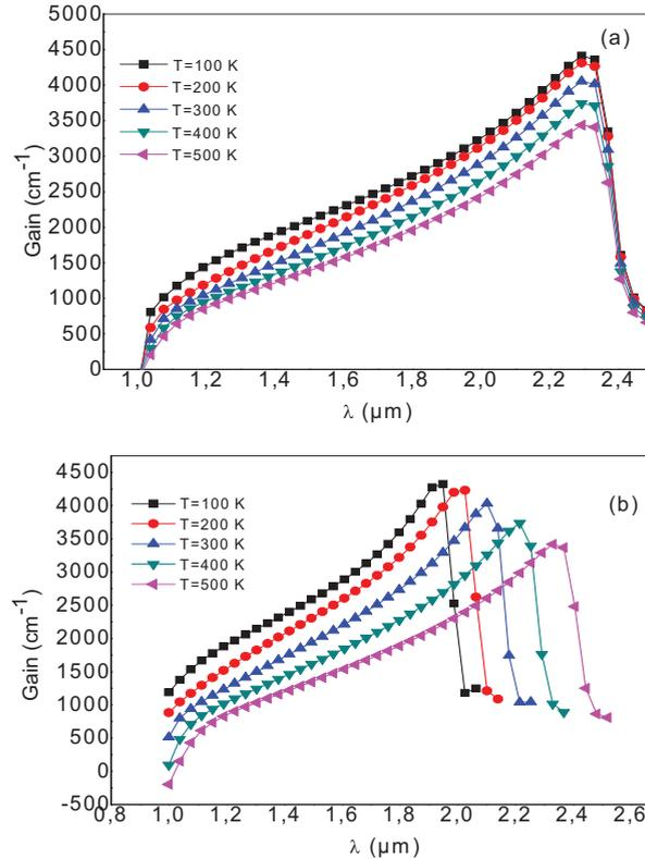
Fig 5. Variation of the gain as a function to wavelength for different temperature with  $N=9.10^{18} \text{ (cm}^{-3}\text{)}$ ,  $x=0.3$ ,  $L_p=10\text{nm}$ .
