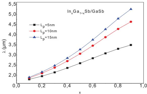
Fig. 2. Wavelengths corresponding to the first transition ( $n=1$ ) between the quantized energy levels of electrons and heavy holes as a function of (In) fraction for  $\text{In}_x\text{Ga}_{1-x}\text{Sb}/\text{GaSb}$  quantum well structure with well widths  $L_p = 5, 10$  and  $15 \text{ nm}$ .
