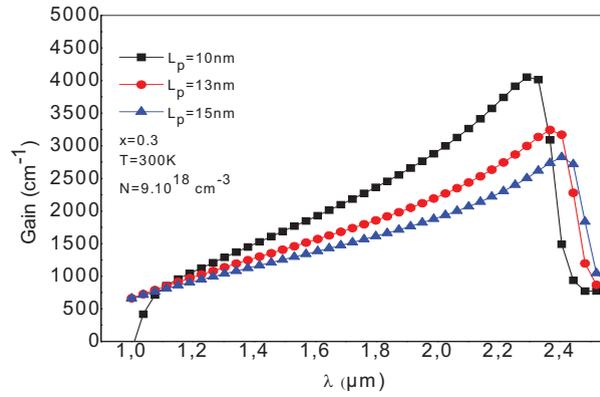
Fig 4. variation of the gain as a function to wavelength for deferent well width.
