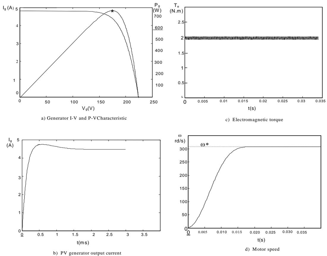
Fig.13: Simulation results for solar insolation  $E=1000W/m^2$
