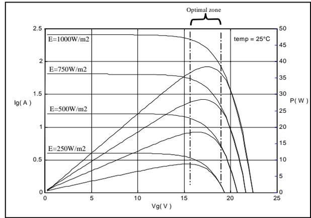
Fig.3 : Photovoltaic module characteristics
