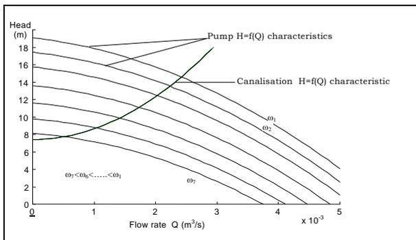
Fig.9 : Multispeed family of pump head capacity curves showing operating points and canalisation characteristic.
