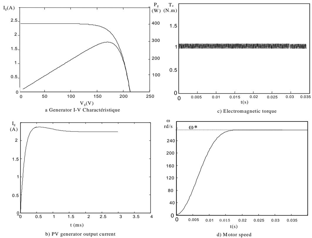
Fig.14: Simulation results for solar insolation  $E=500W/m^2$
