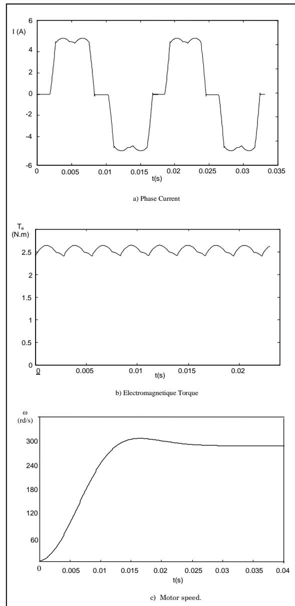
Fig.11: Simulation results without regulation
