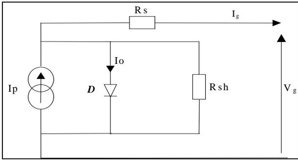
Fig.2 : Equivalent Circuit of the PV generator
