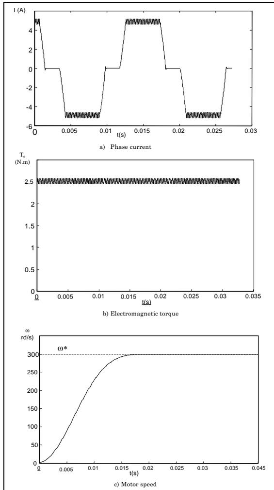
Fig.12: Simulation results with PI speed and hysteresis current controllers regulation
