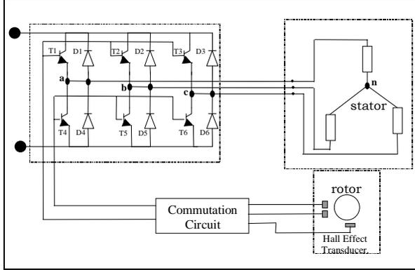
Fig.5 : Brushless PMDC motor and its drive
