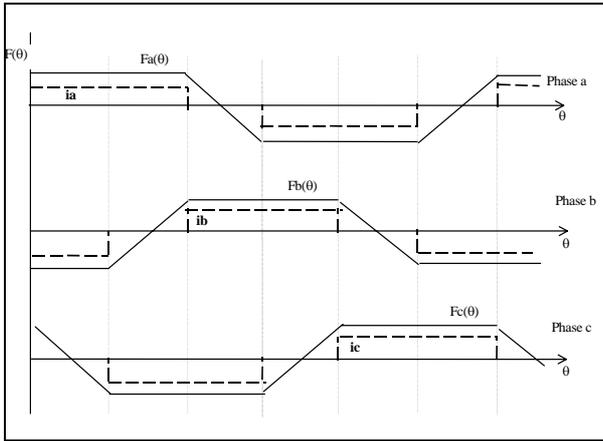
Fig.6 : Back e.m.f and current waveforms
