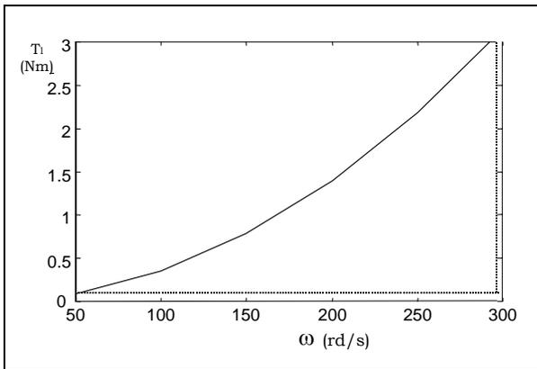
Fig.8: Pump shaft torque versus speed
