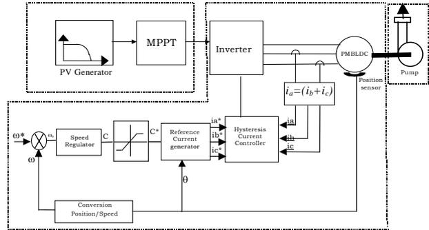
Fig.10: Overall system configuration
