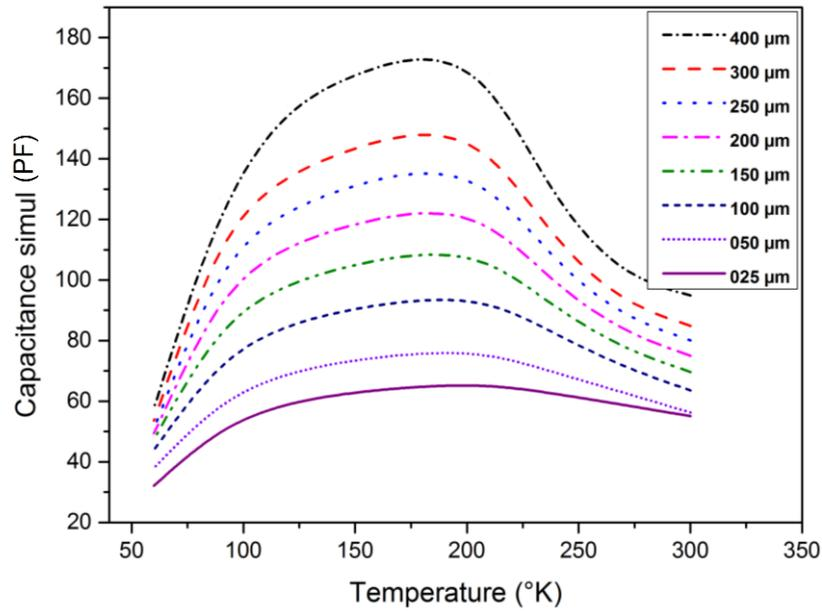
**Figure 5.16: The simulated capacitance-temperature characteristic for different cathode widths.**
