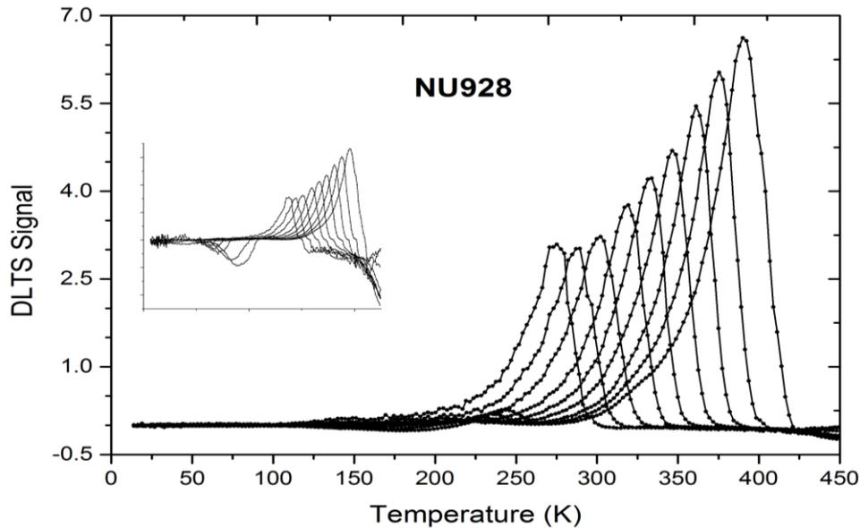
**Figure 5.8: DLTS spectra for the sample (211)A (NU928). In the insert in (b), the positive signal (electron deep levels) is divided by 20.**
