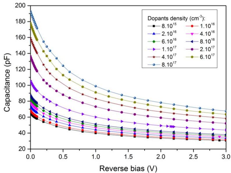
**Figure 5.46: The simulated capacitance voltage of NU928 sample with different dopants densities.**
