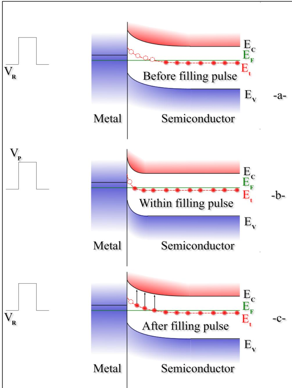
**Figure A.1: Illustration of the band diagram of an n-type Schottky diode under different bias conditions: (a) under reverse bias ( $V = V_R$ ), (b) under filling pulse condition ( $V = V_P$ ) and (c) under reverse bias ( $V = V_R$ ).**
