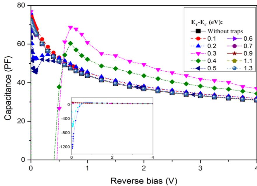
**Figure 5.23: The simulated capacitance-voltage characteristics in present of one acceptor trap at different energy positions.**
