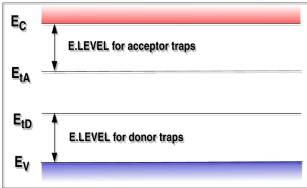
**Figure 4.7: ATLAS definition of the trap energy level for acceptor and donor traps in reference to the conduction and valence band edges.**
