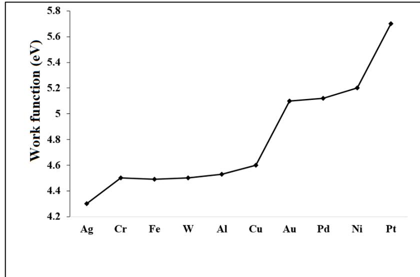
Figure 2-9: The work function of different metals [55].
