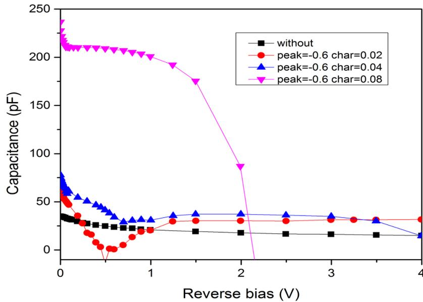
**Figure 5.34: The simulated capacitance-voltage characteristics with traps density decreasing distributions using Gaussian peak at the surface.**
