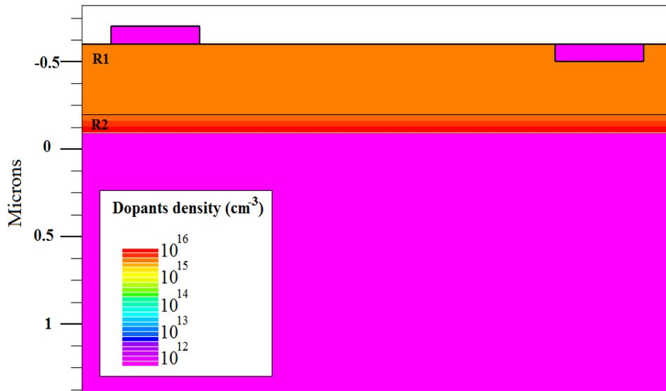
**Figure 5.27: The Acceptor dopant concentration distribution in two different regions (R1 and R2).**
