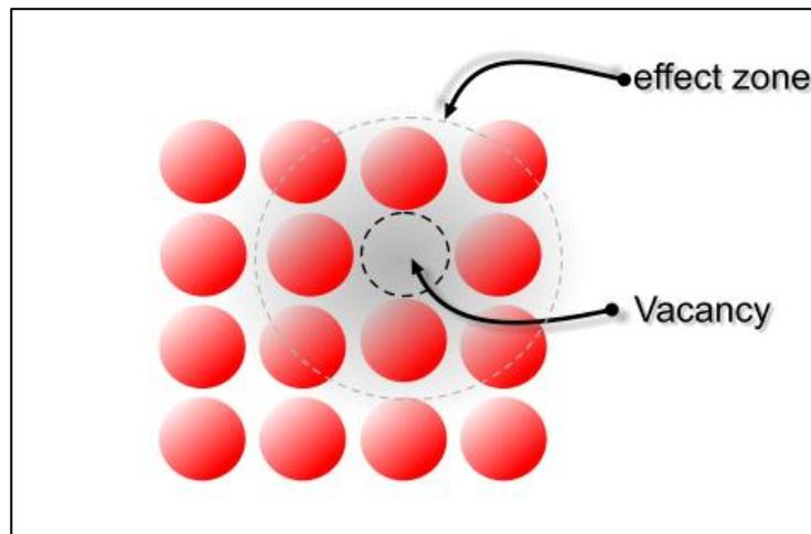
**Figure 3.3: Schematic representation of vacancy defect at the atomic scale**
