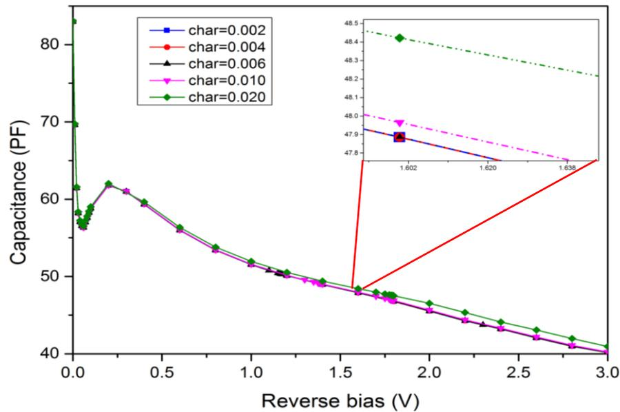
**Figure 5.32: The simulated capacitance-voltage characteristics in presence of dopants density peaks with different characteristic length. The insert is a zoomed C-V in order to clarify the differences.**
