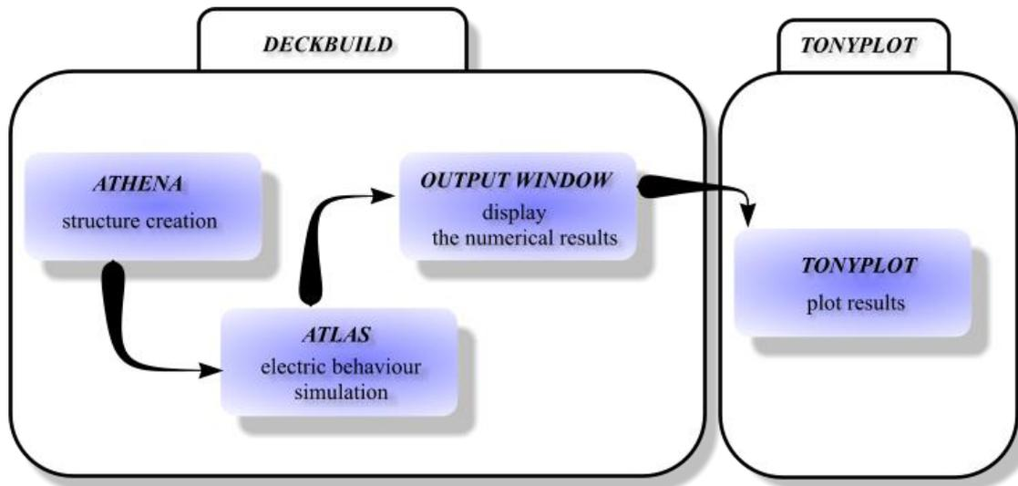
**Figure 4.1: The main modules in SILVACO.**
