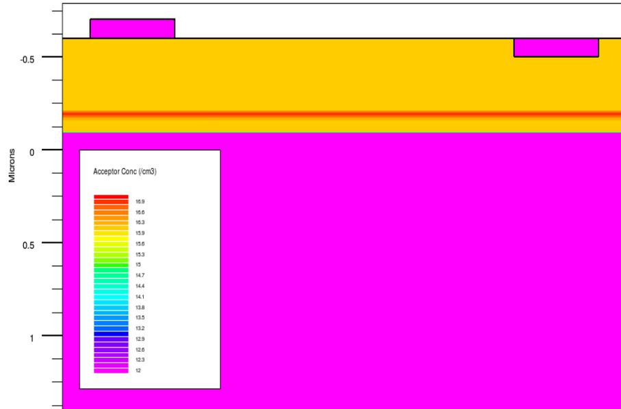
**Figure 5.30: The Acceptor concentration distribution with peak density.**
