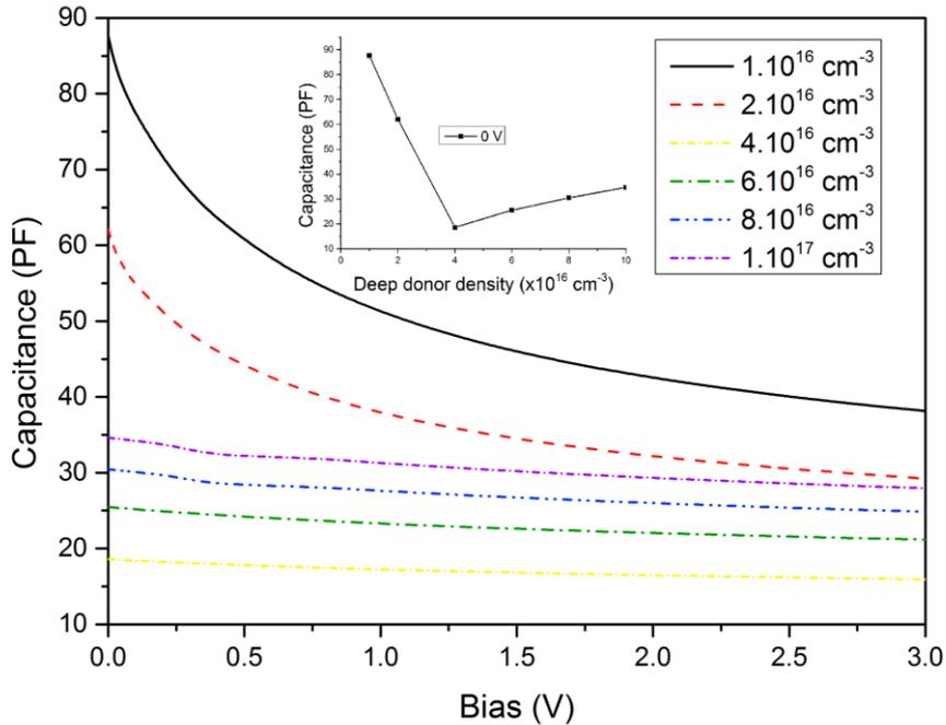
**Figure 5.50: The simulated capacitance-voltage characteristics of the NU928 sample for different densities of the deep donor level “E” The insert is the capacitance for a bias of 0V versus the deep donor density showing the type inversion phenomenon.**
