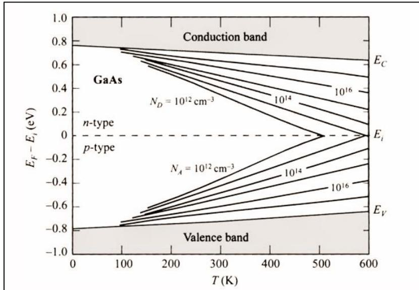
**Figure 2-5: The Fermi level in GaAs with temperature for different doping type and density [1].**
