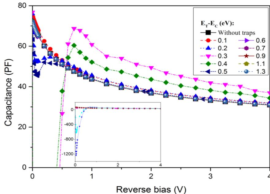
**Figure 5.23: The simulated capacitance-voltage characteristics in present of one acceptor trap at different energy positions.**
