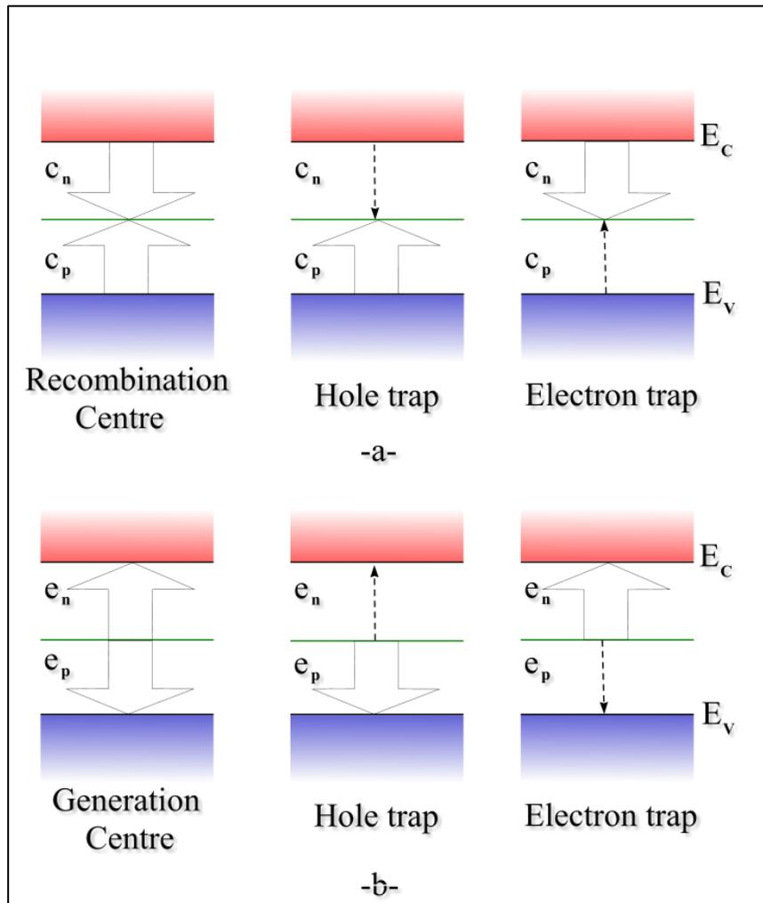
**Figure 3.11: Definition of the terms (electron trap) and (hole trap) and (generation-recombination centre) by means of the relative magnitudes of the capture and emission rates by the width of the arrows. -a- in neutral region, -b- in depletion region.**
