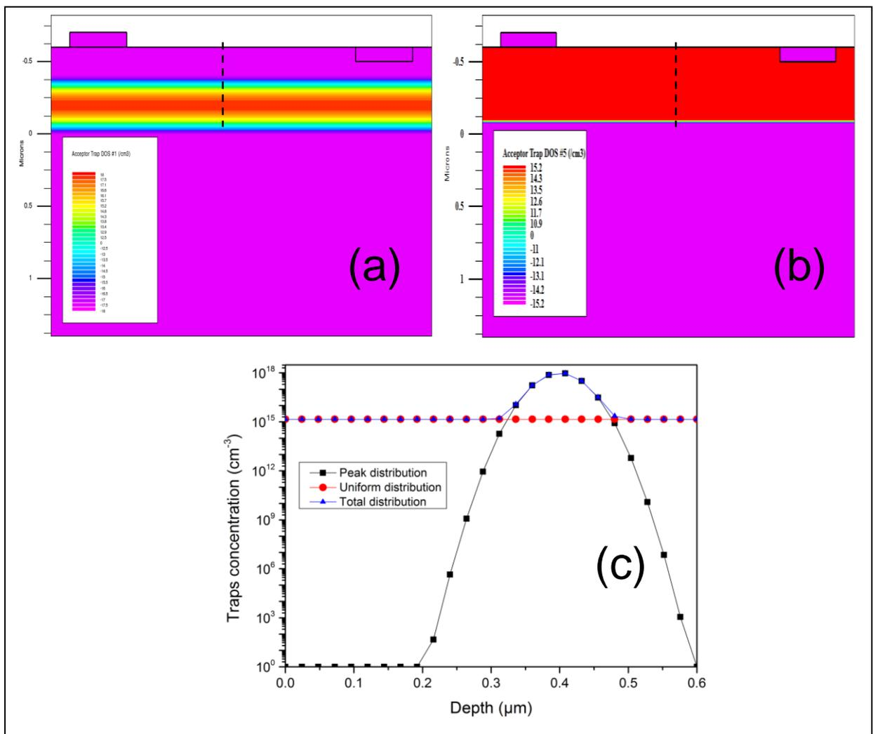
**Figure 5.26:** An example of non-uniform distribution based on Gaussian function used in simulation: a. Gaussian distribution, b. uniform distribution, c. vertical cut (as shown in a. and b. by dashed) shows the profile of both distributions and the total distribution.
