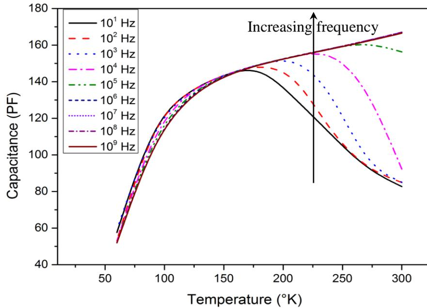
**Figure 5.18: The simulated capacitance–temperature characteristics for different frequencies in the presence of deep acceptors only (311)A sample (NU926).**
