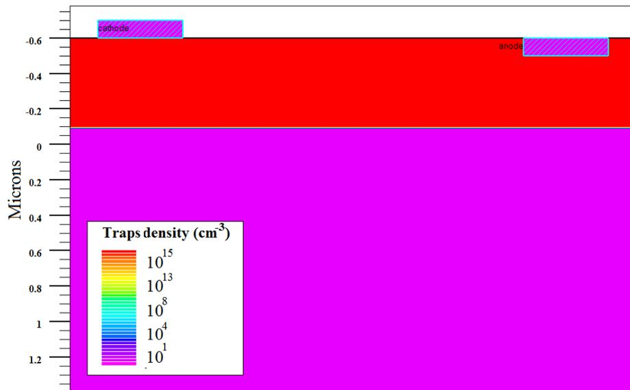
**Figure 5.12:** The deep levels density profile of the simulated device.
