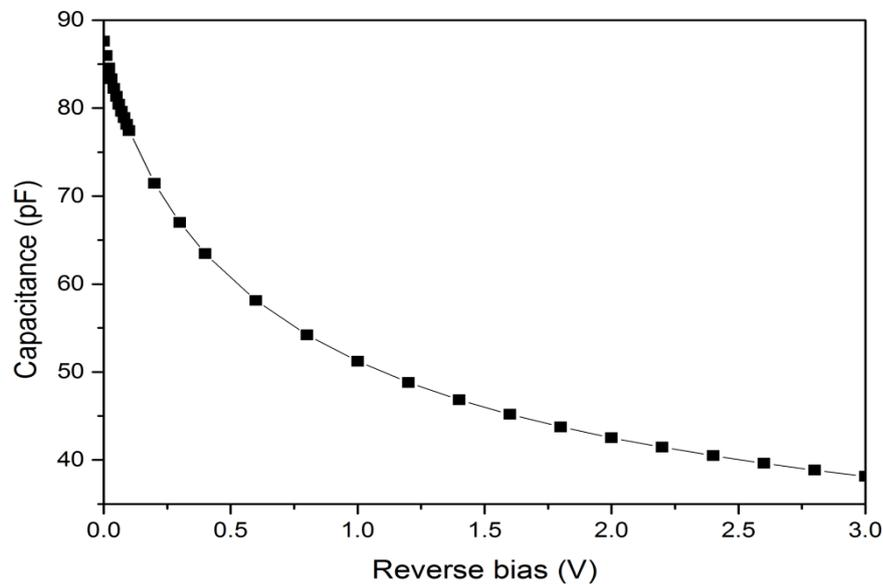
**Figure 5.45: The simulated capacitance voltage of NU928 sample.**
