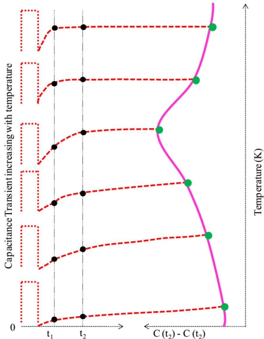
Figure A.3: The generation of DLTS signal from capacitance transient [7].
