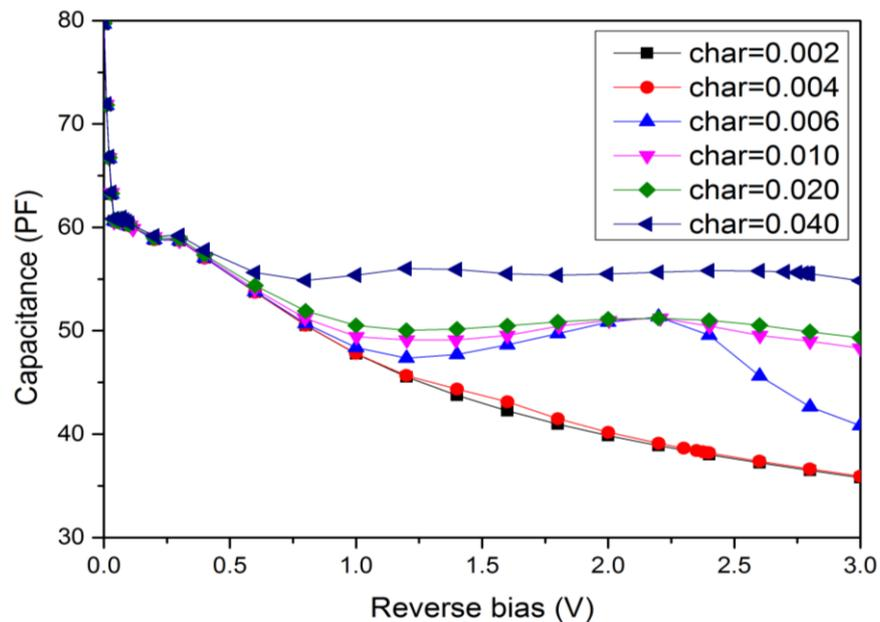
**Figure 5.44:** The simulated capacitance-voltage characteristics of the NU926 sample for different characteristic length of the non-uniformly distributed H3.
