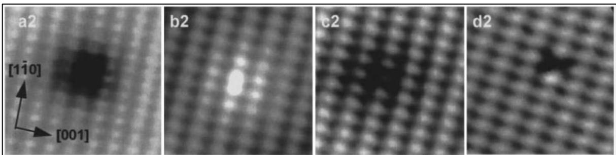
**Figure 3.2:** Images of the major defects in Si-doped GaAs (110) surfaces (a2) show a  $V_{Ga}$ , (b2)  $Si_{Ga}$  donor, (c2)  $Si_{As}$  acceptor, (d2) a  $(Si_{Ga}V_{Ga})$  complex. Adopted from [58].
