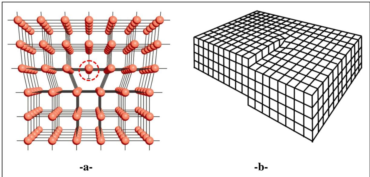
**Figure 3.8: Schematic representation of: -a- Edge dislocation in a cubic crystal [64],
