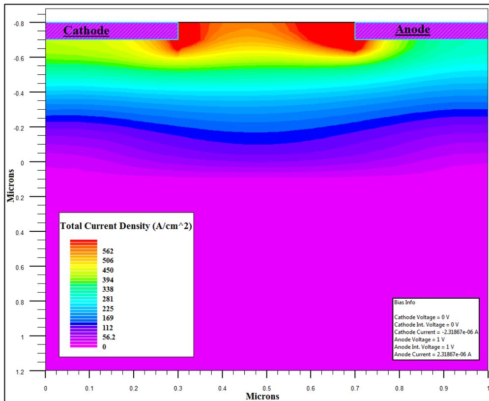
**Figure 4.8: Current density distribution in the device with applied bias equal to 1V.**
