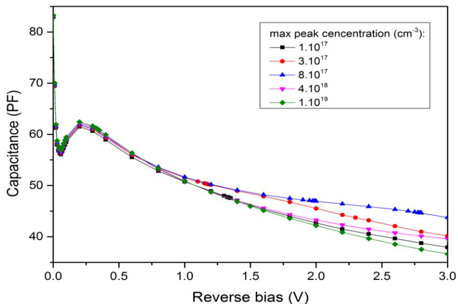
**Figure 5.31: The simulated capacitance-voltage characteristics in presence of dopants density peaks with different densities.**
