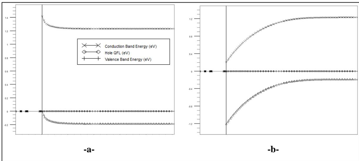
**Figure 4.6: Energy band diagram simulated by SILVACO. a- Ohmic contact. b- Schottky contact.**
