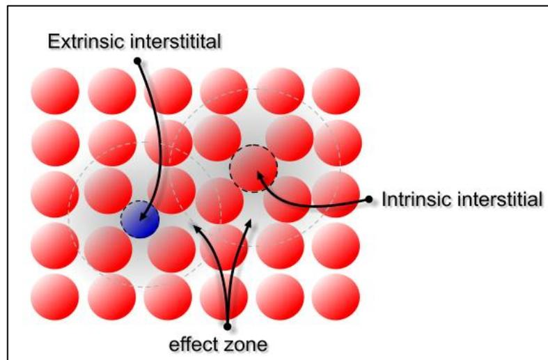
**Figure 3.4: Different types of interstitial defects at the atomic scale.**
