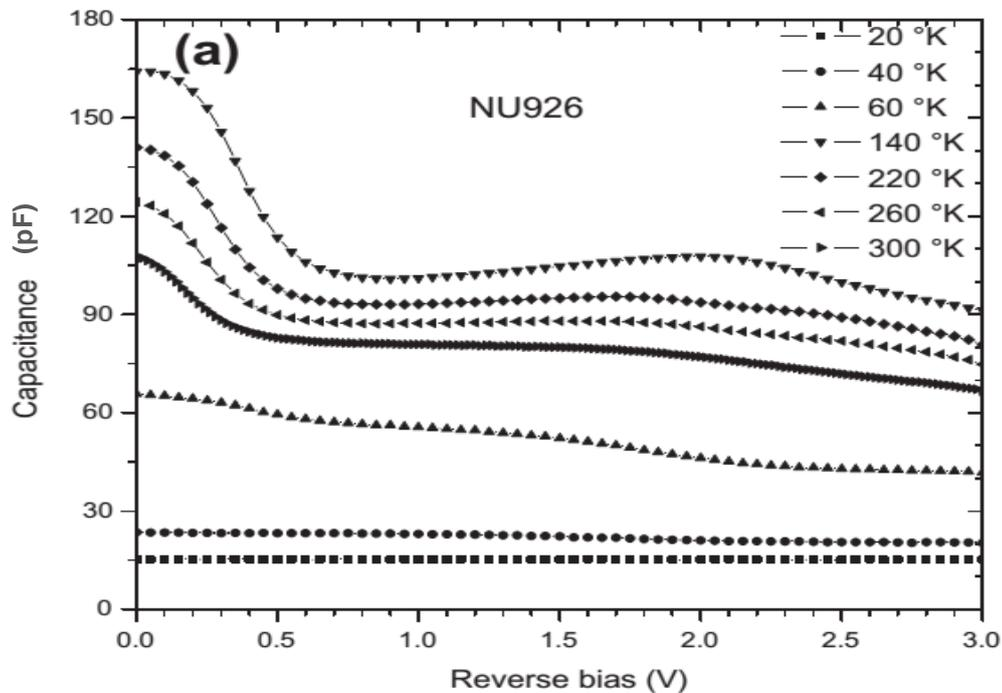
**Figure 5.2:** The capacitance–voltage characteristics at different temperatures for the NU926 sample.
