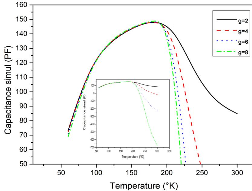
**Figure 5.15: The capacitance temperature characteristic in presence of deep acceptor traps with different degeneracy factor values. The insert is an extended capacitance scale.**
