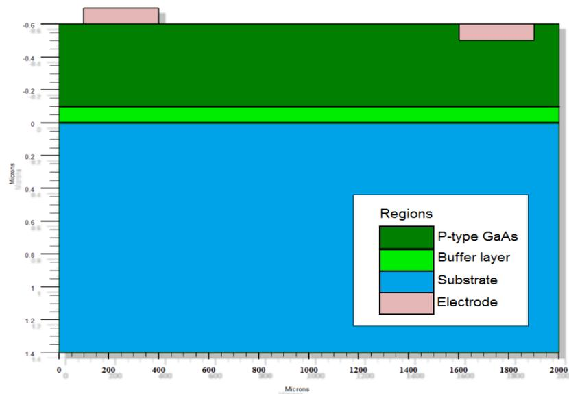
**Figure 5.10:** The different regions of the simulated structure.
