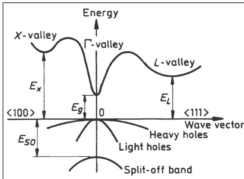
**Figure 2-8: Band structure of GaAs at 300°K [46].**
