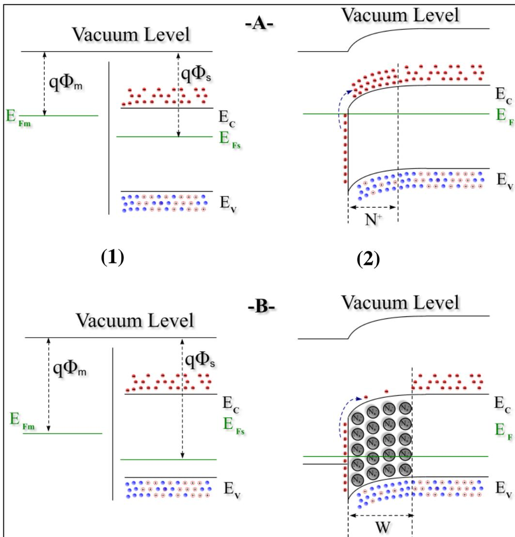
Figure 2-12: Metal-semiconductor band diagram before and after contact (1 and 2 respectively) when  $\Phi_m < \Phi_s$ : A- N-type semiconductor, B- P-type semiconductor.
