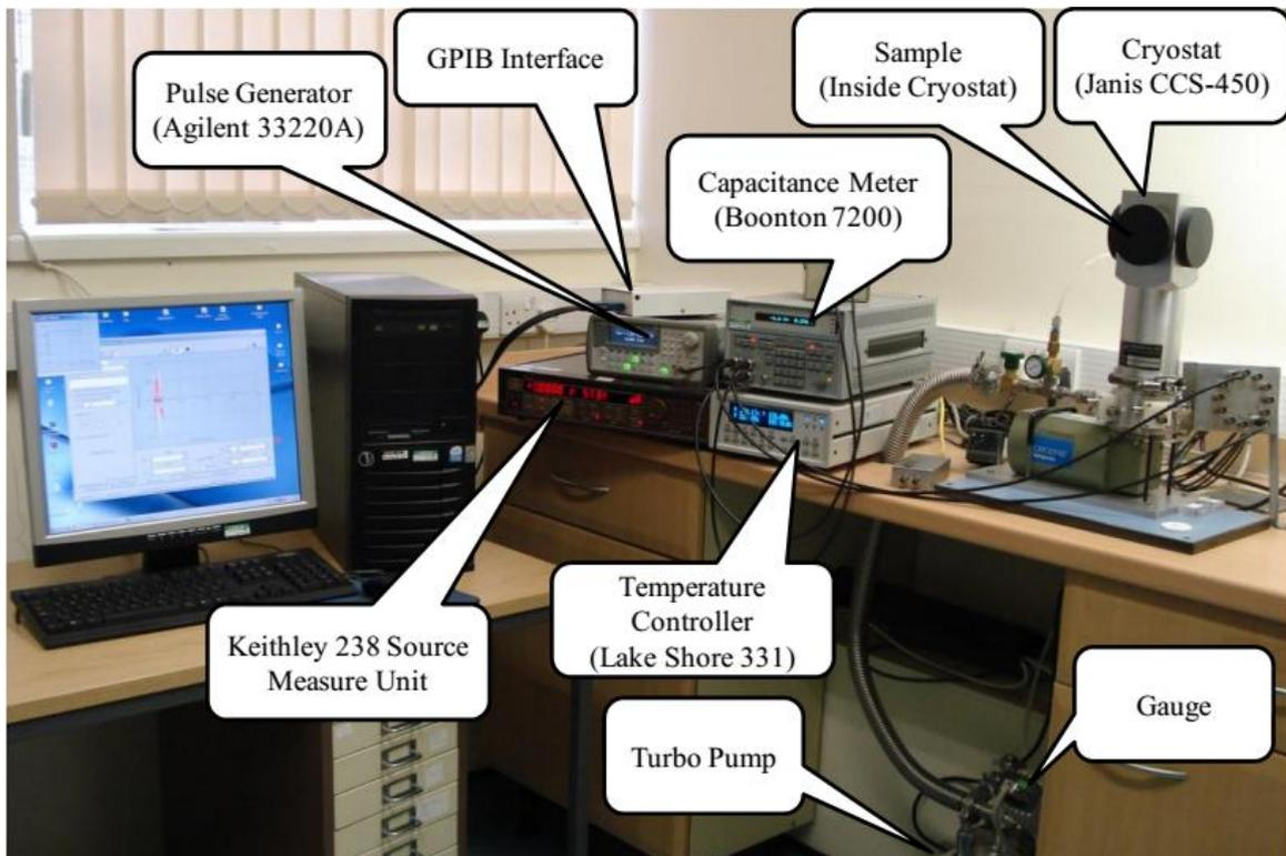
**Figure 5.6: A photograph of the DLTS system at Nottingham University [76].**
