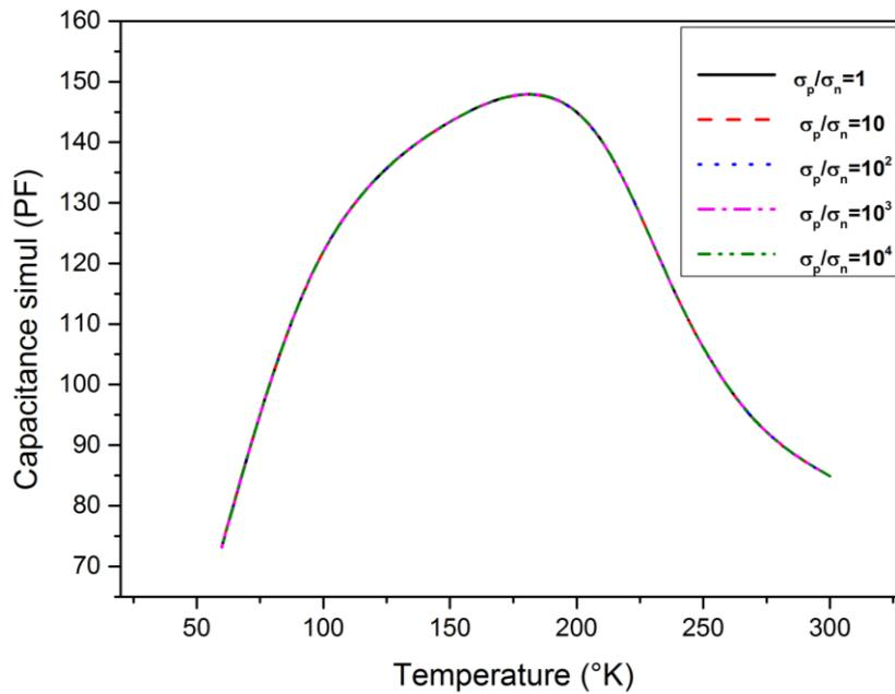
**Figure 5.14: The simulated capacitance temperature characteristic in presence of deep acceptor traps with different electrons capture cross section values.**
