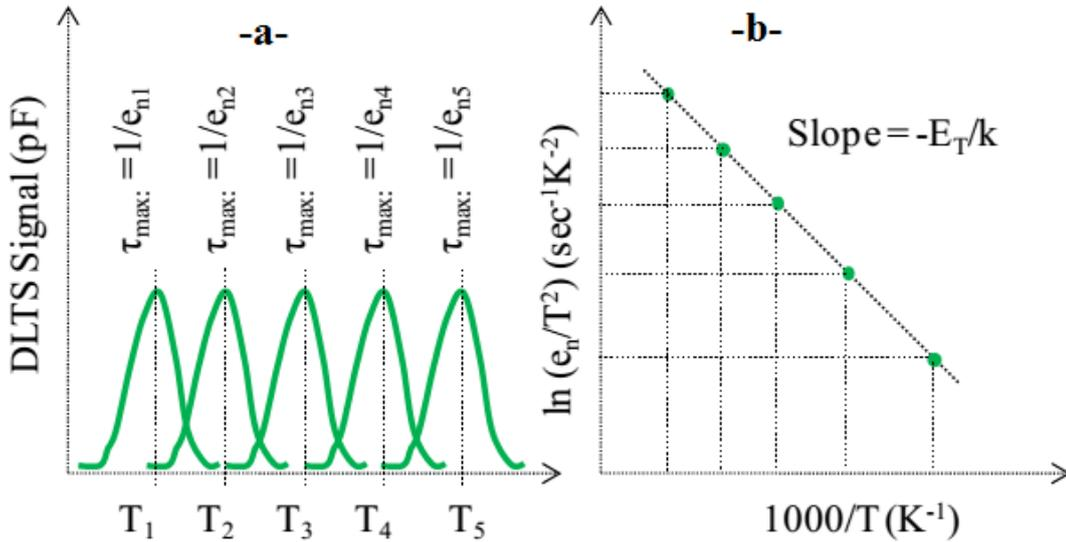
**Figure A.4: a. the change in peak position for different rate windows, b. the Arrhenius plot for the calculation of trap activation energy ( $E_t$ ) [7].**
