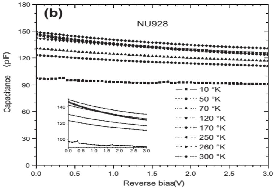
**Figure 5.3: The capacitance–voltage characteristics at different temperatures for the NU928 sample.**
