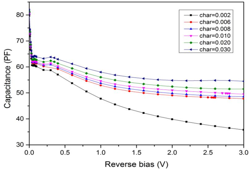
**Figure 5.36: The simulated Capacitance voltage in present of traps peak density with different characteristic lengths.**
