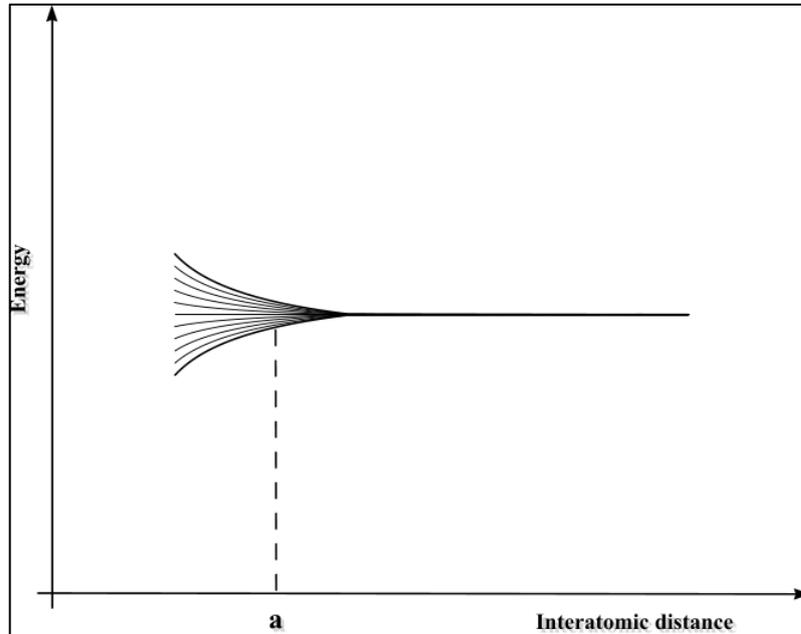
**Figure 2-1: Orbit splitting when several atoms come close to each other.**
