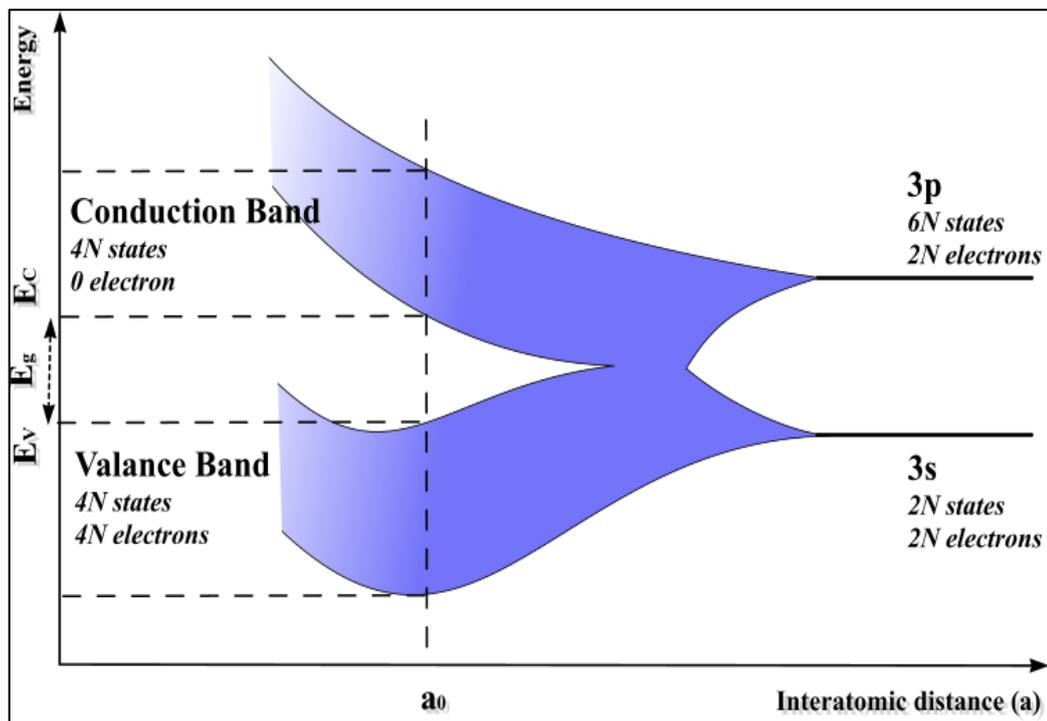
Figure 2-2: Formation of the energy band structure.
