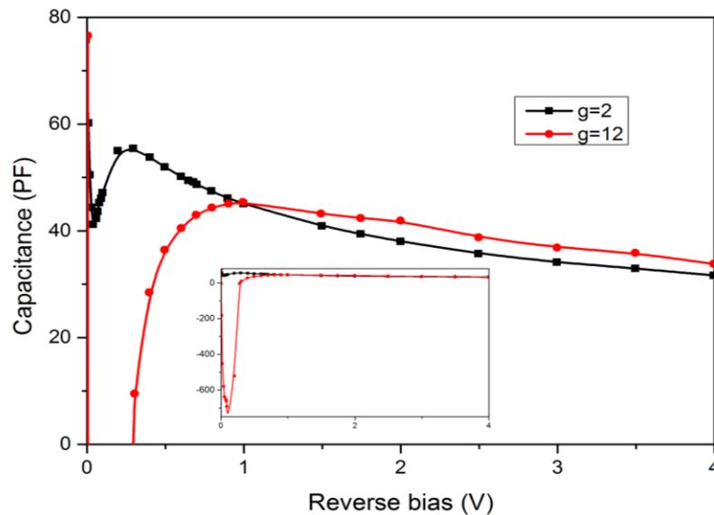
Figure 5.21: The simulated capacitance-voltage characteristics of NU926 sample for different degeneracy factor.
