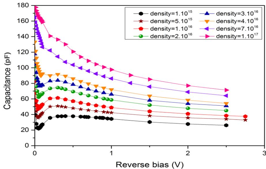
**Figure 5.24: The simulated capacitance-voltage characteristics with different dopants densities.**
