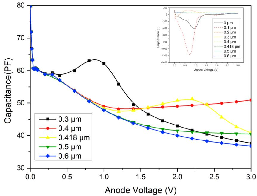
**Figure 5.43:** The simulated capacitance-voltage characteristics of the NU926 sample for different positions of the non-uniformly distributed H3 from the surface. The insert is for other positions for which a negative capacitance appears.
