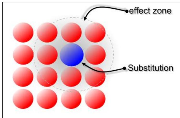
**Figure 3.5: Representation of substitution defect at the atomic scale**
