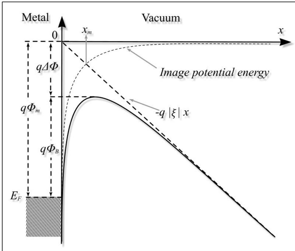
Figure 2-14: Energy-band diagram between a metal surface and a vacuum.
