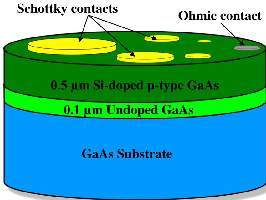
**Figure 5.1:** Schematic representation of the grown structures.
