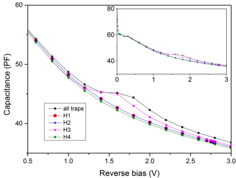
**Figure 5.39:** The simulated Capacitance voltage in presence of every trap peak alone.
