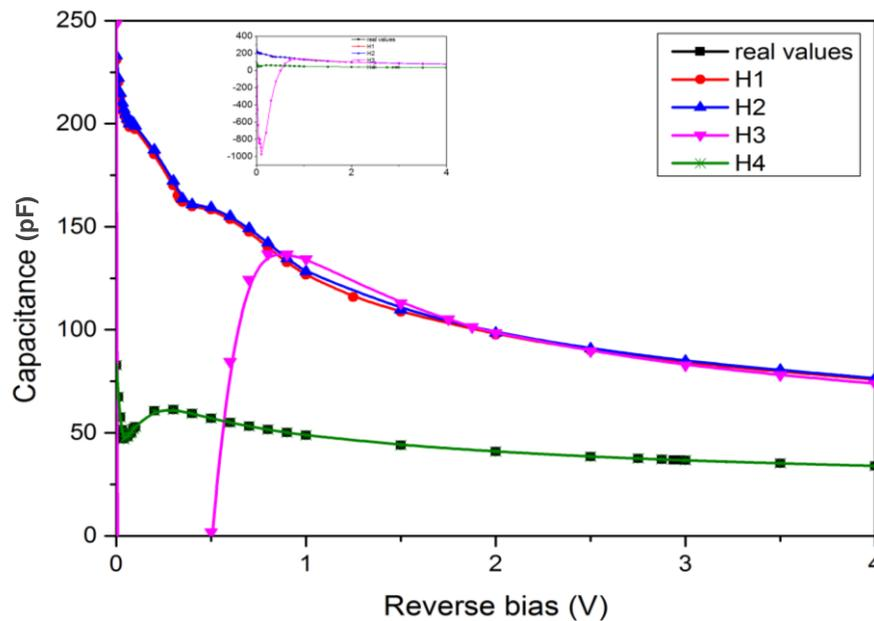
**Figure 5.22: The simulated capacitance-voltage characteristics of NU926 sample: real density values of all levels (squares), high density of: H1 (circles), H2 (up triangles), H3 (down triangles) and H4 (stars).**
