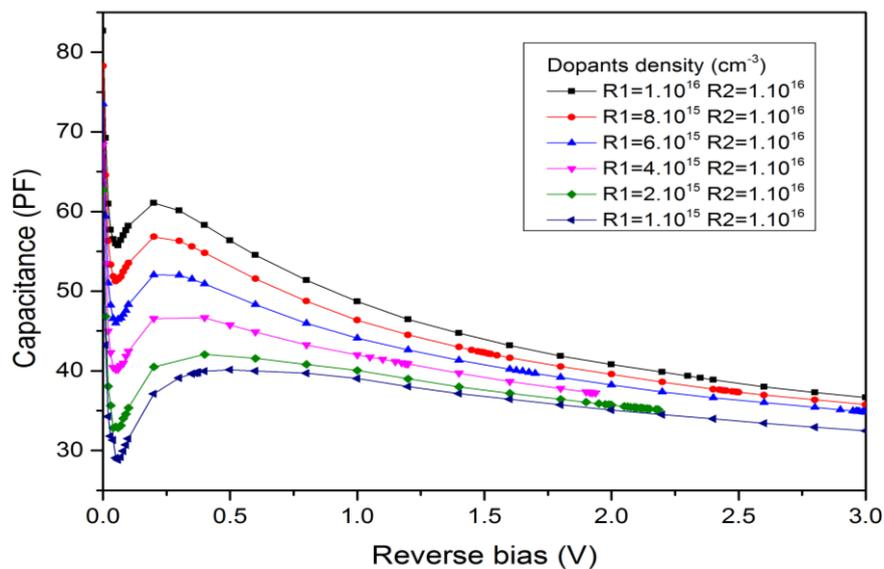
**Figure 5.28: The simulated C-V characteristics with different dopants densities in the first region (R1).**
