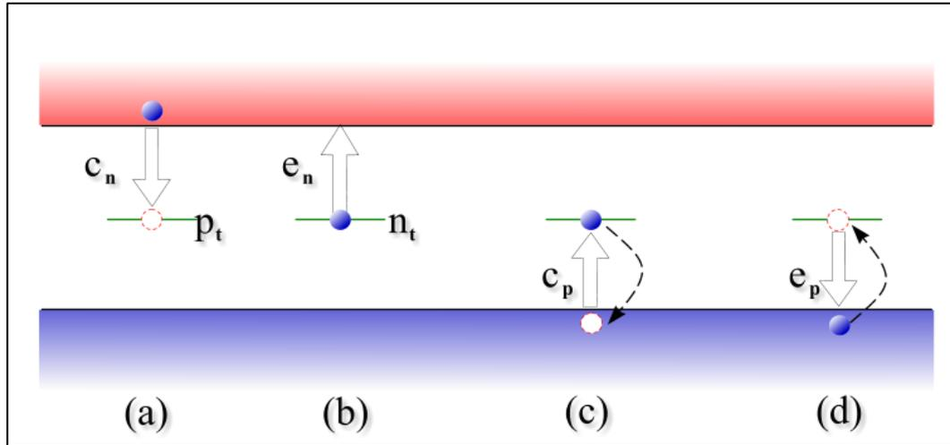
**Figure 3.12: The four carriers' transition processes. a- electron capture, b- electron emission, c- hole capture and d- hole emission.**
