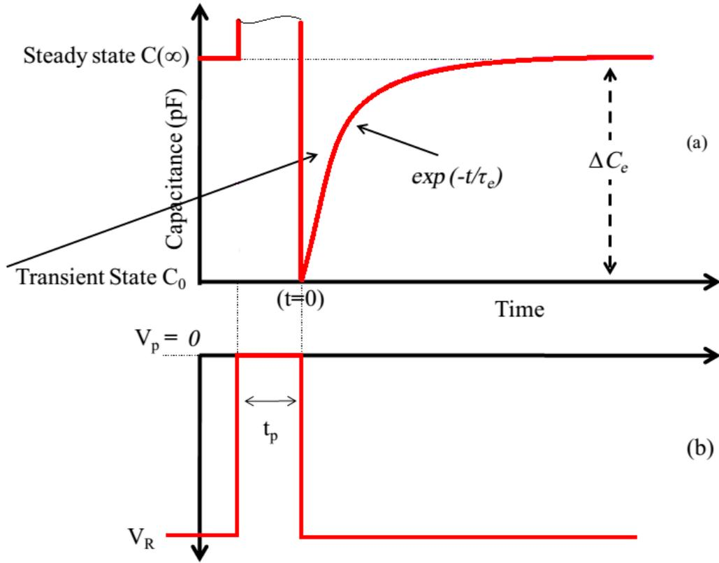
**Figure A.2: (a) Capacitance transient response of the Schottky diode for different bias conditions shown in (b).**
