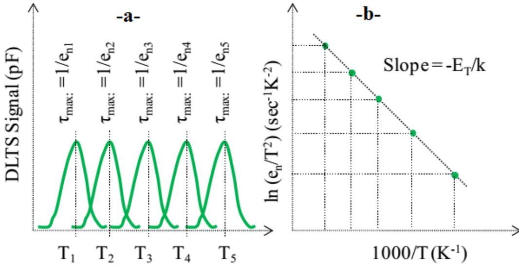
**Figure A.4: a. the change in peak position for different rate windows, b. the Arrhenius plot for the calculation of trap activation energy ( $E_t$ ) [7].**
