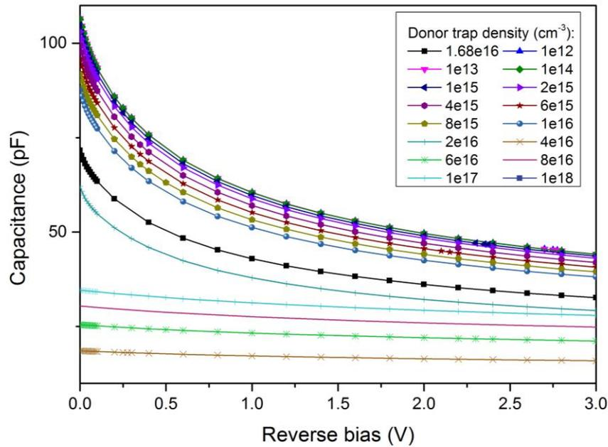
**Figure 5.47: The simulated capacitance voltage of NU928 sample with different donor traps densities.**
