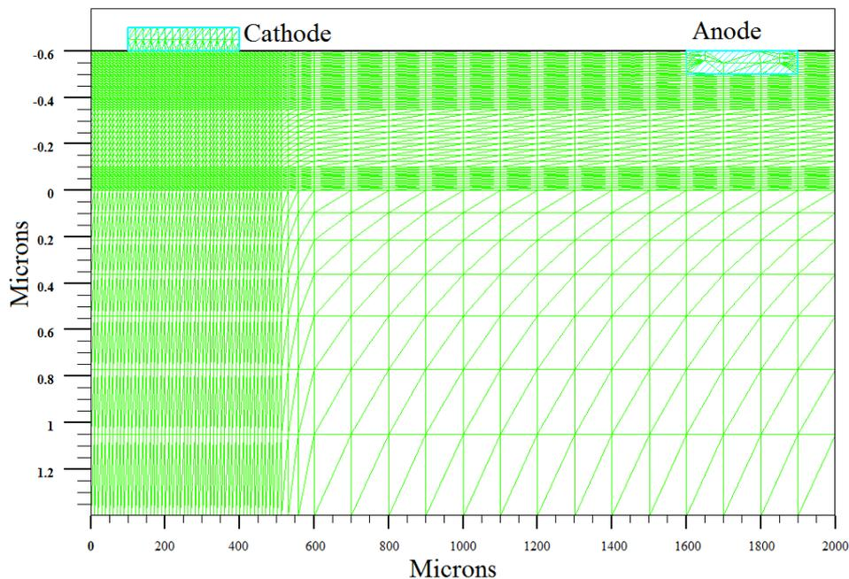
**Figure 5.9: The mesh grid used in the structure simulation.**
