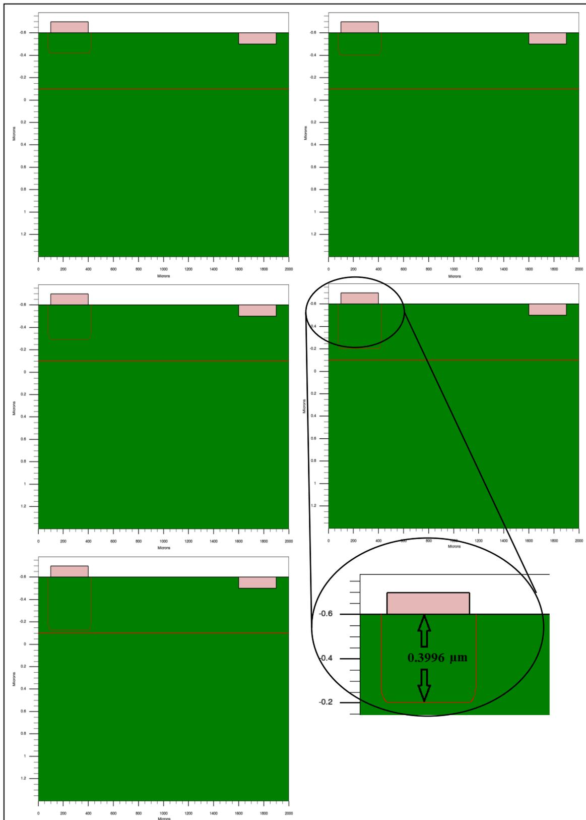
**Figure 5.25: The expansion of the depletion region of the sample NU926 for different biases.**
