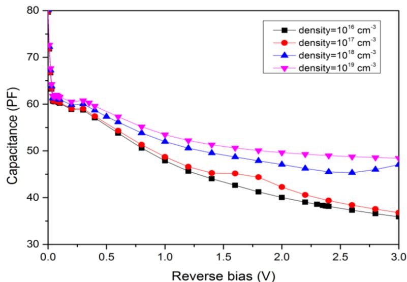
**Figure 5.38: The simulated Capacitance voltage in present of traps peak with different concentrations.**
