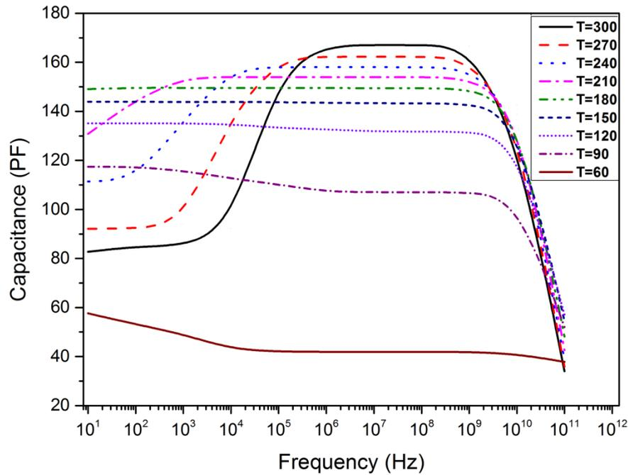
**Figure 5.19: The simulated capacitance–frequency characteristics for different temperatures in the presence of deep acceptors only, (311)A sample (NU926)**
