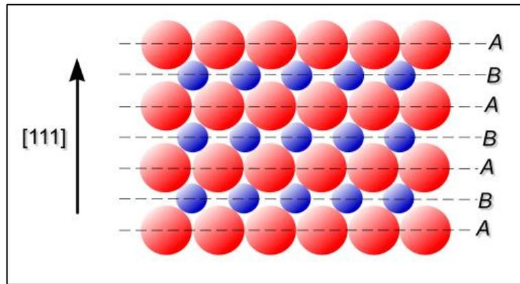
**Figure 2-7: Schematic representation of gallium-arsenide structure shows the difference between (111B) and (111A) planes (-A- and -B-respectively).**
