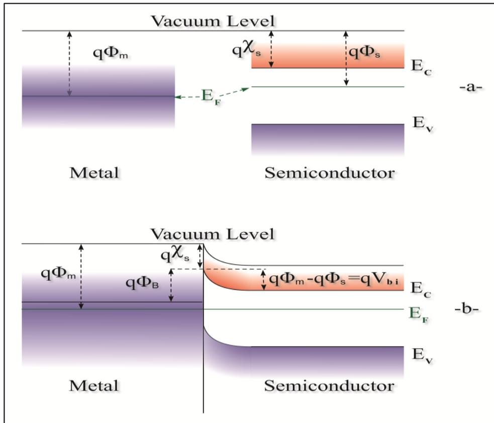
**Figure 2-10: The band diagram of metal and semiconductor: (a) before contact and (b) after contact.**
