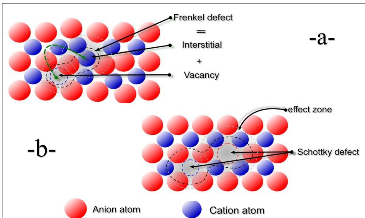
**Figure 3.7: Schematic representation defect clusters in compound materials.**
