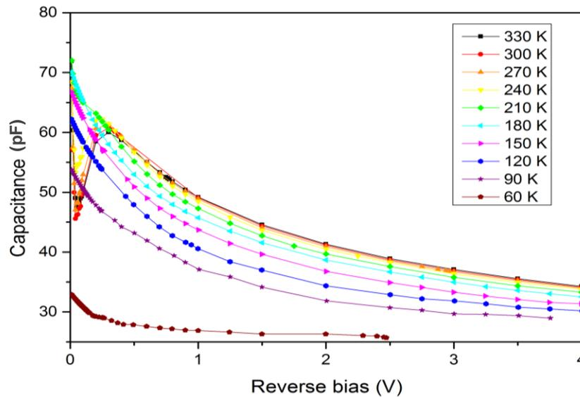
Figure 5.20: The simulated capacitance-voltage characteristics for the NU926 sample.
