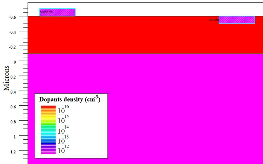
**Figure 5.11:** The acceptors dopant density profile of the simulated device.
