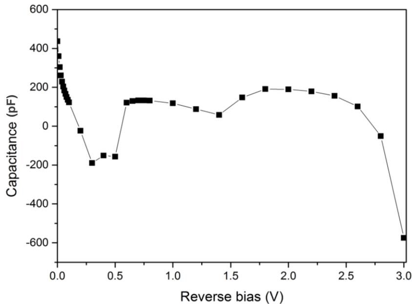
**Figure 5.40: The simulated capacitance-voltage characteristics of the NU926 sample for gradient trap (H3) distribution from top to bottom.**
