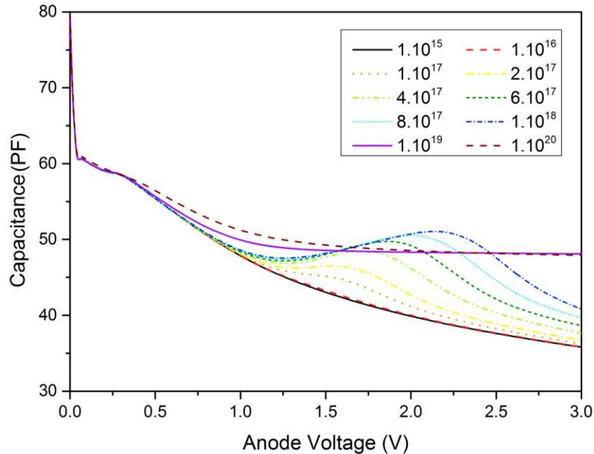
**Figure 5.41: The simulated capacitance-voltage characteristics of the NU926 sample for different densities of the non-uniformly distributed H3. Other levels are kept uniform.**
