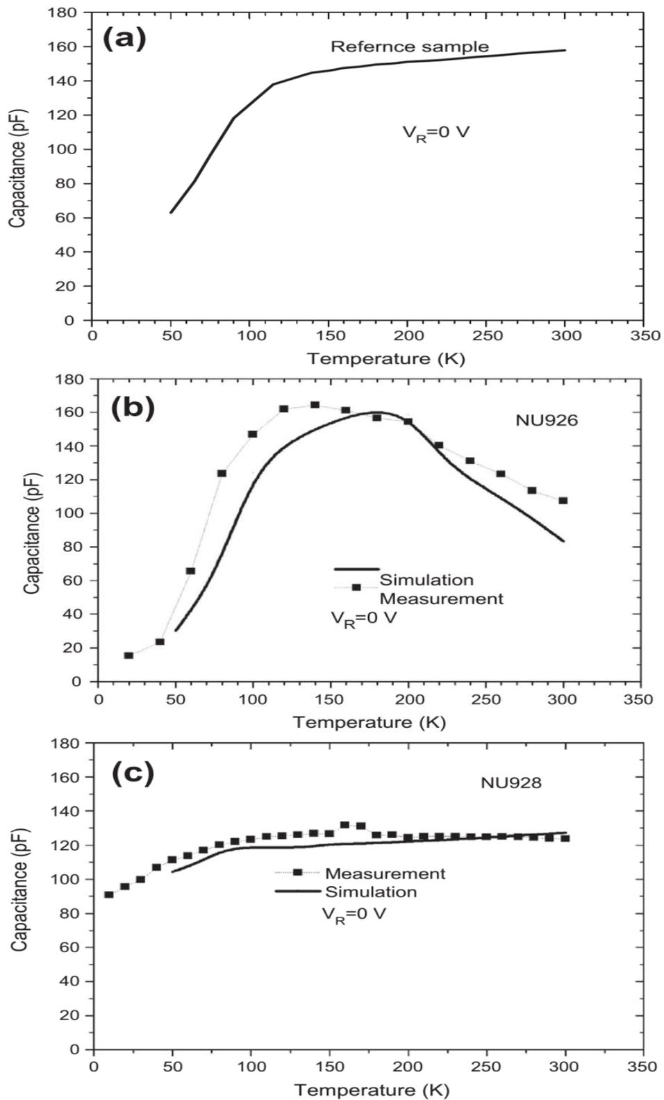
**Figure 5.17: The simulated capacitance–temperature characteristics for three samples: in the absence of deep levels [(a), reference sample], in the presence of deep acceptors [(b) (311)A sample (NU926)] and in the presence of deep acceptors and donors [(c), (211)A sample (NU928)].**
