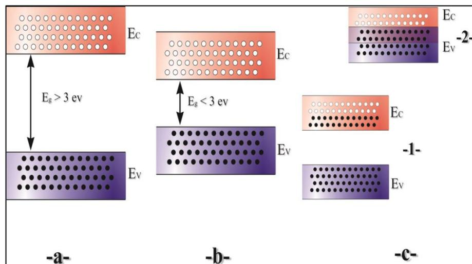
Figure 2-3: Energy band structure for different type of material: a- insulators, b- semiconductors, c- conductors.
