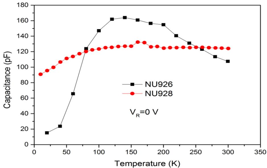
**Figure 5.4: The capacitance–Temperature characteristics at fixed bias ( $V=0$ ) for the samples (311)A (NU926) and (211)A (NU928).**
