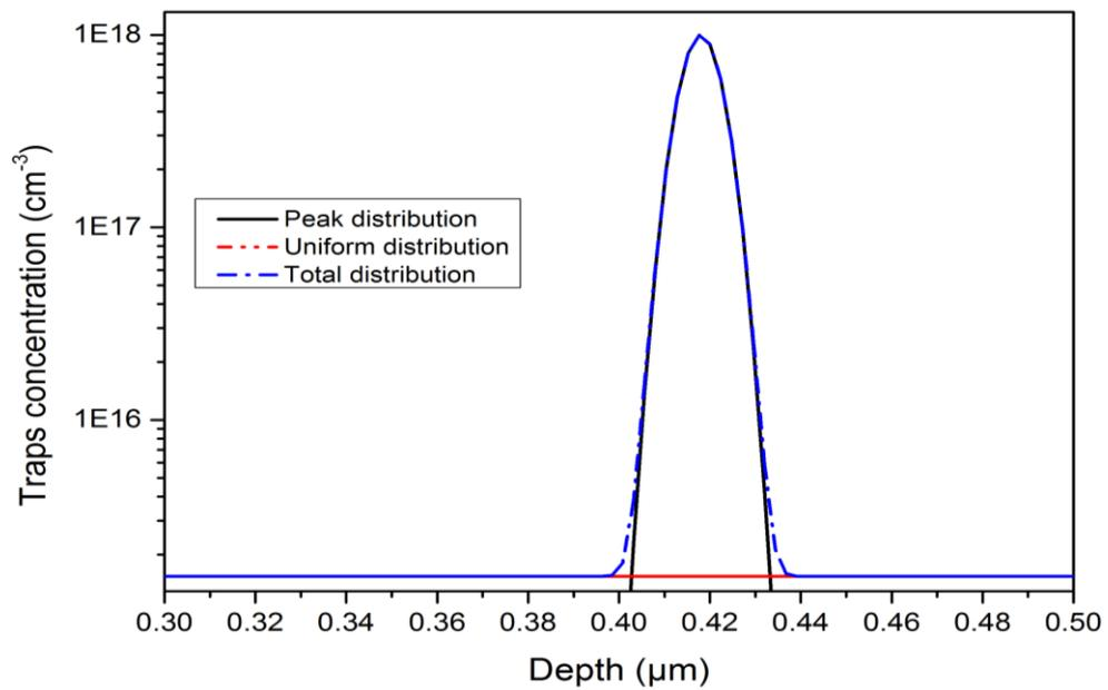
Figure 5.52: The peak's profile of traps high density used in simulation.
