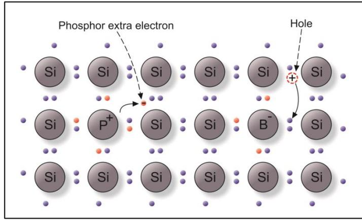
**Figure 2-4: The process of capture and release of electrons by impurity atoms when silicon is doped with boron or phosphor respectively.**
