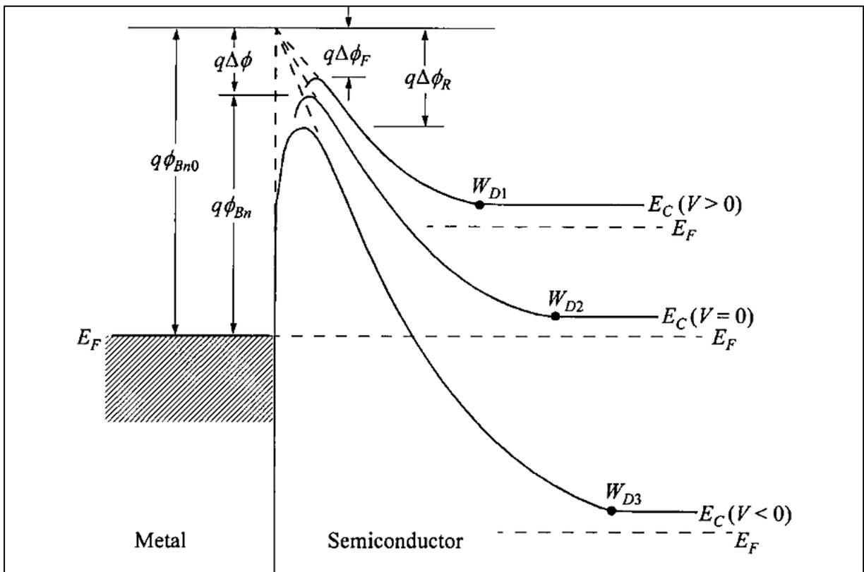
**Figure 2-15: Energy-band diagram incorporating the Schottky effect for a metal n-type semiconductor contact under different biasing conditions. The intrinsic barrier height is  $q\phi_{Bn0}$ . The barrier height at thermal equilibrium is  $q\phi_{Bn}$ . The barrier lowering under forward and reverse bias are  $\Delta\phi_F$  and  $\Delta\phi_R$  respectively.**
