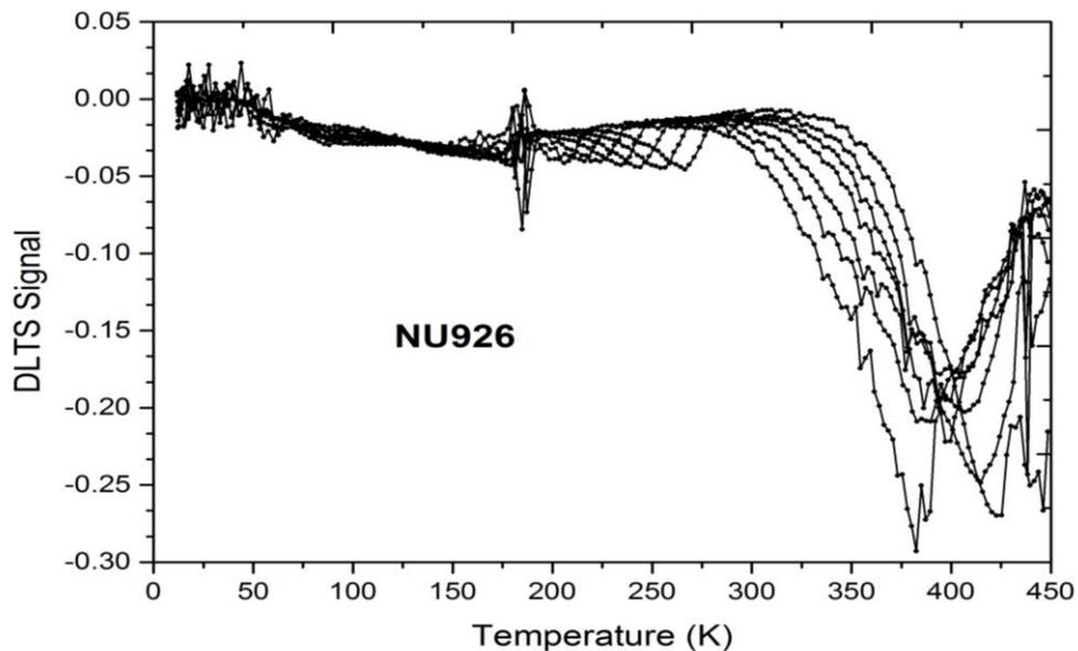
**Figure 5.7: DLTS spectra for the sample (311)A (NU926).**
