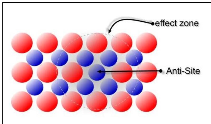
**Figure 3.6: Representation of Anti-site defect at the atomic scale in compound materials.**
