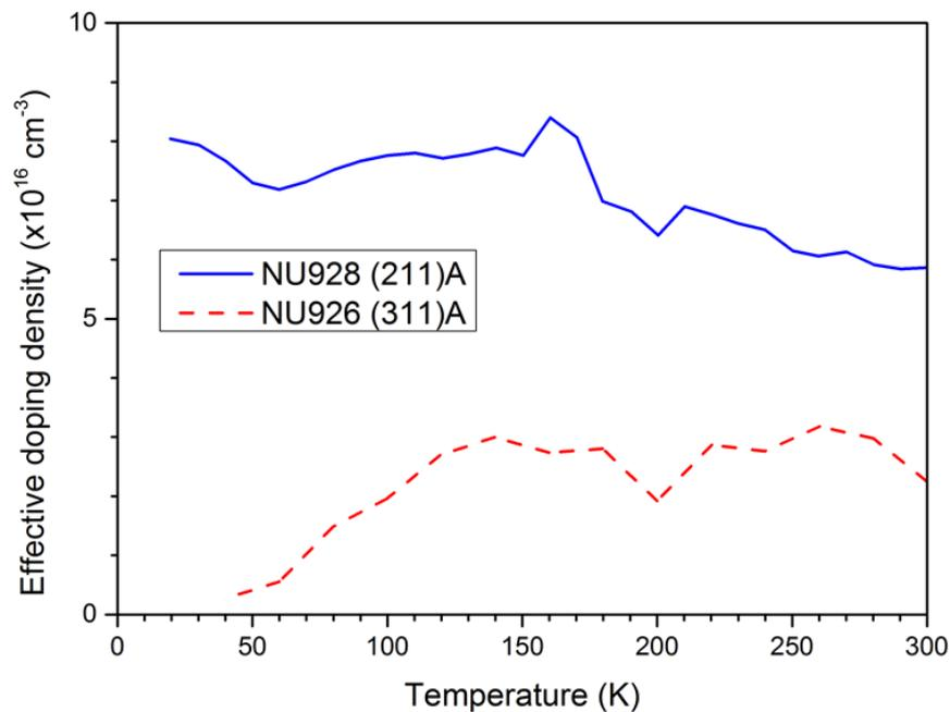
**Figure 5.5: The average effective density evaluated from the C–V characteristics of the (211)A and (311)A samples at different temperatures.**
