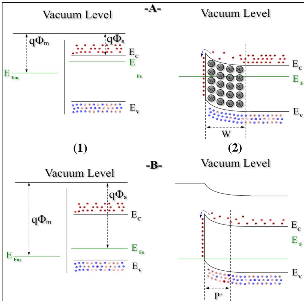
**Figure 2-11 Metal-semiconductor band diagram before and after contact (1 and 2 respectively) when  $\Phi_m > \Phi_s$ : A- N-type semiconductor, B- P-type semiconductor.**
