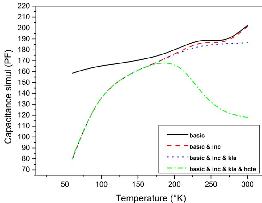
**Figure 5.13: The simulated capacitance-temperature characteristic using different models.**
