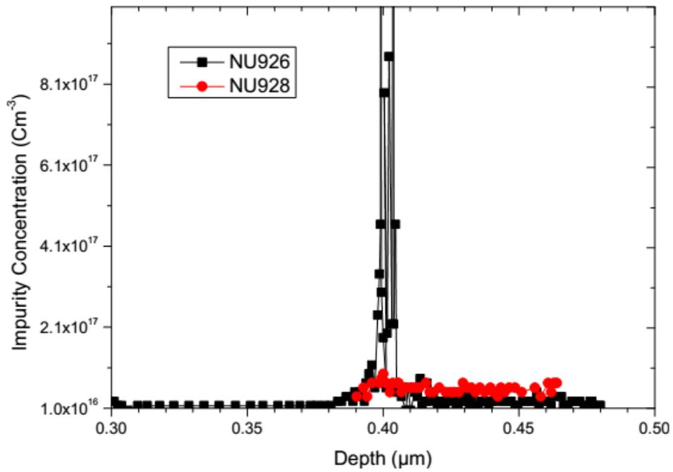
Figure 5.51: The effective doping density profile evaluated from the C-V characteristics.
