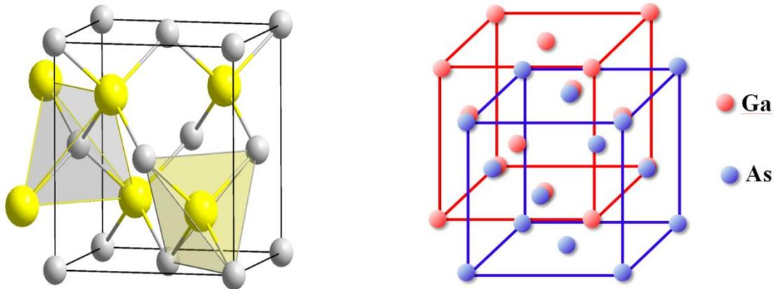
**Figure 2-6: Zinc-blende structure of gallium arsenide**
