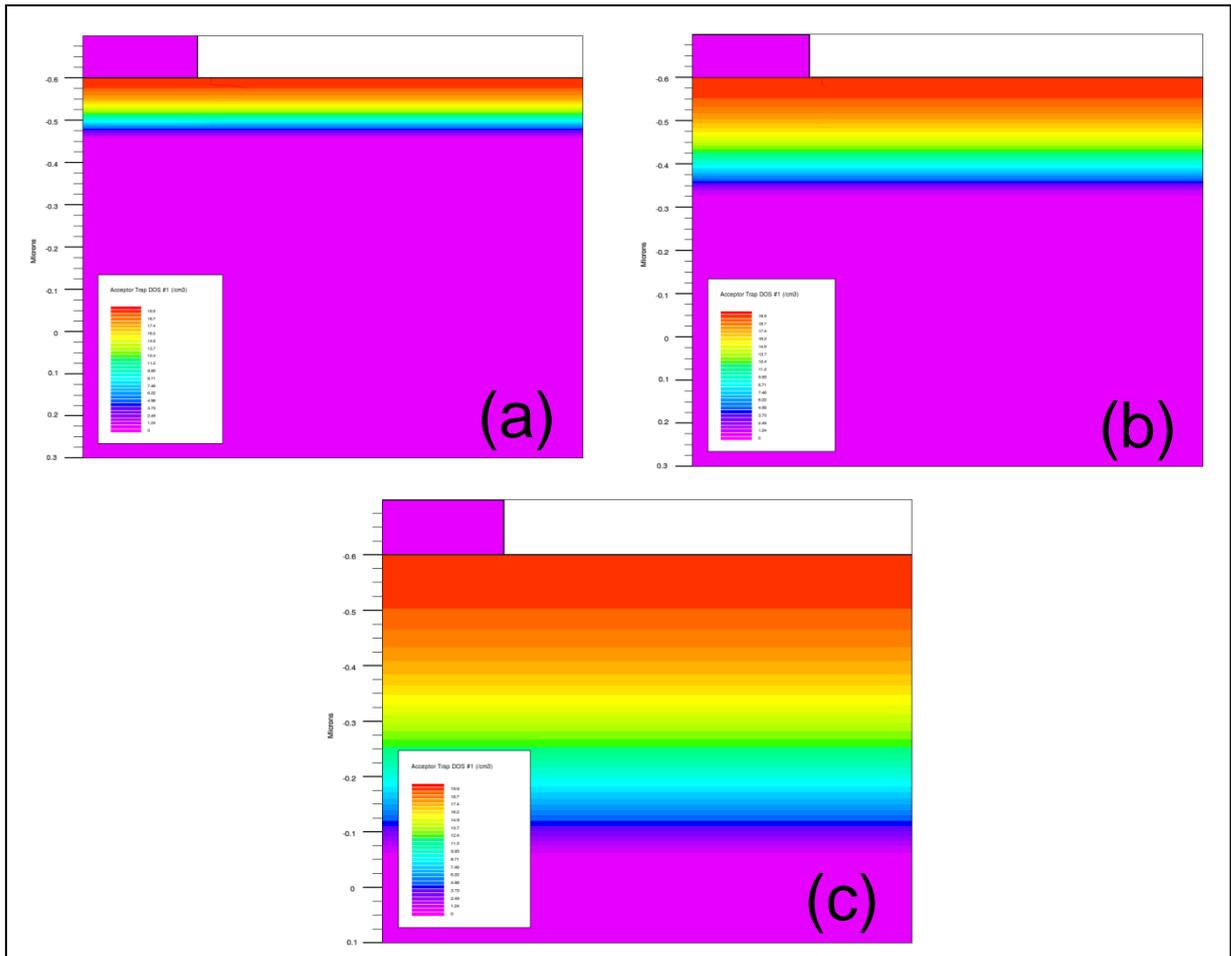
**Figure 5.33: Traps density decreasing distributions using Gaussian peak at surface with different characteristic: a. char=0.02 b. char=0.04 c. char=0.08.**
