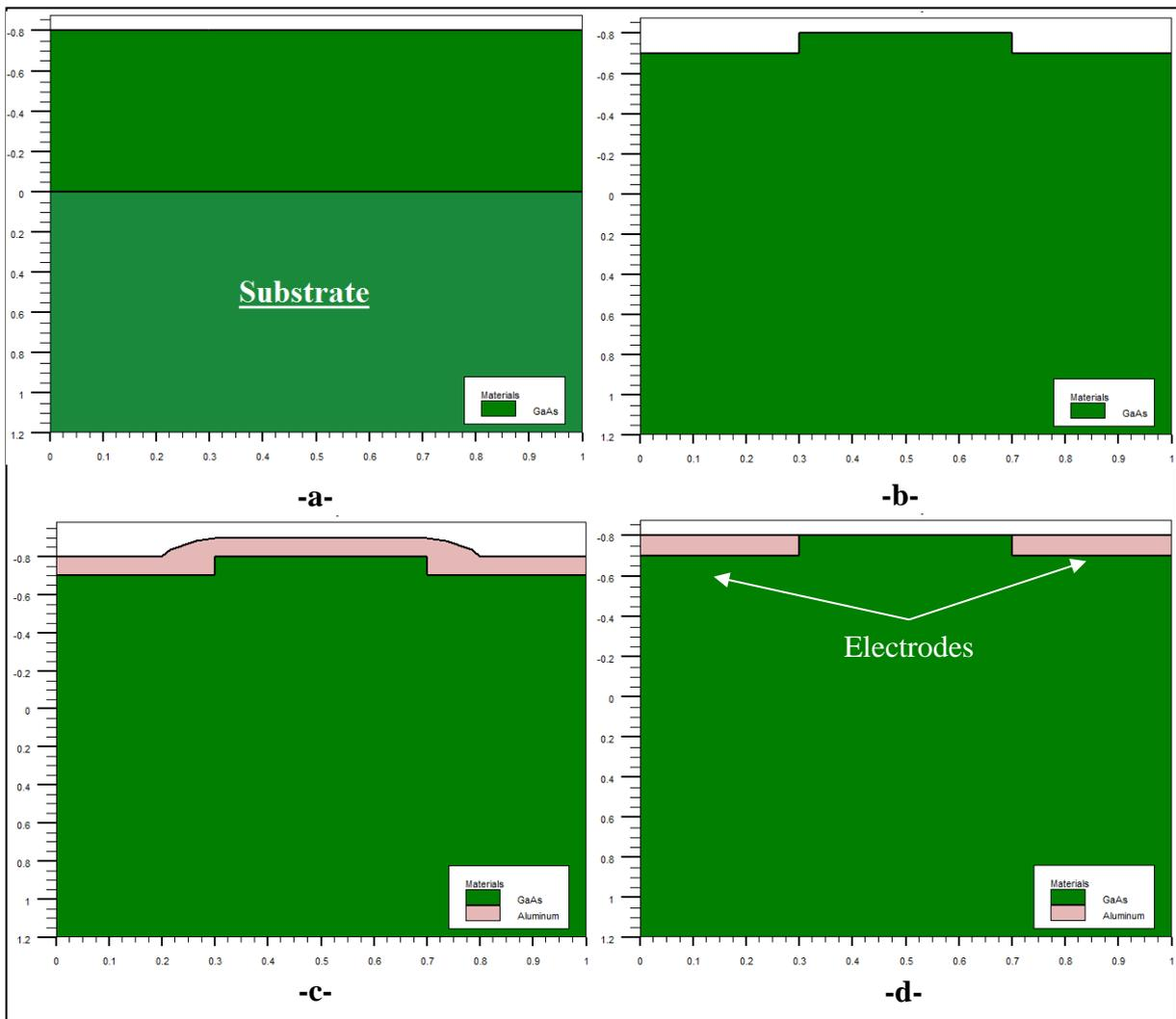
**Figure 4.4: Electrodes deposition steps: a- Primary structure. b- Prepared structure for metal deposition. c- Metal deposition. d- Final structure.**
