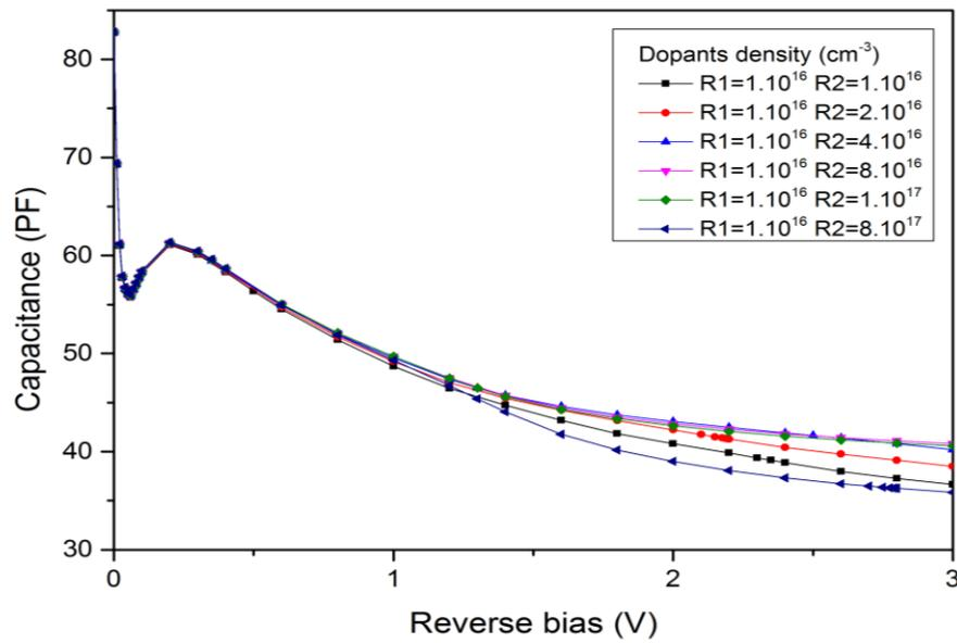
**Figure 5.29: The simulated C-V characteristics with different dopants densities in the second region (R2).**
