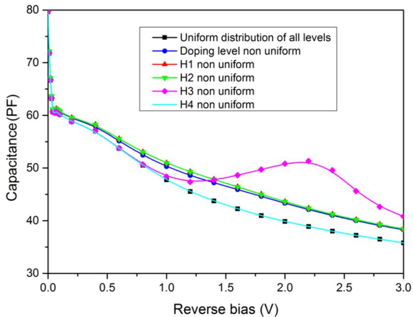
Figure 5.49: The simulated capacitance-voltage characteristics of NU926 sample: uniform distribution of all levels (squares), doping level non-uniform (circles), H1 non-uniform (up triangles), H2 non-uniform (down triangles), H3 non-uniform (diamonds) and H4 non-uniform (simple line).
