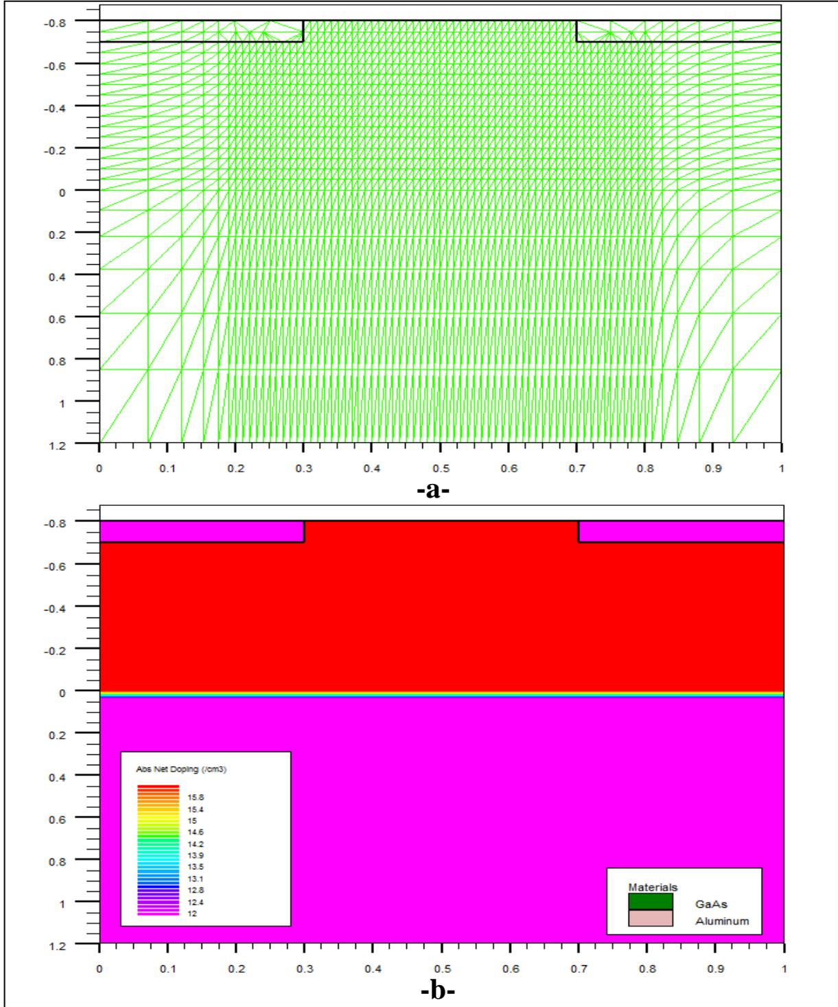
Figure 4.5: Final structure: a- Structure mesh. b- Dopants density.
