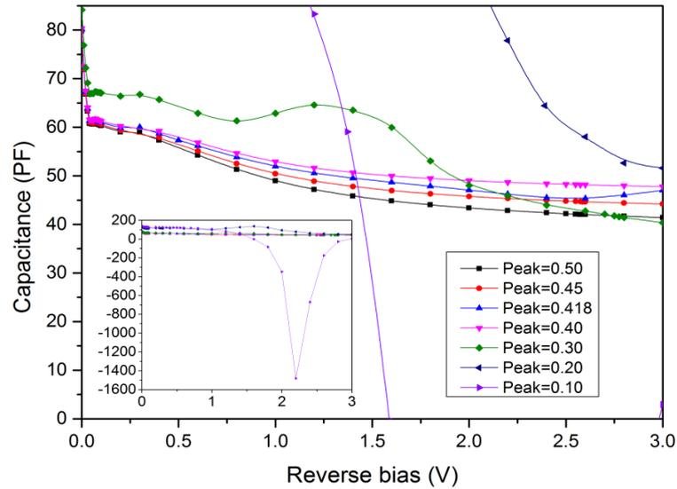
**Figure 5.37: The simulated Capacitance voltage in present of traps peak at different distances from the surface.**
