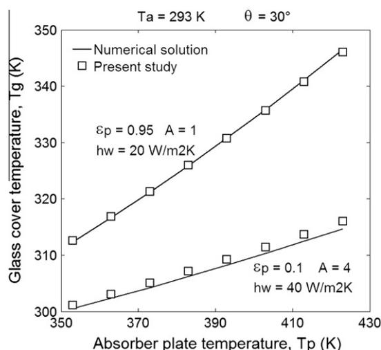
Fig. 5. Variation of the glass cover temperature with the absorber plate temperature.
