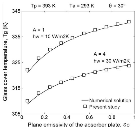
Fig. 3. Variation of the glass cover temperature with the plane emissivity of the absorber plate.
