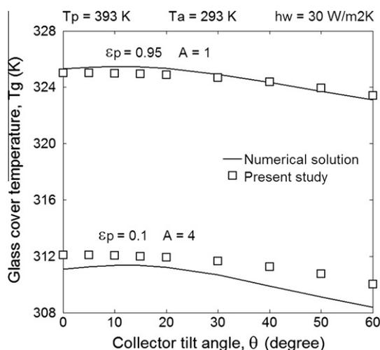
Fig. 4. Variation of the glass cover temperature with the collector tilt angle.
