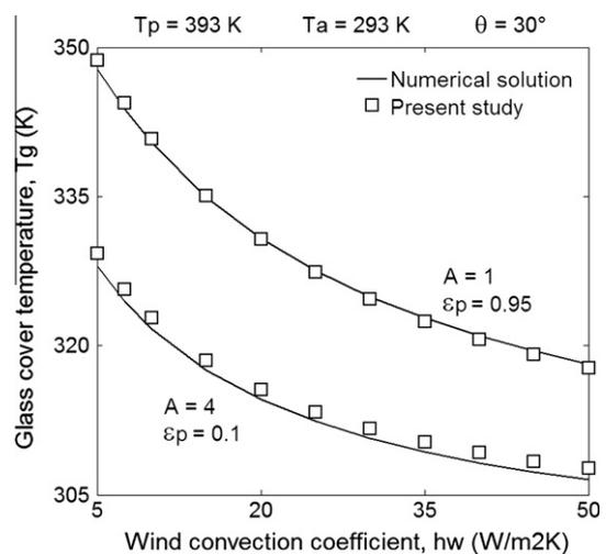
Fig. 2. Variation of the glass cover temperature with the wind convection coefficient.
