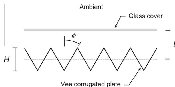
Fig. 1. Cross section of 60° vee corrugated absorber plate and flat glass cover.
