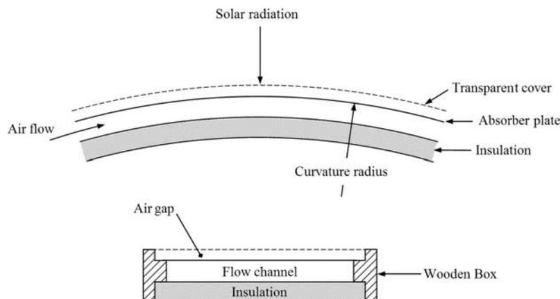
Figure 1. Side and cross section view of the curved solar air heater.
