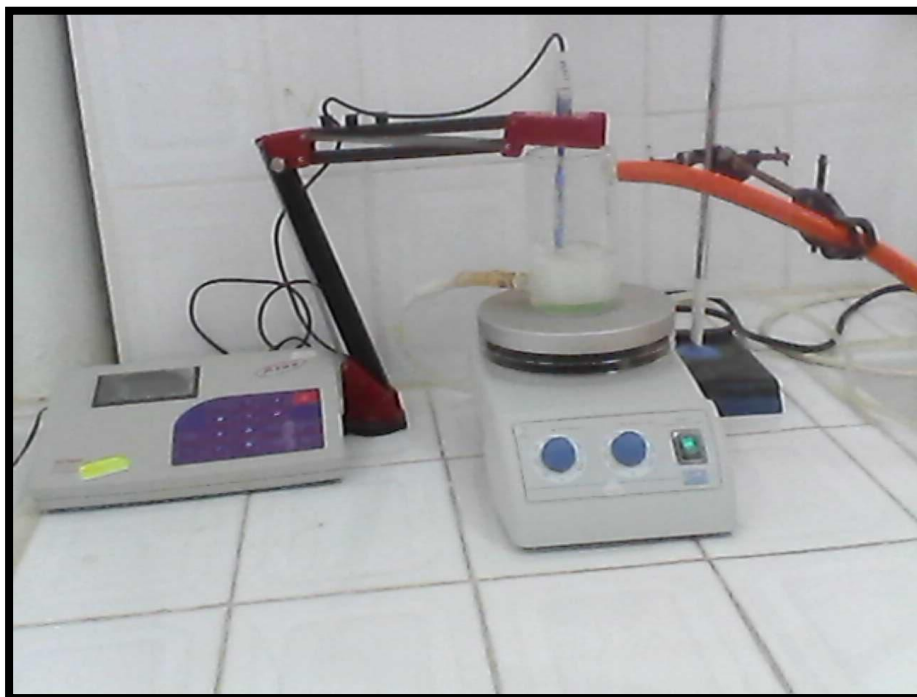
Figure II.3: Montage de l'extraction liquide-liquide
