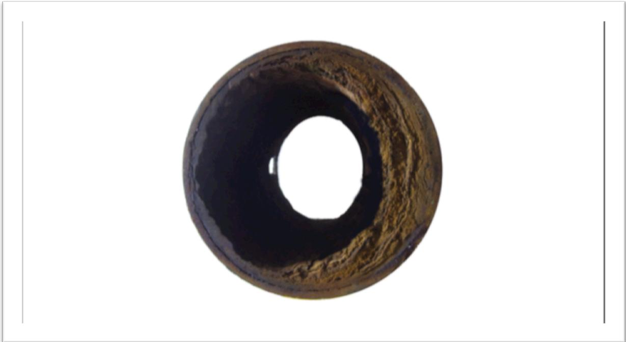
**Figure I-1: The cross section of the "scale" of a pipe**
