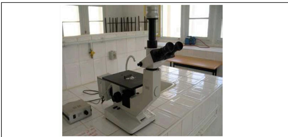
**Figure II-11 : Optical microscope HUND T100-WETZLAR**
