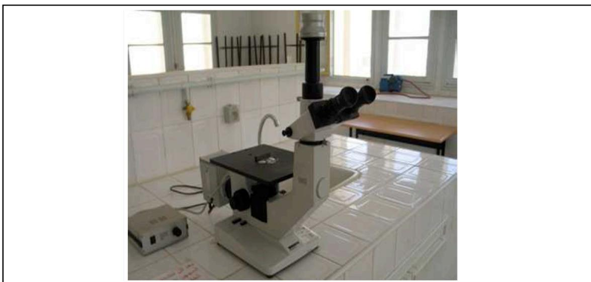
**Figure II-11 : Optical microscope HUND T100-WETZLAR**
