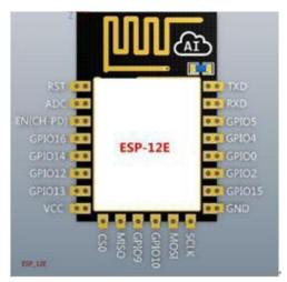
Fig.II.16 ESP-12E Pin Description
