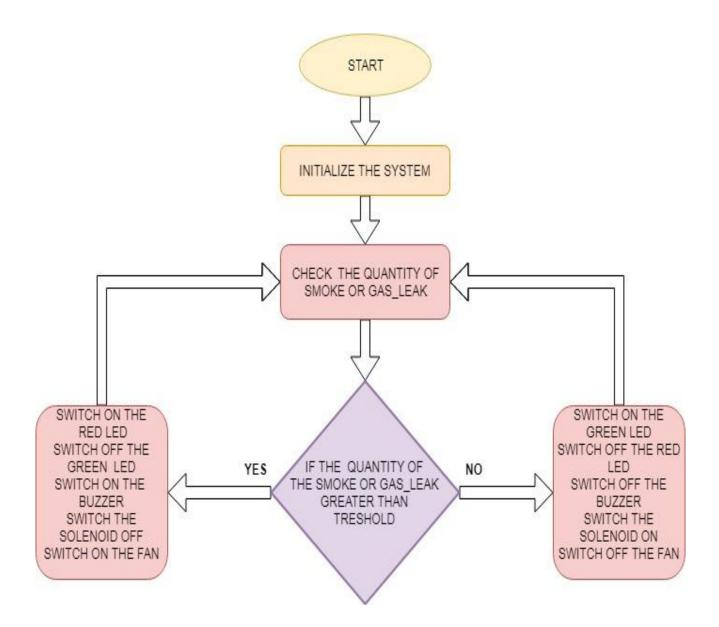
Fig.III.23 Chart Flow for gas leak & smoke
