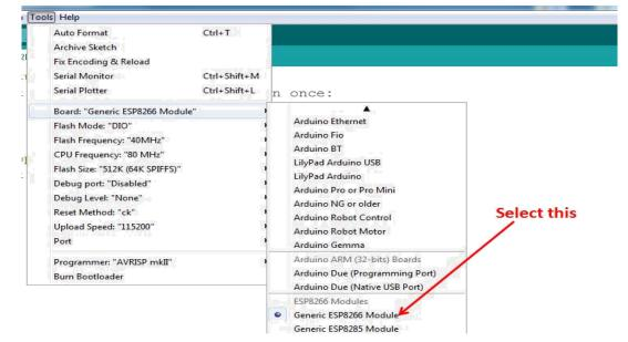
Fig.II.22 Selection of Generic ESP8266 Module
