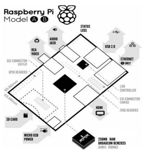
**Fig.II.1** Raspberry pi components
