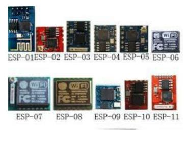
Fig.II.14 ESP8266 Boards
