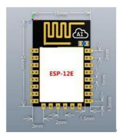
Fig.II.17 ESP-12E Packaging and Dimension
