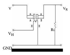
The above is basic test circuit of the sensor. The sensor need to be put 2 voltage, heater voltage (VH) and test voltage (VC) . VH used to supply certified working temperature to the sensor, while VC used to detect voltage (VRL) on load resistance (RL) whom is in series with sensor. The sensor has light polarity, Vc need DC power. VC and VH could use same power circuit with precondition to assure performance of sensor. In order to make the sensor with better
