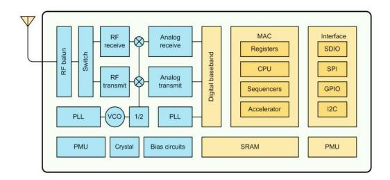
Fig.II.15 ESP8266EX Block Diagram
