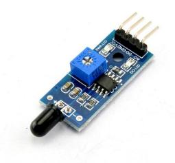
Fig.III.4 Flame Sensor
