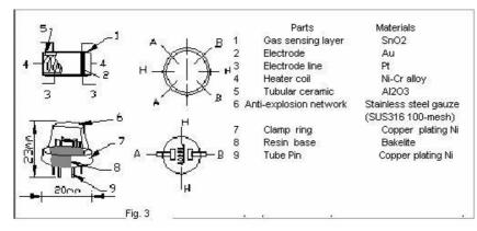
Structure and configuration of MQ-2 gas sensor is shown as Fig. 3, sensor composed by micro AL2O3 ceramic tube, Tin Dioxide (SnO2) sensitive layer, measuring electrode and heater are fixed into a crust made by plastic and stainless steel net. The heater provides necessary work conditions for work of sensitive components. The enveloped MQ-2 have 6 pin, 4 of them are used to fetch signals, and other 2 are used for providing heating current.
