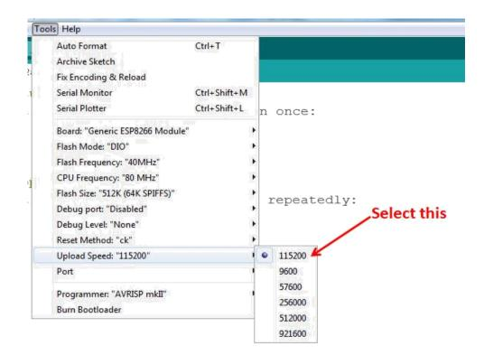
Fig.II.23 Selection of baud rate 115200
