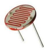
Fig.III.5 Light Dependent Resistor LDR
