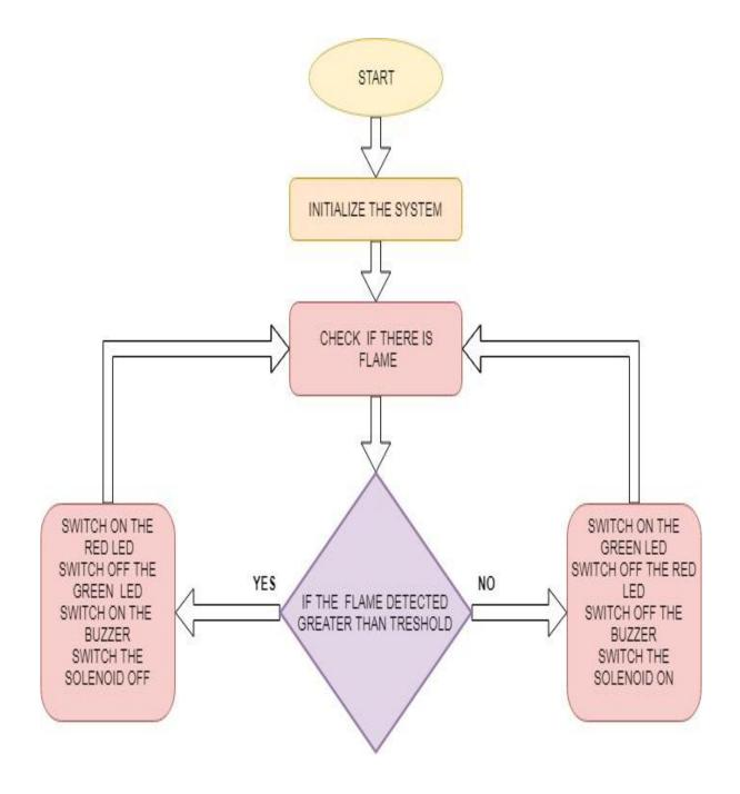
Fig.III.24 Chart Flow for Detecting a Flame
