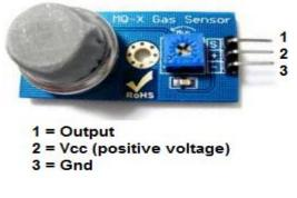
Fig.III.2 MQ2 Smoke Sensor
