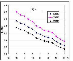
Fig.2 shows the typical temperature and humidity characteristics. Ordinate means resistance ratio of the sensor (Rs/Ro), Rs means resistance of sensor in 1000ppm Propane under different tem. and humidity.
