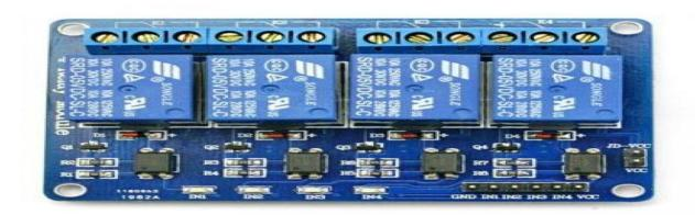
Fig.III.6 Four Channel Relayboard
