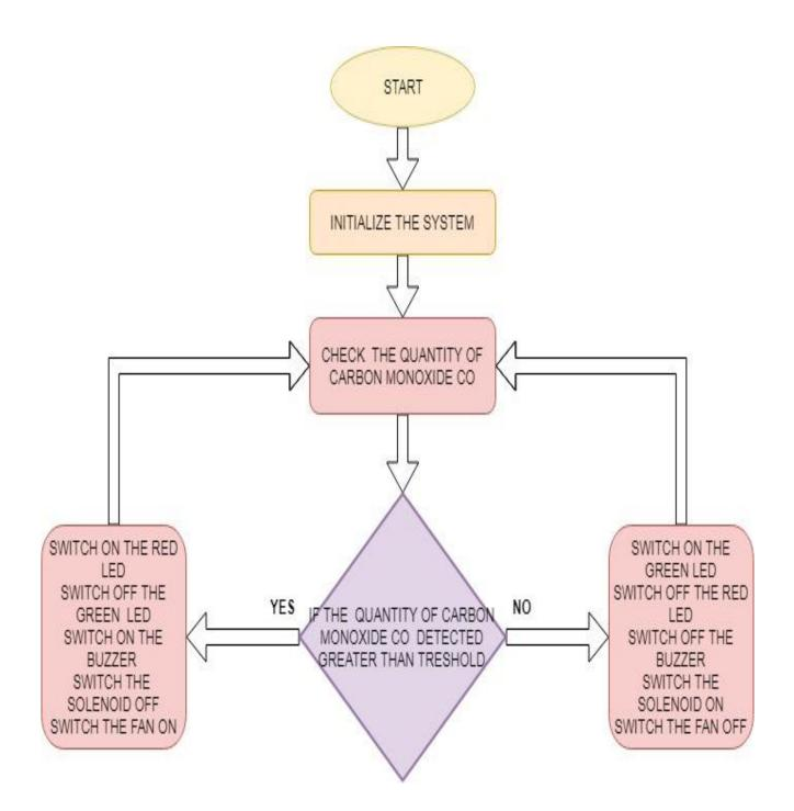
Fig.III.25 Chart Flow for Detecting Carbon Monoxide CO
