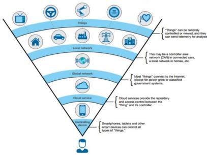
Fig.I.1 Automation System Using (IoT)
