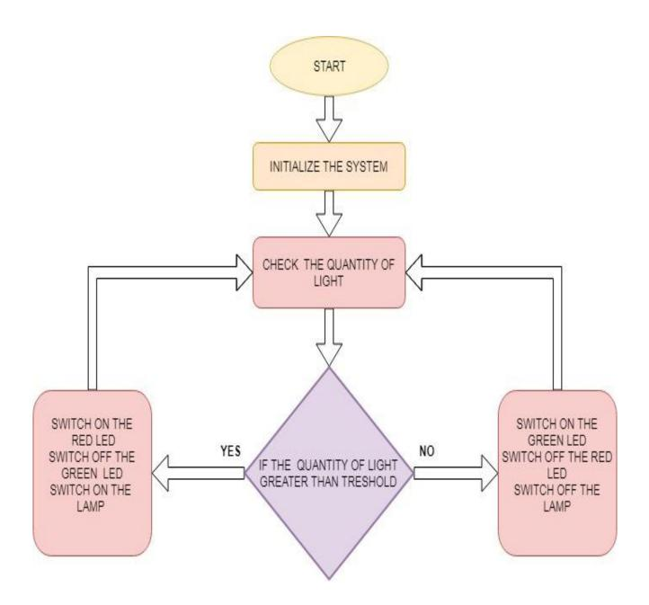
Fig.III.26 Chart Flow for Detecting Light
