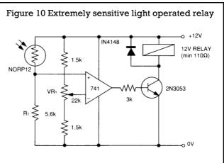
(Relay energised when light exceeds preset level.) Incorporates a balancing bridge and op-amp.  $R_1$  and NORP12 may be interchanged for the reverse function.
