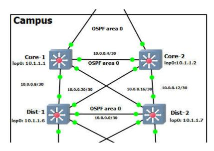
Figure 3.3 : Distribution and Core Layers of Enterprise Campus Network.
