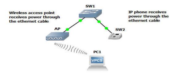
Figure 1.11 : Power over Ethernet.
