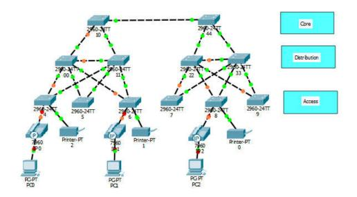
Figure 1.2 : The Hierarchical Network Model.
