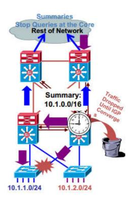
Figure 2.17 : Summary at the Distribution Layer Reduces Routing Traffic. [11]
