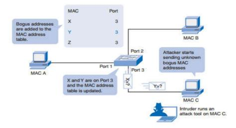
Figure 2.21 : Host C Sends Frames with Bogus Sources.
