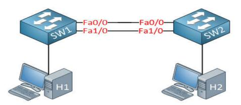
Figure 2.8 : redundancy between two switches. [8]
