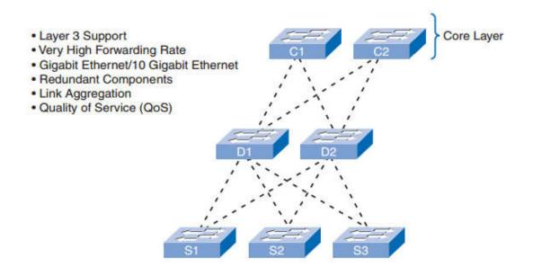
Figure 1.14 : Core Layer Switch Features.
