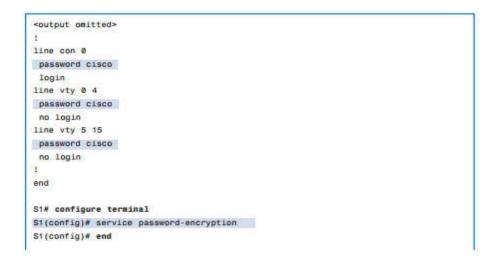
Figure 2.18 : Clear-text Passwords in the running-config File.
