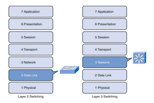
Figure 2.12 : Layer 2 and Layer 3 Switching. [3]
