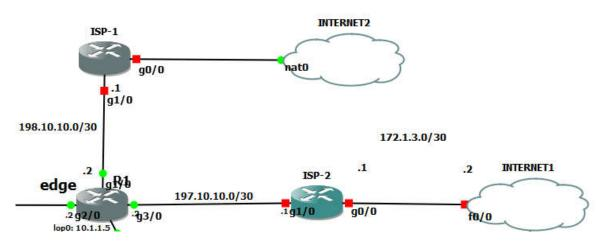
Figure 3.7 : Company Connection to the Internet via edge router.
