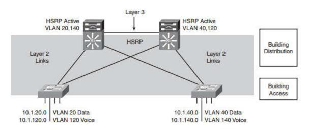
Figure 2.15 : Layer 3 Distribution Switch Interconnection. [12]
