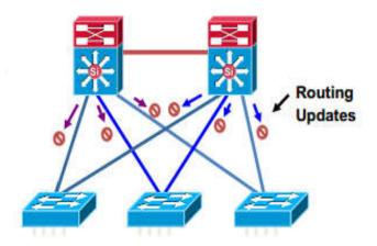
Figure 2.16 : Limit Unnecessary Peering Across the Access Layer. [11]
