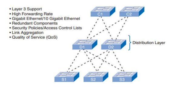
Figure 1.13 : Distribution Layer Switch Features.
