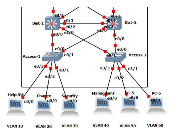
Figure 3.2 : Access Switches Connected to Distribution Layer.
