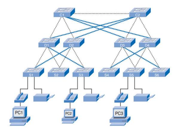
Figure 1.7 : Redundancy. [3]
