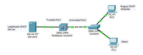
Figure 2.22 : DHCP Snooping to Prevent DHCP Attacks.
