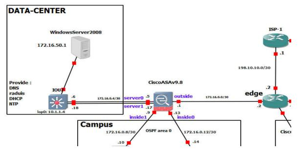
Figure 3.4 : CiscoASAv9.8, Campus, DATA-CENTRE and edge Connection.
