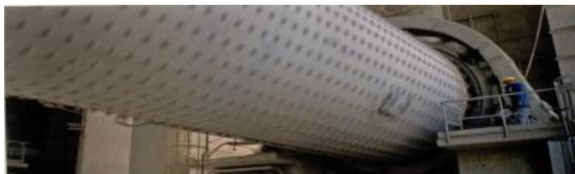
Figure I.7 : Broyeur de ciment [1]
