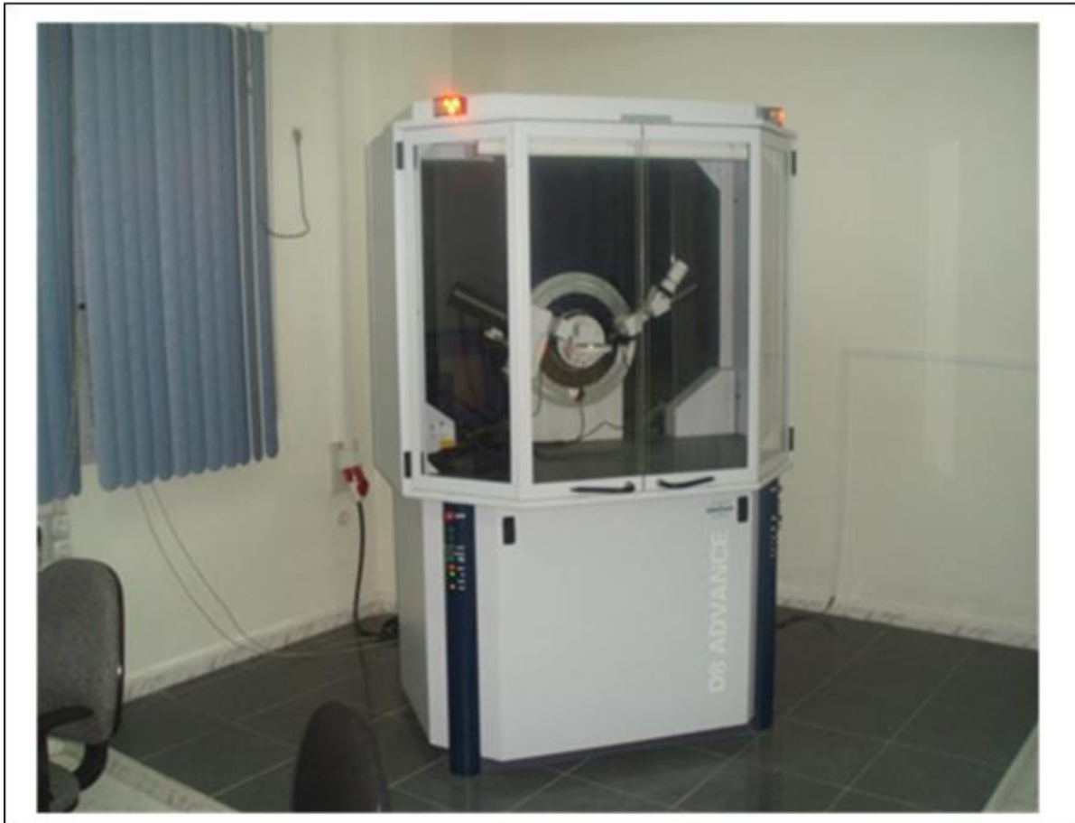
Figure.III.8. Diffractomètre Panalytical X'Pert (D8 ADVENCE) BRUKER.
