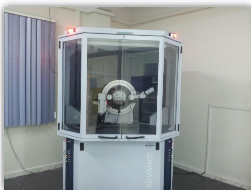
Figure (II-20) : Diffractomètre BRUKER-AXS type ADVANCE D8.
